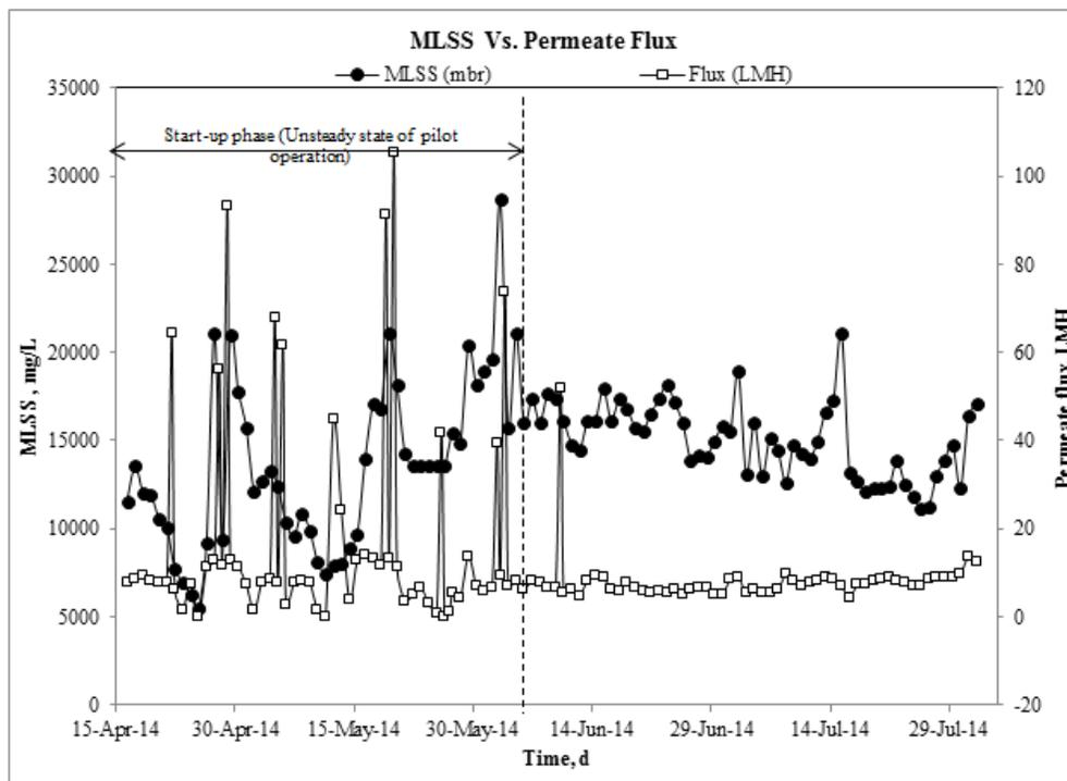
Figure 19: MLSS concentration vs. permeate flux
