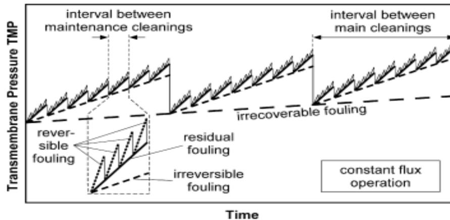
**Figure 14:** Various fouling rates under long term operation of full-scale MBRs (Drews, 2010)
