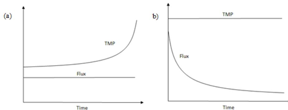
**Figure 12:** (a) Constant flux mode (b) Constant TMP mode
