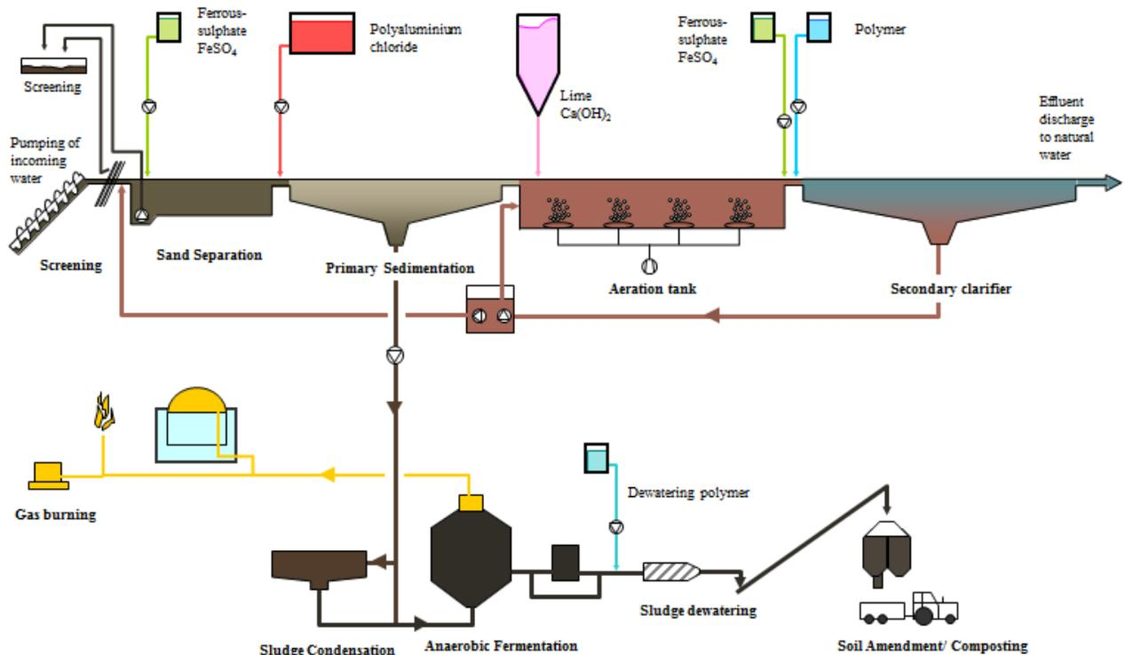
**Figure 4:** Conventional Activated Sludge Process at Kenkäveronniemi WWTP, Mikkeli, Finland
