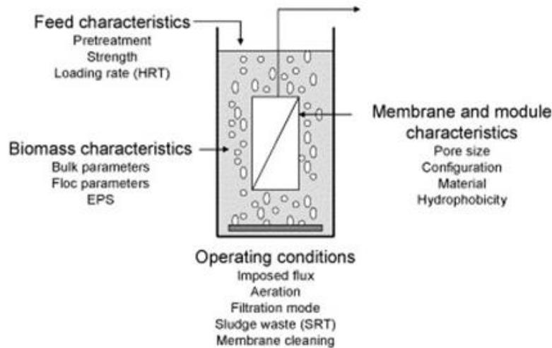
**Figure 15:** Interrelationships of parameters affecting membrane fouling (Le-Clech et al., 2006)
