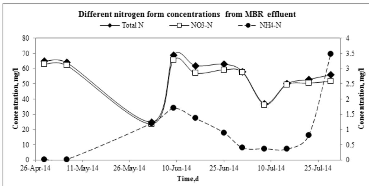
Figure 31: Concentration of different nitrogen from MBR effluent
