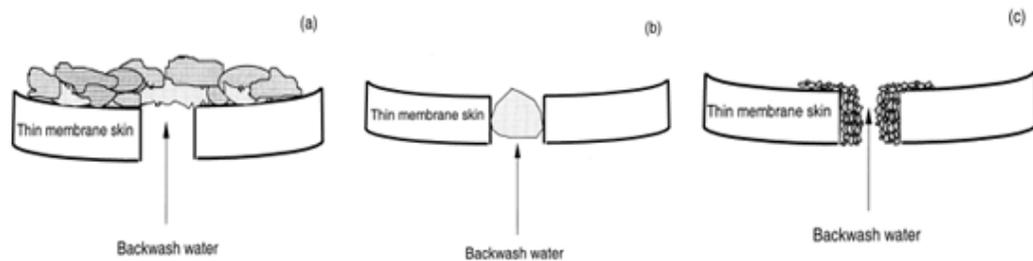
**Figure 13:** Membrane fouling mechanisms: (a) Gel/ cake formation (b) Pore plugging (c) Pore narrowing (Bourgeois et al., 2001)
