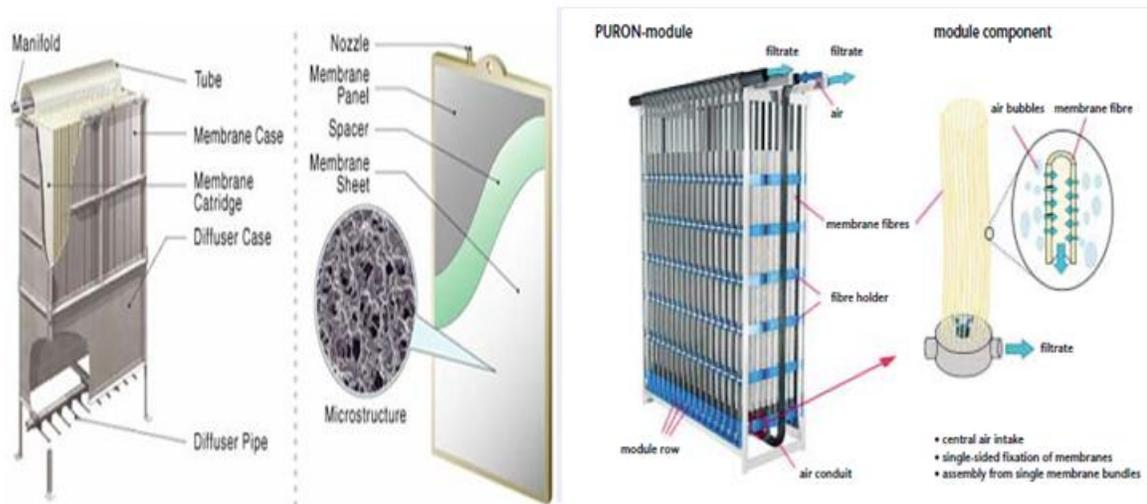
**Figure 9:** Flat-sheet & Tubular membrane modules
