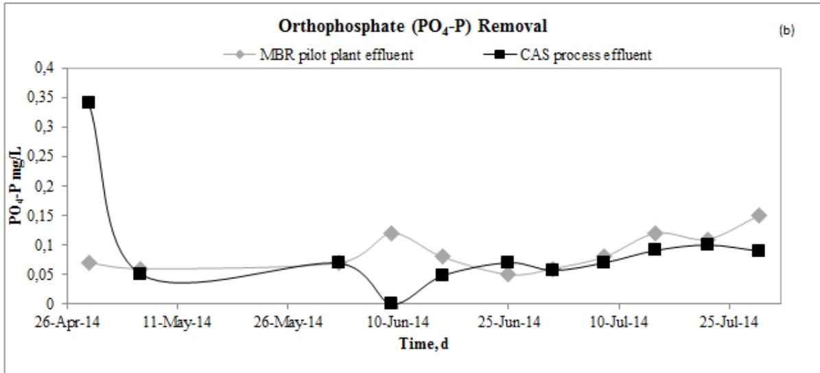
Figure 29: (a) Total phosphorus, (b) PO<sub>4</sub>-P removal
