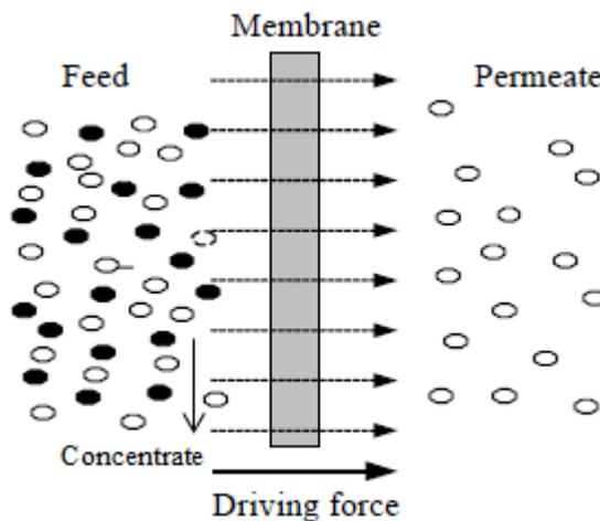
**Figure 7:** Membrane filtration principle (Abeyanyaka, 2009)
