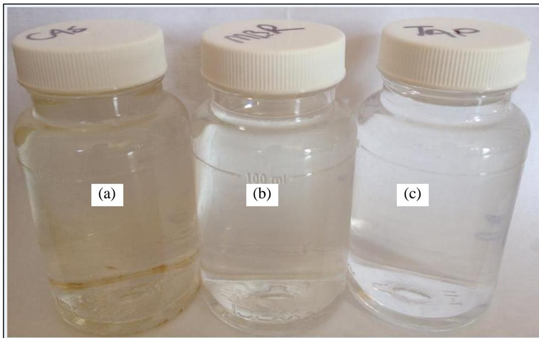
Figure: (a) CAS process effluent (b) MBR pilot plant effluent (c) Tap water
