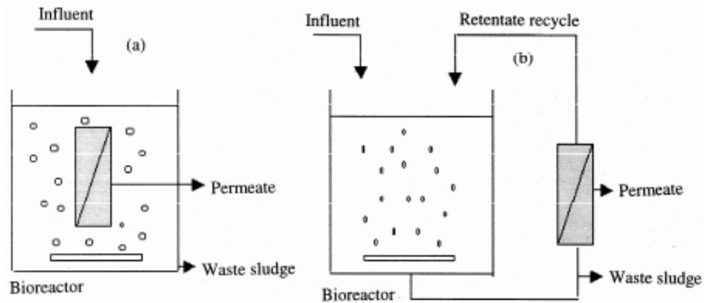
**Figure 11:** MBR arrangements (a) Submerged/immersed, (b) Side-stream/ external (Gupta et al., 2006)
