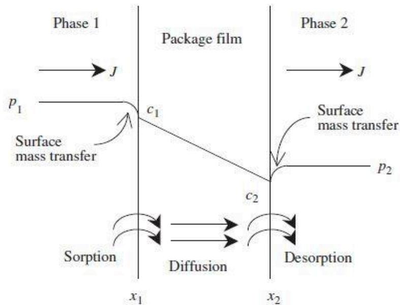
**Figure 6.** Gas permeation through packaging material, where  $p$ =pressure,  $c$ = permeant concentration (Siracusa, 2012).
