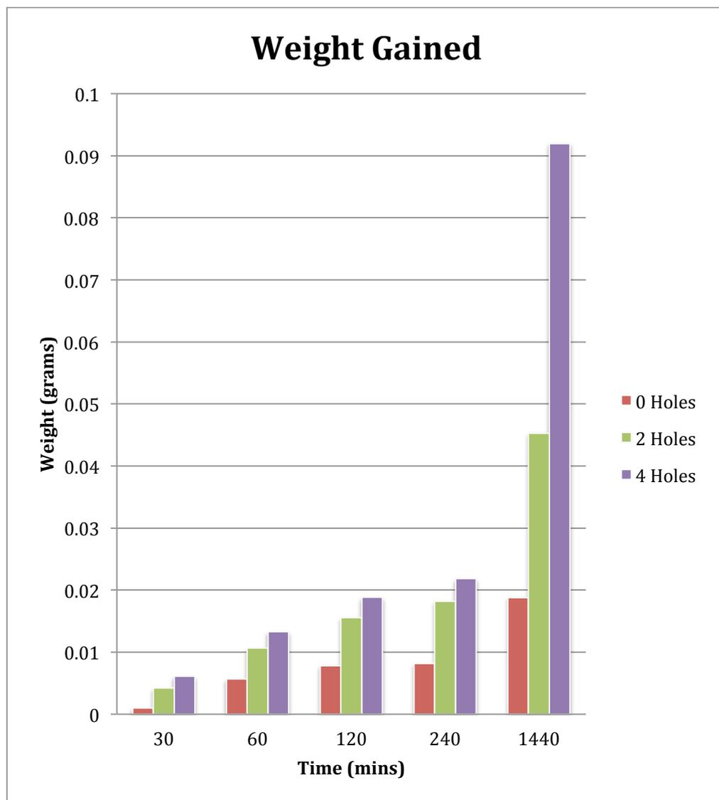
Figure 34. Average weight gained of moisture for Condition A.
