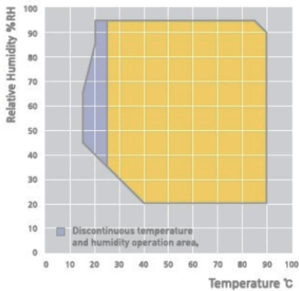
**Figure 26.** Temperature & Humidity Control Range (Jeitech, 2015).
