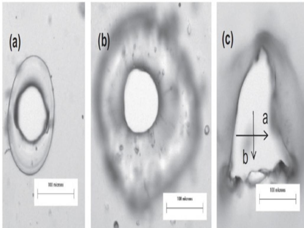
**Figure 12.** Comparative images for: (a) Microperf-BOPP, (b) Microperf-PET and (c) Mechperf-PET. a and b give the various diameters in x-y-direction. (Larsen & Liland, 2013, p. 275.)
