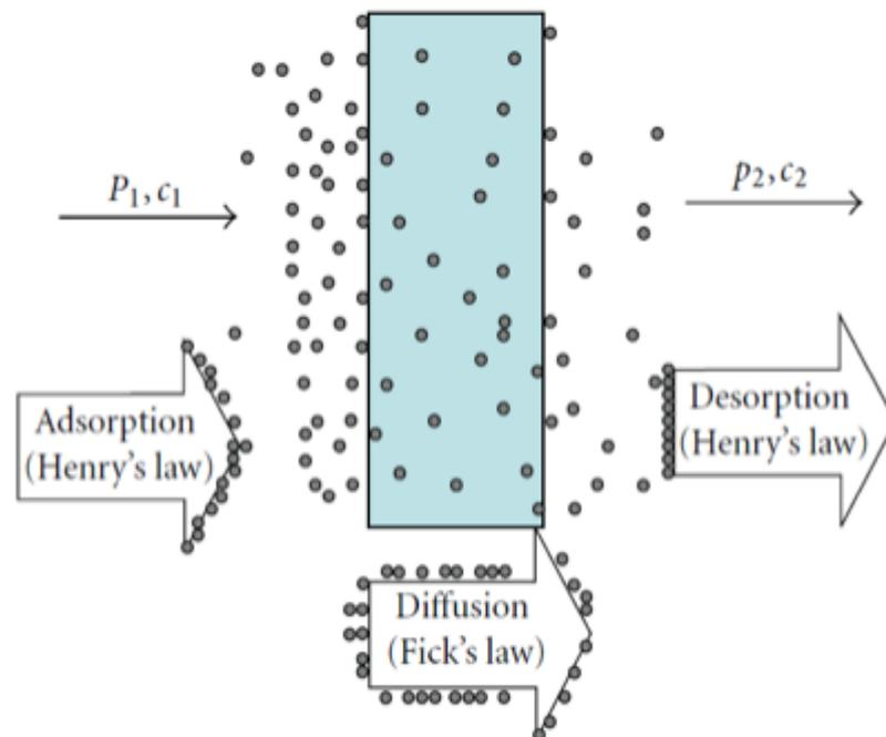
**Figure 5.** Penetration mechanism over polymeric film seal (Siracusa, 2012, p. 2).
