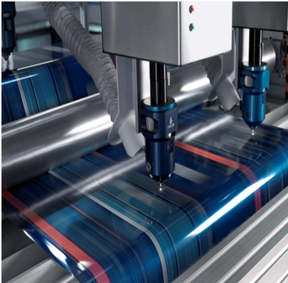
**Figure 8.** Laser perforation process on a printed web (Packaging-Labeling, 2015).
