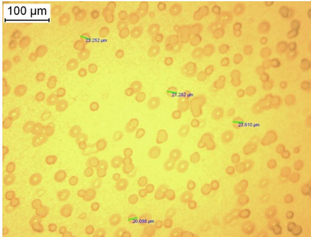
**Figure 19.** Microscopic view of 20  $\mu\text{m}$  diameter holes of a polycarbonate membrane.
