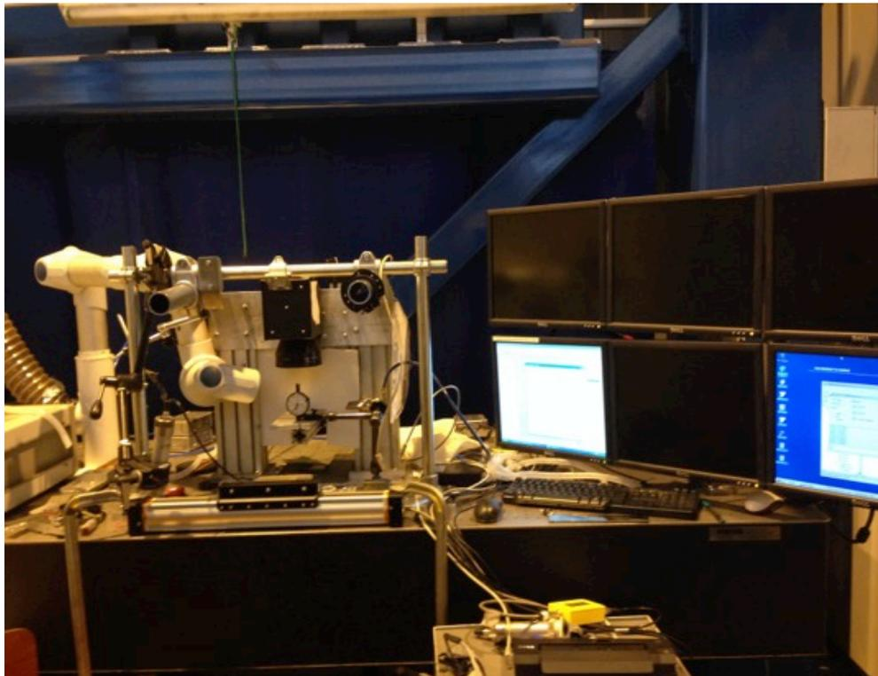
**Figure 18.** LUT future factory's fiber laser assembly used in perforation.
