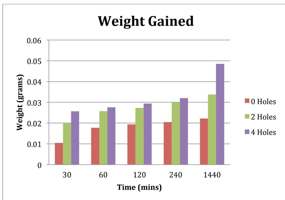
**Figure 36.** Average weight gained of moisture by flask assemblies within 24 hours of Condition B (Fridge Condition).
