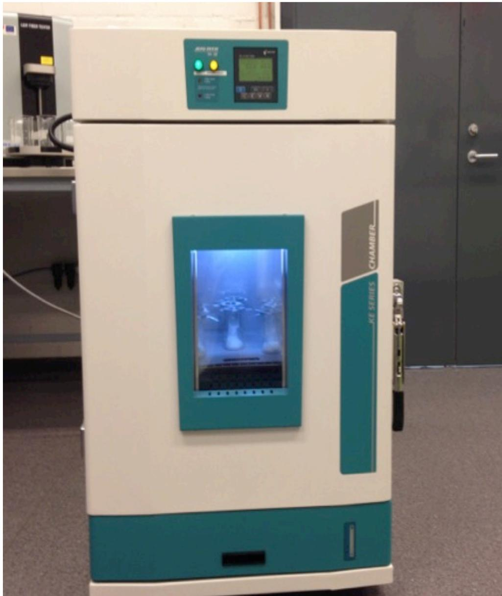
**Figure 25.** Jeiotech temperature and humidity chamber.
