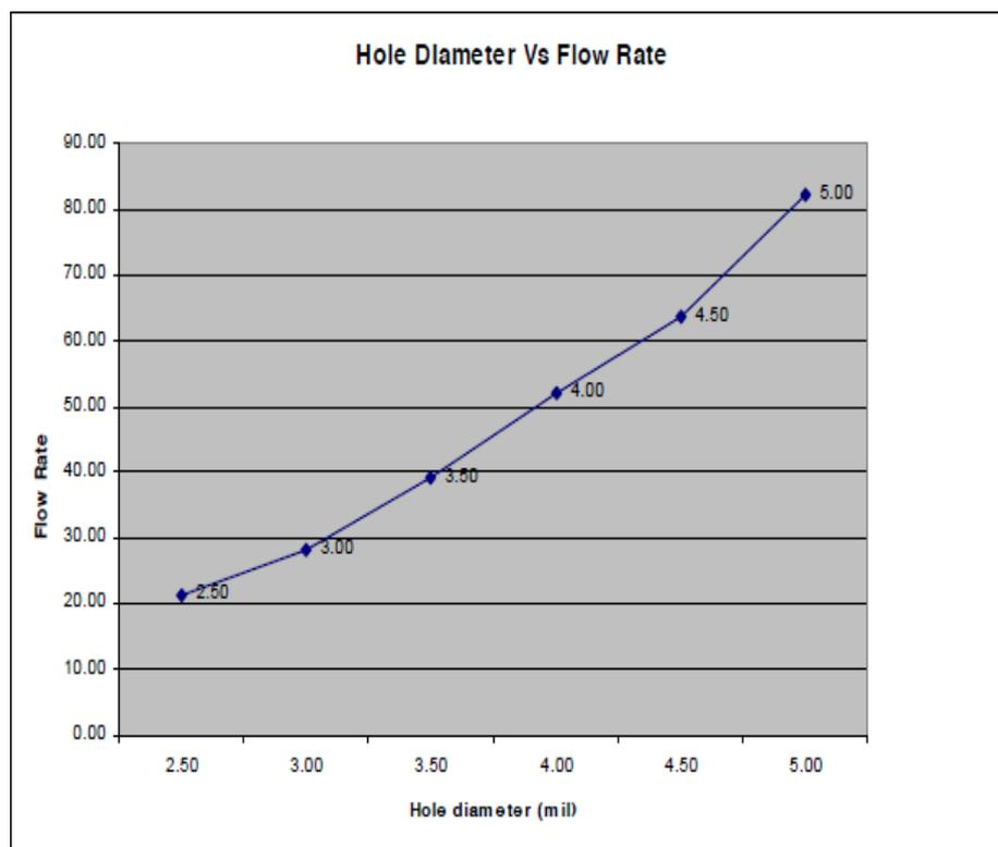
**Figure 11.** Flow rate ( $\text{g}/\text{m}^2/\text{h}$ ) with respect to hole diameter for a film laminate (Christopher, 2002 p. 4).
