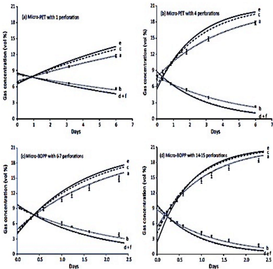
**Figure 13.** Observable change in the amount of gases with respect to the holes used in period of storage. (Fishman, Rodov, & Ben-Yehoshua, 1996.)
