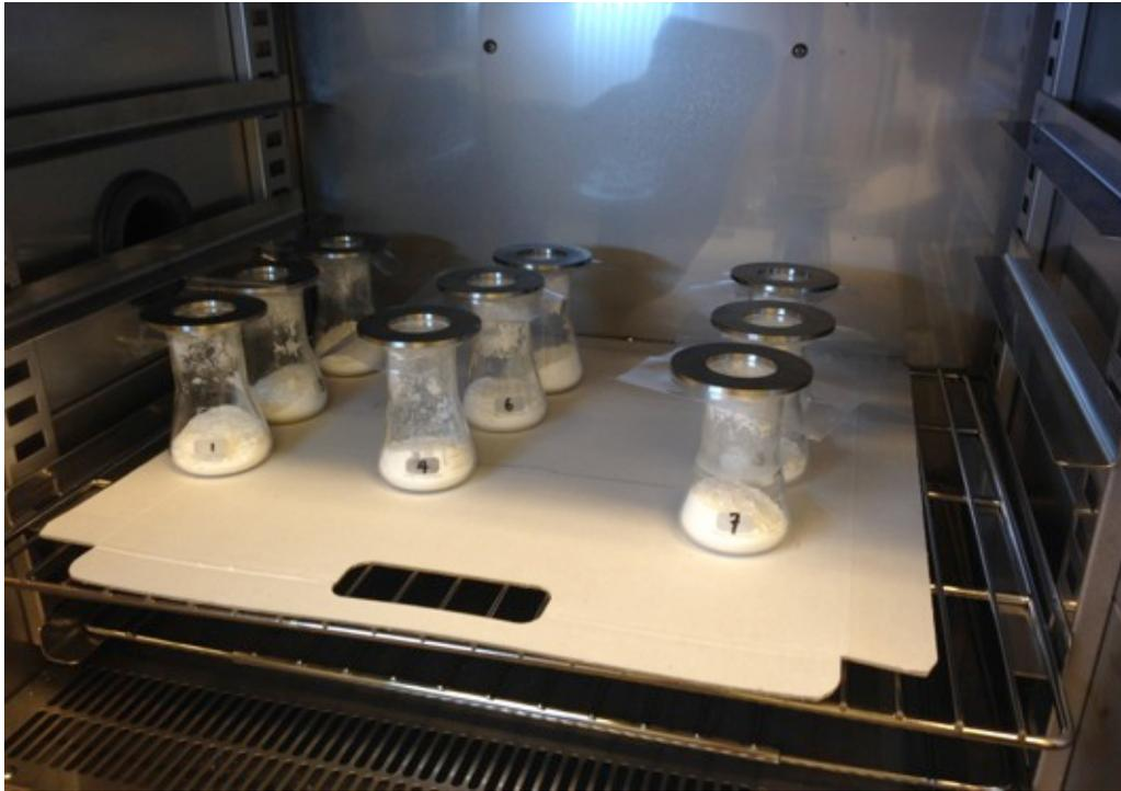
**Figure 28:** Marked assemblies inside of the temperature and humidifying chamber.
