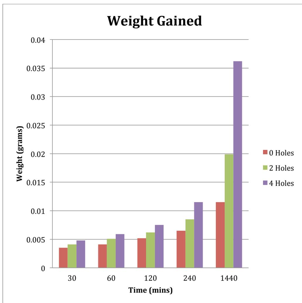
**Figure 38.** Average weight gained of moisture by flask assemblies within 24 hours of Condition C (Tropical condition).
