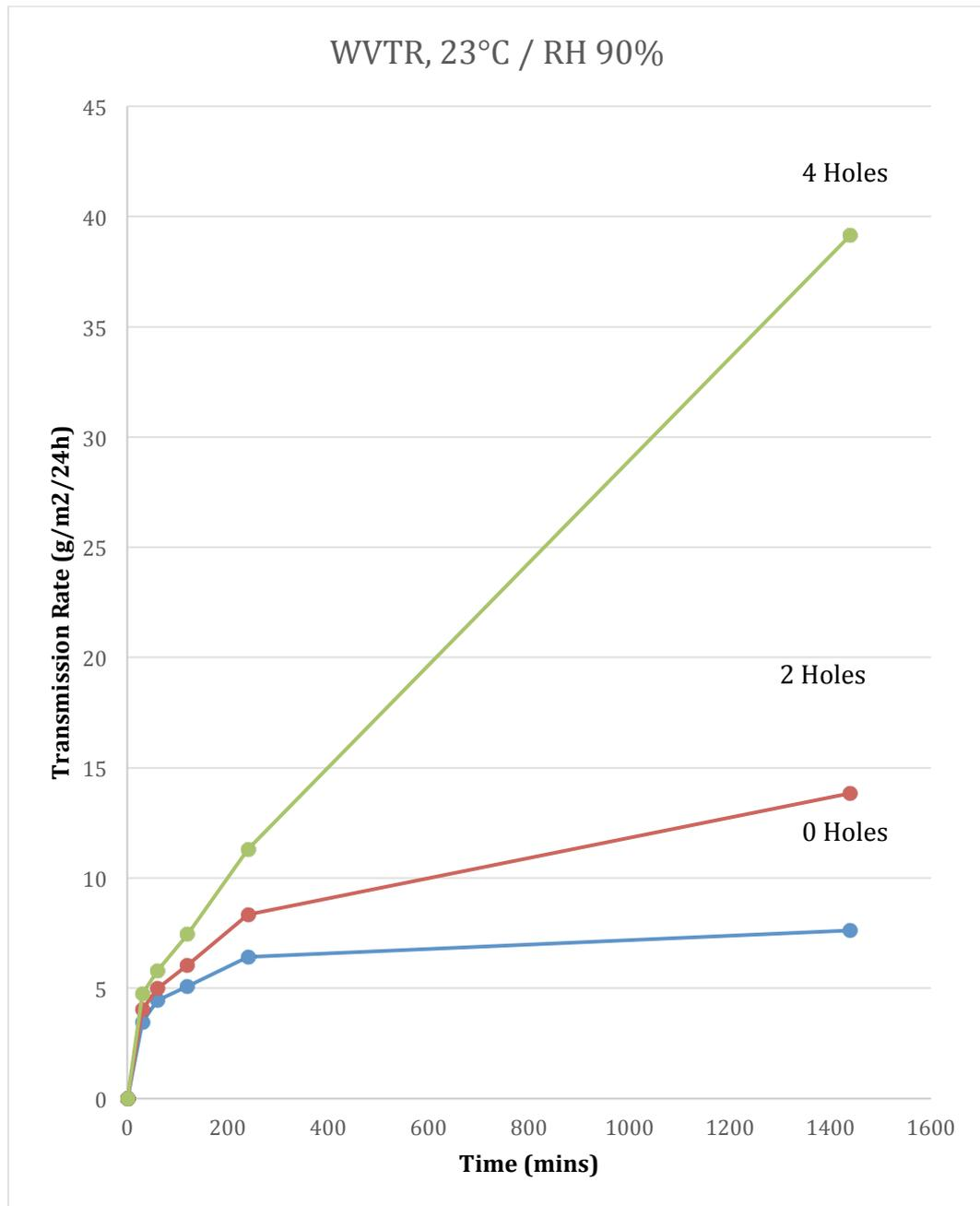
**Figure 39.** WVTR measurement with various test pieces with 24 hours at Condition C (Tropical Condition).
