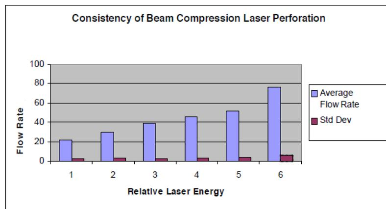
**Figure 10.** Flow rate (g/m<sup>2</sup>/h) with respect to the relative laser energy (Joules) for the Beam Compression Laser (Christopher, 2002).
