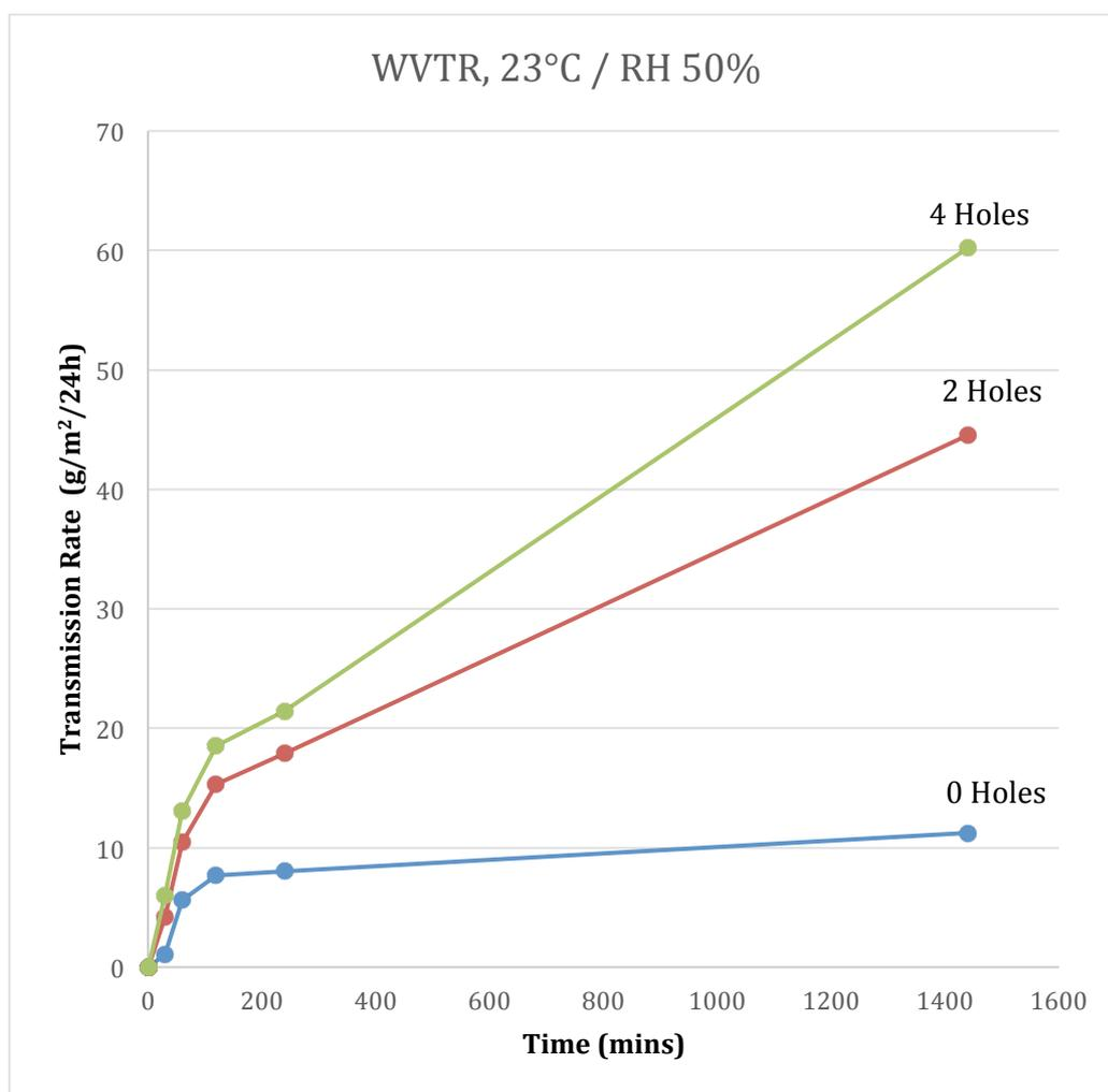
Figure 35. WVTR measurement with various test pieces with 24 hours at Condition A (Standard Condition).
