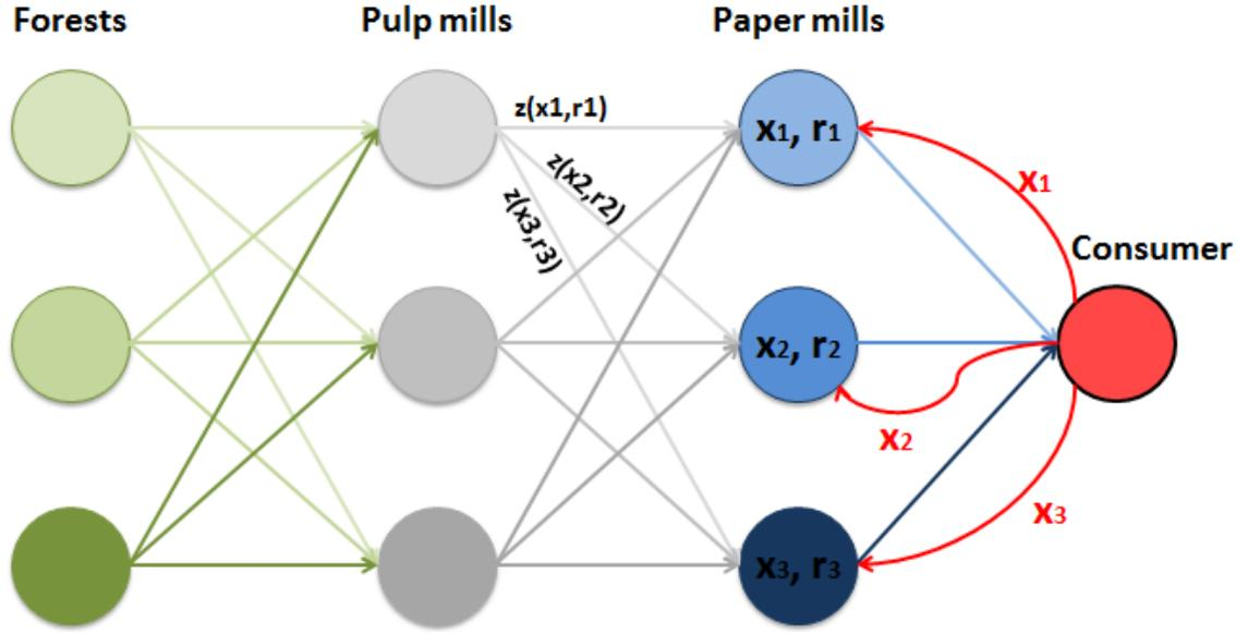
Figure 15: Model of the supply chain for manufacturing one tonne of paper and shipping it to a consumer. Red arrows represent transportation of waste paper from consumer to paper mills for recycling. Values  $x_i$  is the amount of waste paper, which should be shipped to a corresponding mill.  $z(x_i, r_i)$  is virgin pulp requirements, which should be shipped to a corresponding paper mill from any pulp mill.
