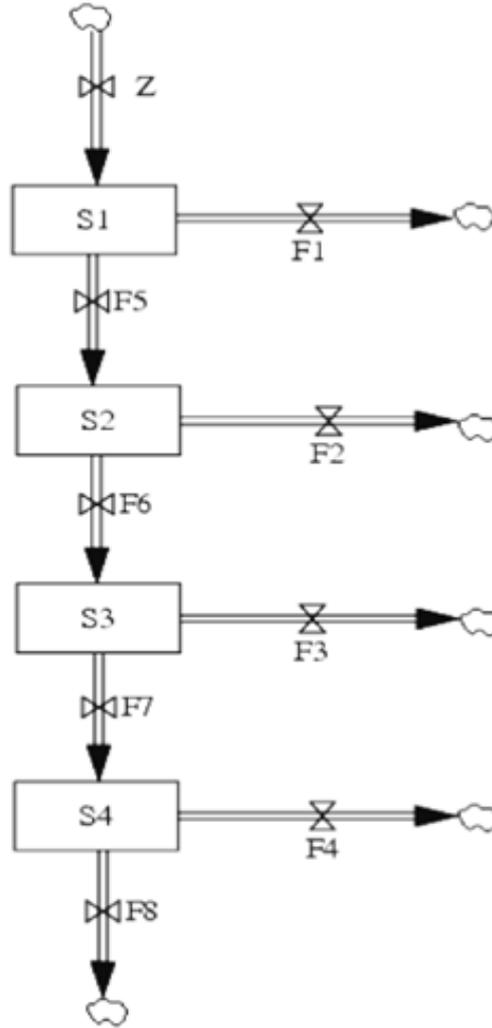
Figure 2: Closed-system fibre recycling model. Stocks S1 - S4 represent fibre stocks of different qualities in the system. Flows F1 - F4 represent nonrecycled fibre flows exiting the system. Flows F5 - F8 represent damaged fibre flows. Flow Z represents the new fibre requirement for the system.[14]
