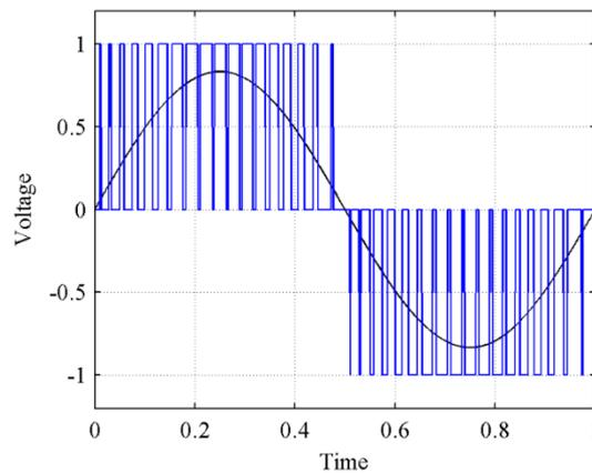
Figure 1.2. An example of a PWM-waveform. Stepped line is the actual voltage curve and sinusoidal line is the fundamental waveform.
