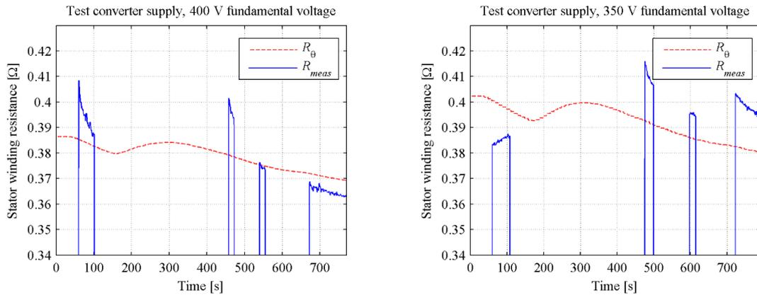
Figure 4.4 Stator winding resistance curves during the measurements on test converter supply of 400 V and 350 V. The resistance  $R_{meas}$  is determined from the 4-wire measurement between the tests. The resistance  $R_{\theta}$  is calculated from the stator winding temperature. The plots show that the 4-wire resistance measurement gives inconsistent results.
