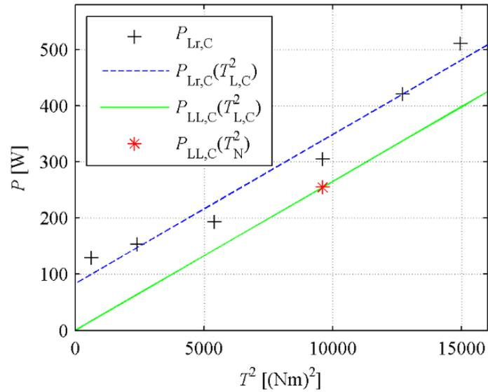
Figure 4.1. Determining the stray-load losses with the residual loss method on the 350 V, 50 Hz test converter supply. The dashed line is the smoothed linear relationship of the residual loss points. However, the loss points seem to form more like an exponential curve.
