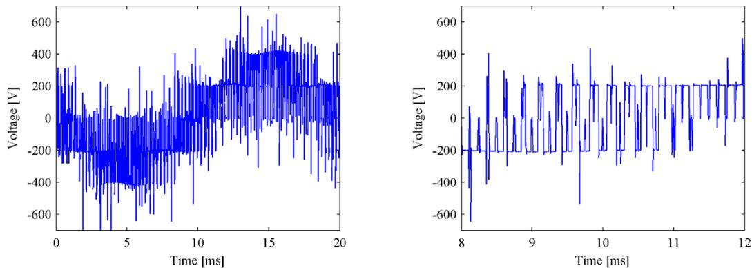
Figure 1.3. An example of an actual output voltage waveform of a commercial two level frequency converter. The fundamental frequency is 50 Hz and carrier frequency 4 kHz. Left plot shows the waveform during a complete fundamental frequency period of 20 ms. The right plot gives a closer view between 8 ms and 12 ms marks of the first plot, making the squared waveform more easily seen.
