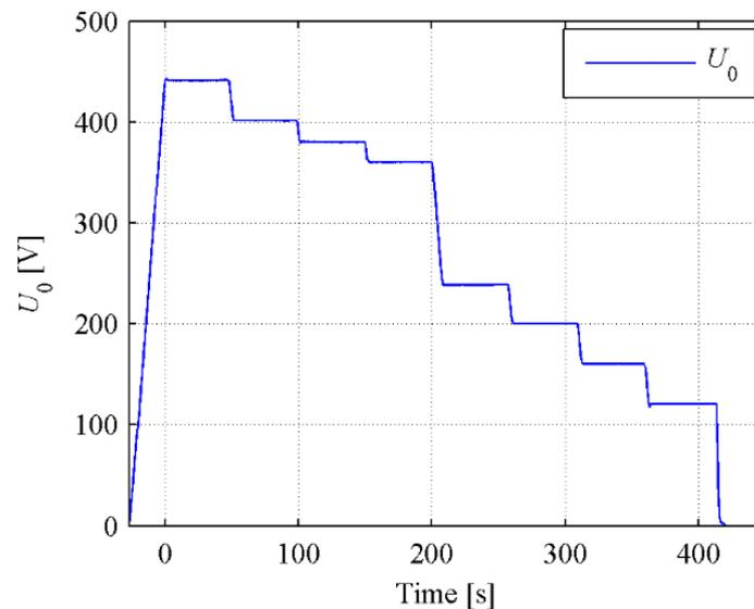
Figure 3.6. The measured voltage curve during no-load test. Voltage points between 110 % and 30 % of rated voltage were applied in descending order and each point was run for approximately 45 seconds. The delay of adjusting the voltage between the measurement points causes the total duration of all eight points to exceed 400 seconds.
