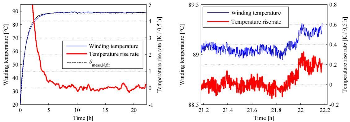
Figure 3.3. Temperature measurements and rise rates during the heat run of the rated voltage test run. Left plot shows the whole 22-hour heat run and the right plot is a more detailed view of the last 60 minutes. The dashed line in left plot depicts the stator winding temperature  $\theta_{\text{meas,N,fit}}$  calculated from the thermal time constant  $\tau$  determined for the motor. Calculations and determination of  $\tau$  are presented in Appendix 2.
