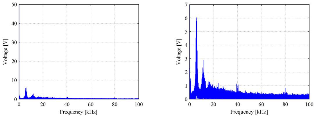
Figure 1.5. An example of harmonic content of a DTC modulated voltage waveform with fundamental frequency of 50Hz. The left plot shows the harmonics in similar scale as the SVM harmonics in Figure 1.4. The right plot has smaller voltage scale to bring the high frequency harmonics more visible.
