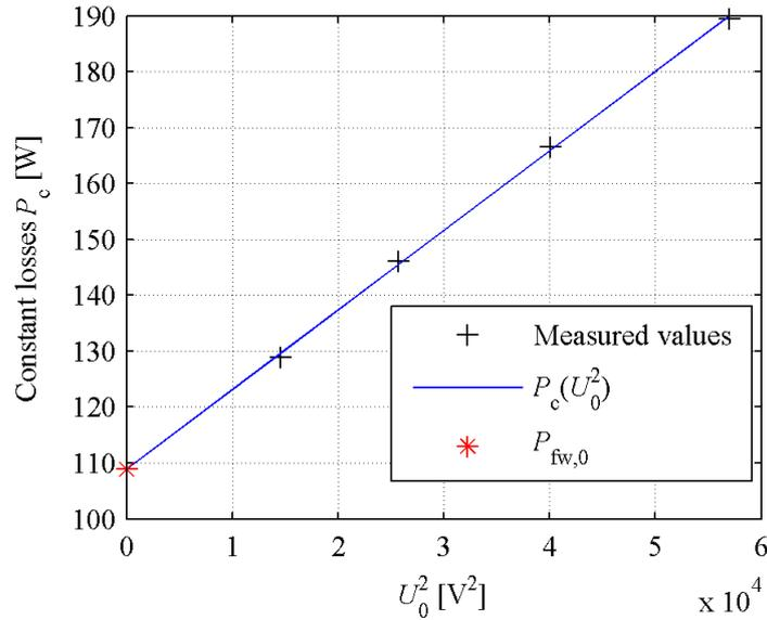
Figure 3.7. The principle of determining friction and windage losses. Four points marked with “+” are the values of constant losses at 30 % – 60 % voltage points drawn as function of  $U_0^2$ . The no-load friction and windage losses  $P_{fw,0}$  are determined by linearly extrapolating constant losses to zero voltage. (IEC 2014a.) The measured values are from the no-load test of the rated voltage test run.
