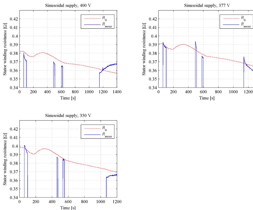
Figure A3.1 Stator winding resistance curves during the sinusoidal supply tests of 400 V, 377 V and 350 V. The resistance  $R_{\text{meas}}$  is determined from the 4-wire measurement between the tests. The resistance  $R_{\theta}$  is calculated from the stator winding temperature. The plots show that the 4-wire resistance measurement gives inconsistent results.
