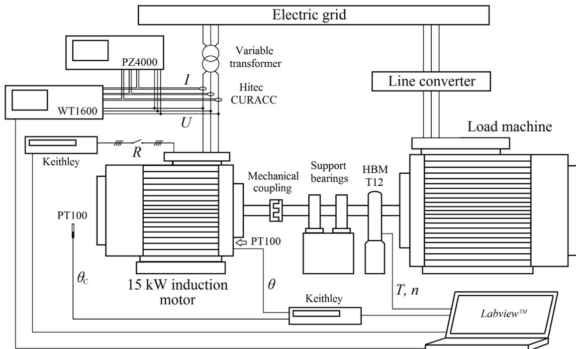
Figure 3.1. Measurement setup for tests on sinusoidal supply. The 15 kW induction motor was loaded with a larger machine. All measurement data was gathered with a LabVIEW-interface simultaneously from several instruments.
