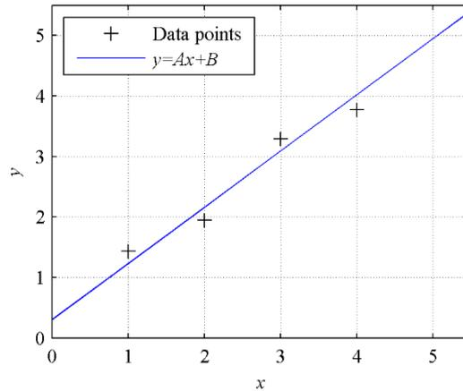
Figure A4.1 Linear regression analysis. A linear relationship  $y = Ax + B$  is formed from the known points marked with “+”.
