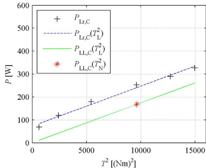
Figure 4.2. Determining the stray-load losses with the residual loss method on the 400 V, 50 Hz DTC converter supply. The dashed line is the smoothed linear relationship of the residual loss points. The residual loss points seem to be arranged in just the opposite manner when compared to Figure 4.1.
