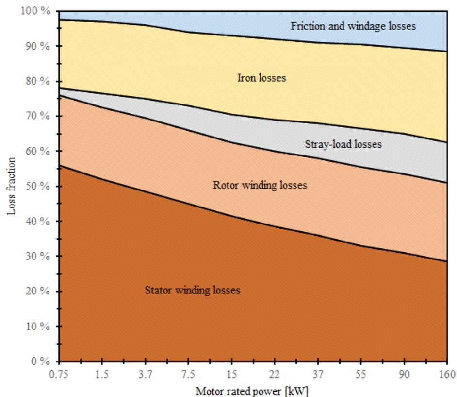
Figure 1.1. Typical loss distribution of four-pole induction motors. The figure shows relative proportions of each loss component and their dependence on the motor size (motor rated power from 0.75 kW to 160 kW). Data adopted from de Almeida et. al. (2008).
