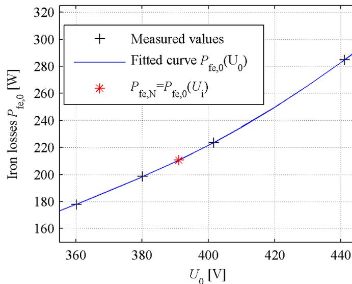
Figure 3.8. Determining the rated load iron losses. The four points marked with “+” are the values of no-load iron losses at 90 % – 110 % voltage points drawn as function of  $U_0$ . The rated load iron losses  $P_{fe,N}$  are determined by interpolating from  $P_{fe,0}(U_0)$ -curve at voltage  $U_i$ .
