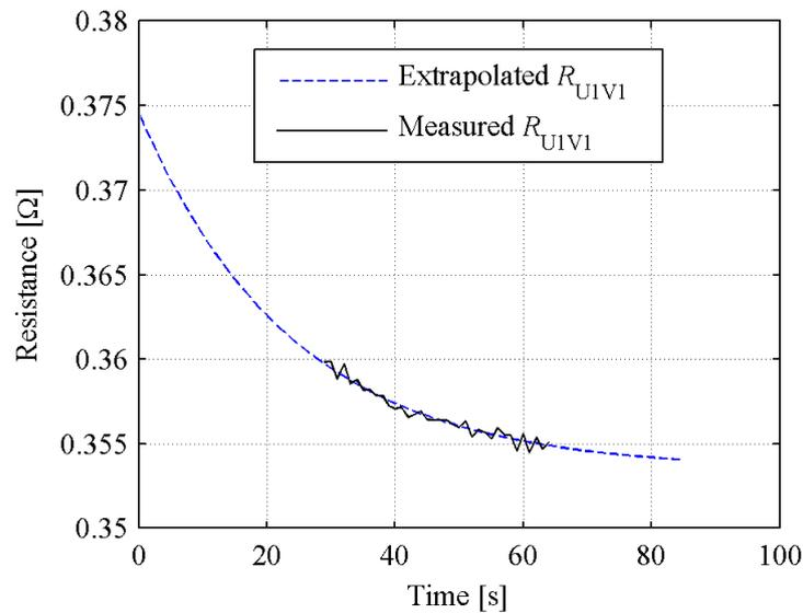
Figure A2.1. The measured and extrapolated curves for  $R_{U1V1}$  as function of time at the end of rated load test. At  $t = 0$  s, the motor was stopped from rated load. The value of extrapolated  $R_{U1V1}$ -curve at  $t = 0$  s is the rated load value  $R_{U1V1,N}$ .
