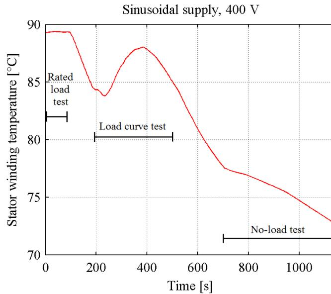
Figure 4.3. The measured stator winding temperature curve during the 400 V, 50 Hz test run on sinusoidal supply.
