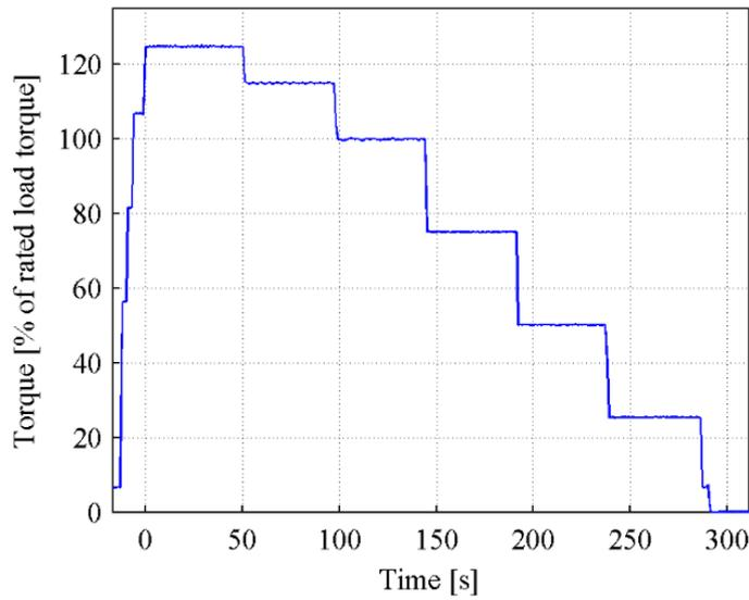
Figure 3.5. The measured torque during load curve test of the 400 V, 50 Hz test run in percents of rated load torque. The load points of 125 % to 25 % of rated load were applied in descending order and each point was run for approximately 45 seconds.
