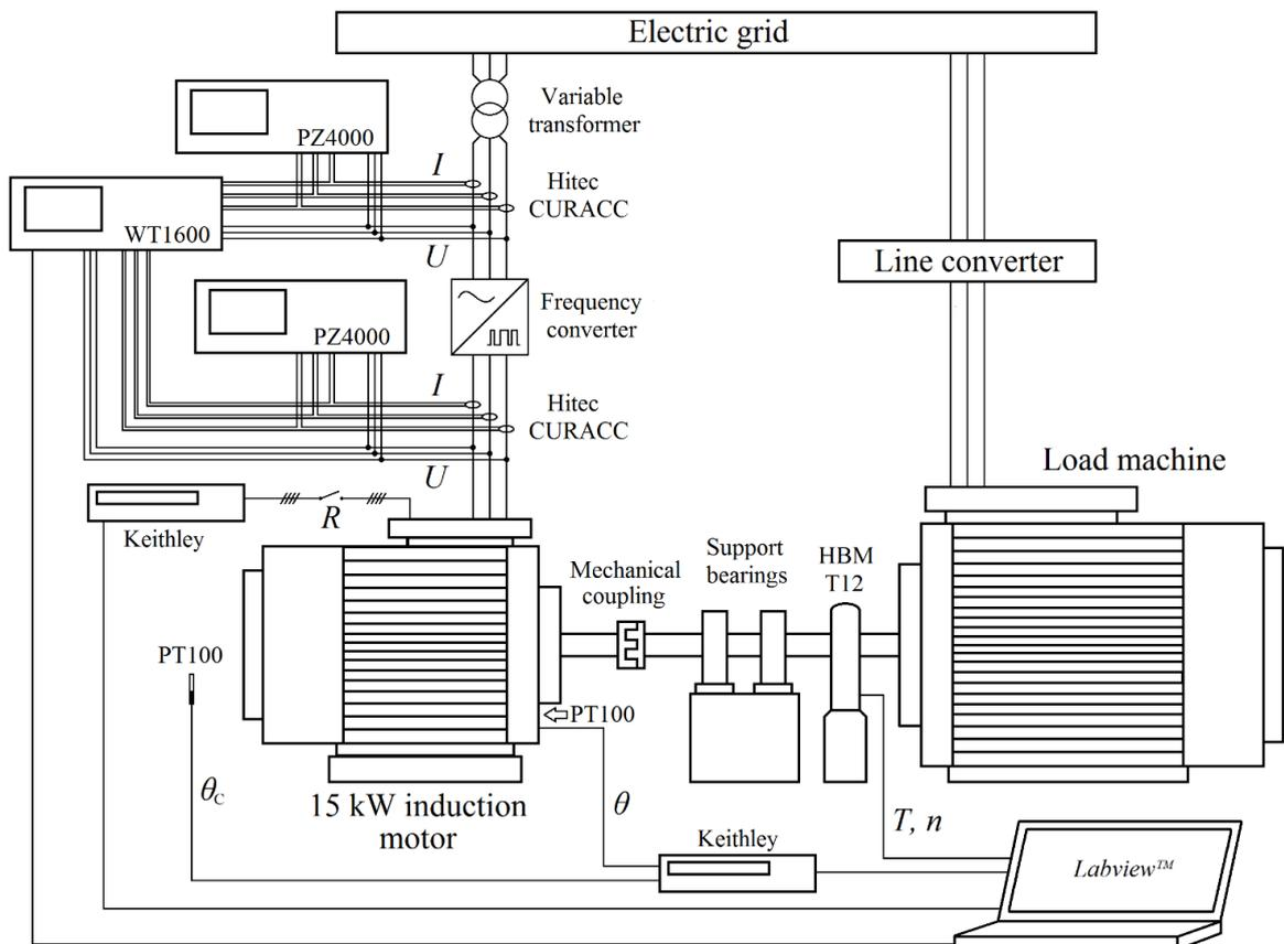
Figure 3.2. Measurement setup for tests with frequency converter supply. In addition to measurements with sinusoidal supply, the setup includes a frequency converter and output measurements of the converter supply.
