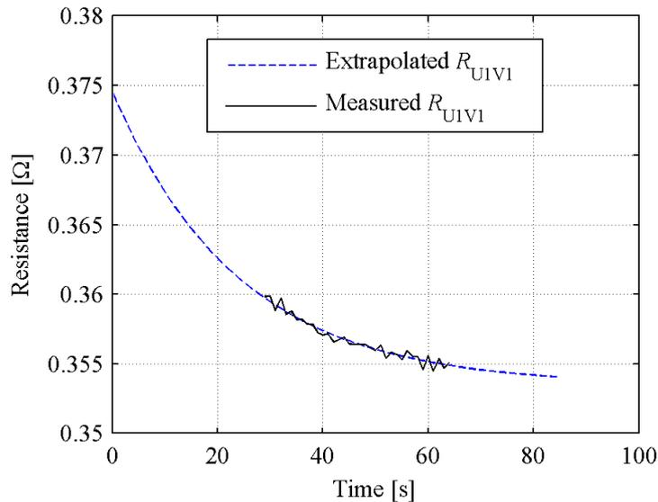
Figure 3.4. The measured and extrapolated curves for  $R_{U1V1}$  as function of time at the end of rated load test. At  $t = 0$  s, the motor was stopped from rated load. The value of extrapolated  $R_{U1V1}$ -curve at  $t = 0$  s is the rated load value  $R_{U1V1,N}$ .
