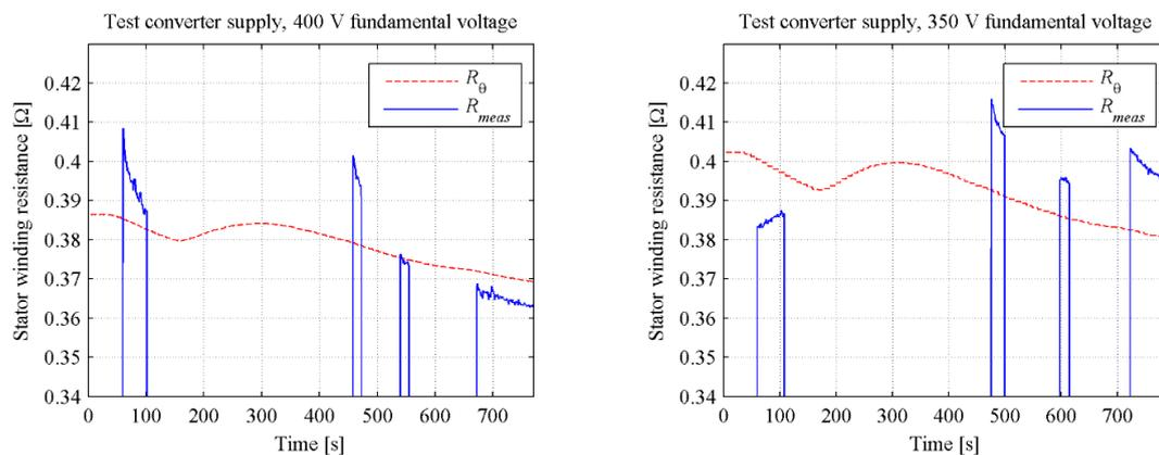
Figure A3.2 Stator winding resistance curves during the measurements on test converter supply of 400 V and 350 V. The resistance  $R_{meas}$  is determined from the 4-wire measurement between the tests. The resistance  $R_\theta$  is calculated from the stator winding temperature. The plots show that the 4-wire resistance measurement gives inconsistent results.
