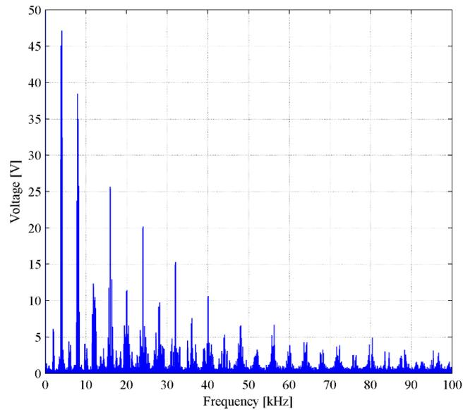
Figure 1.4. An example of harmonic content of a SVM voltage waveform with a carrier frequency of 4 kHz, fundamental voltage of 230 V and fundamental frequency of 50Hz. The fundamental frequency, which is also the first harmonic, is not visible in the plot. The most significant high frequency harmonics are located near the carrier frequency and its multiples.
