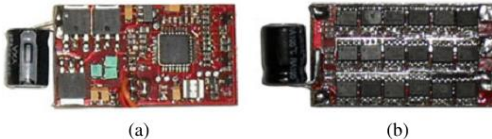
Figure 7. ESC: (a) top view; (b) bottom view (Carrillo, 2013).
