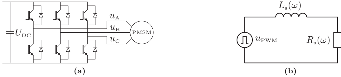
Figure 4.10: a) Three-phase voltage source inverter connected to a PM synchronous machine (PMSM). b) Simplified one-phase electrical circuit of the PMSM to model higher-order current harmonic ripple assuming the PM emf harmonics to have a much lower frequency than the switching frequency. Here, u_{\text{PWM}} [V] is the voltage harmonics (except fundamental) caused by PWM switching, L_s [H] is the synchronous phase inductance of the PM machine, whose value is a function of frequency, and R_s [ \Omega ] is the AC resistance of the stator phase coil.
