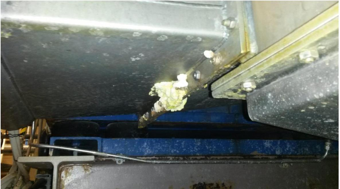
**Figure 23.** A minor leakage caused by crevice corrosion, that has crystallized and formed a “cake” that prevents further leakage in sodium chlorate pipeline.
