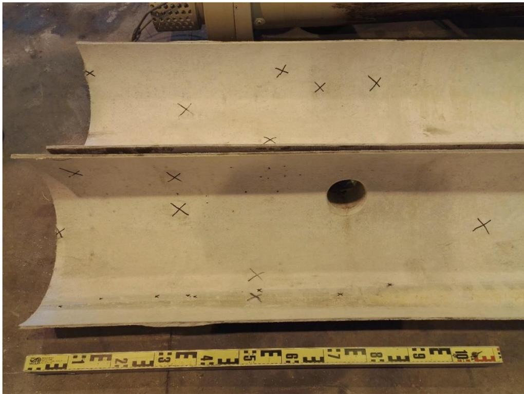
**Figure 19.** Blisters marked with an X in chlorine header pipe, with a reference gauge of 1100 mm.
