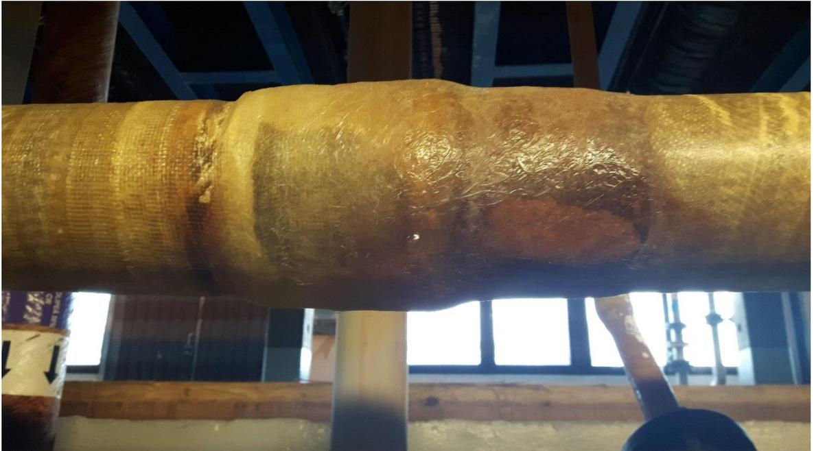
**Figure 24.** Delayering and color transformation in failed PP/FRP pipeline containing caustic soda.
