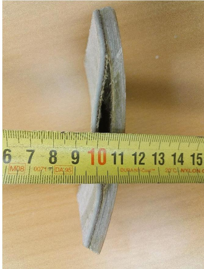
**Figure 21.** The cross-section of a permeation caused blister in ECTFE/FRP chlorine header pipe, showing that the permeation has stopped at the higher density VE-resin layer causing the bulging of the ECTFE-layer.
