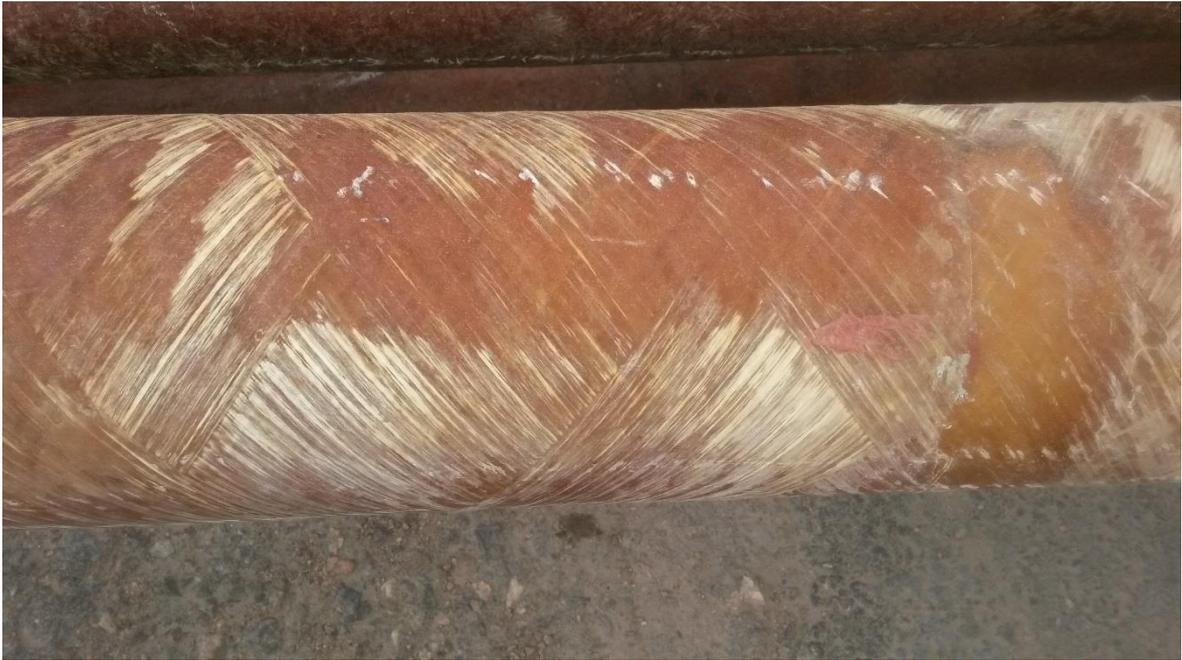
**Figure 25.** A UV-radiation caused failure in the outer layer of a NaOH PP/FRP pipeline.
