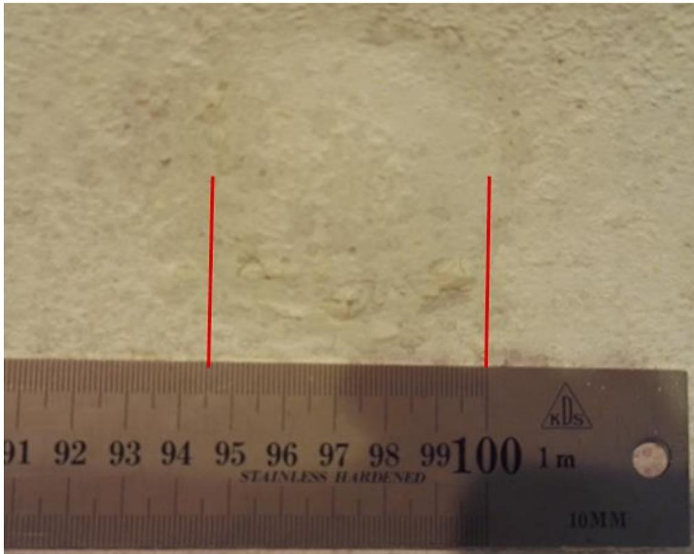
**Figure 20.** Close-up picture of an average sized blister in ECTFE/FRP chlorine header pipe.
