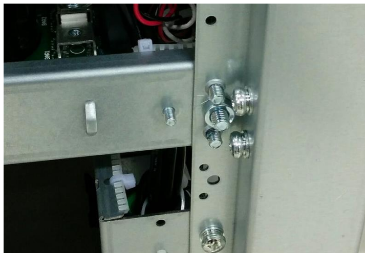
Figure 25. Three type of screws and multiple insertion direction of screws used in 93E model
