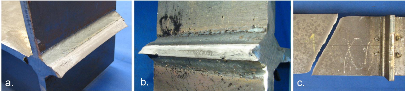
Fig. 1. Failure modes of non-load carrying joints: (a) failure at weld toe due to softening, at 45 degrees through the thickness of the base plate (according to Tresca approach); (b) failure with a double 45-degree mode; and (c) desired failure mode in the base plate outside the joint at an angle of 30 degrees over the width of the plate.
