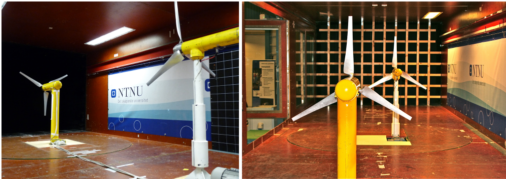
Figure 3: Model in the wind tunnel [49]: perspective (left) and from downwind (right) views.
