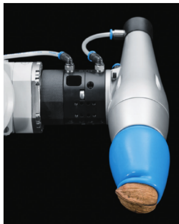
Figure 52. FlexShapeGripper: hydraulic fluid inside the silicone "chameleon tongue" grips objects by drawing them inward (Festo FlexShapeGripper n.d.).
