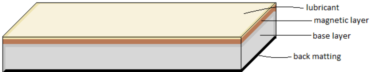
Figure 4 Composition of a magnetic tape
