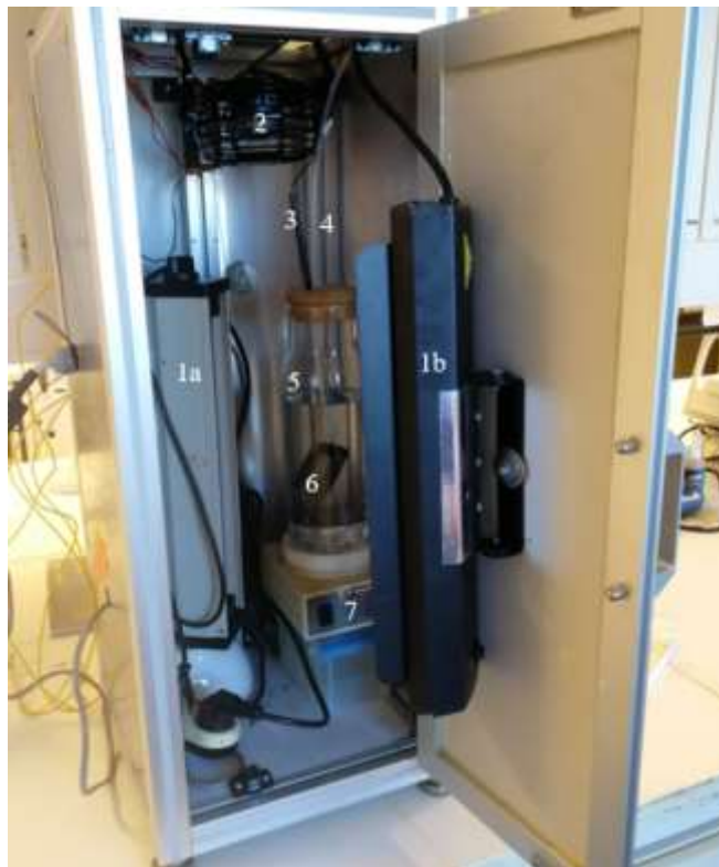
Figure 7 The UV-photocatalysis unit used for the experiments.
