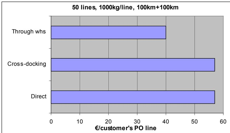
**Figure 11.** Activity costs in Cross-Docking, 50 lines, 1000kg/line, 100km+100km (Modified from Aminoff et al. 2002)
