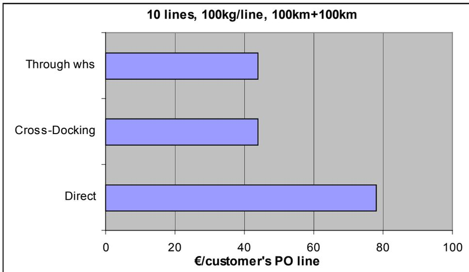
**Figure 10.** Activity costs in Cross-Docking, 10 lines, 100kg/line, 100km+100km (Modified from Aminoff et al. 2002)
