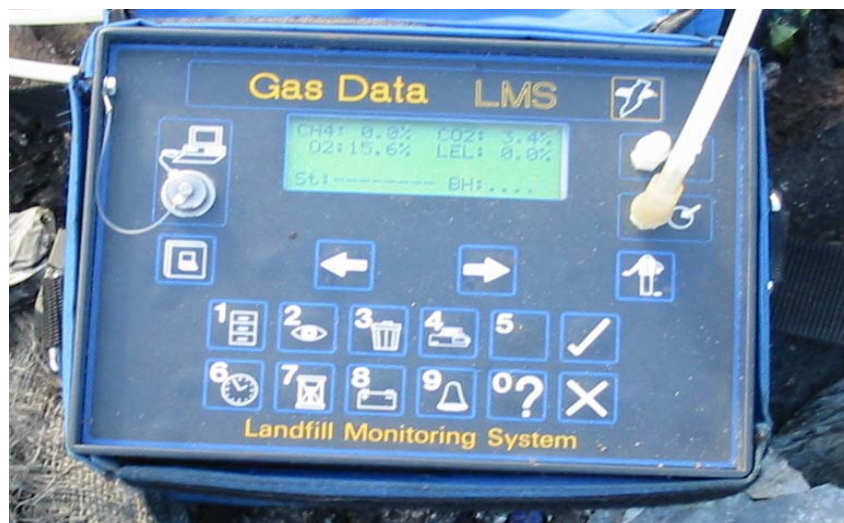
Figure 7. Landfill gas monitoring gauge.
