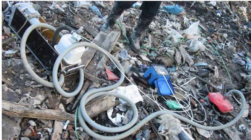
Figure 6. Landfill gas measurement system.
