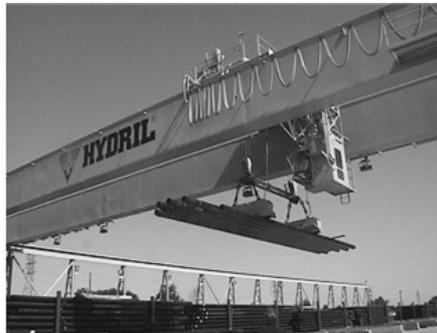
Figure 14. The original idea for solving the problem by means of an overhead crane with a magnet (source <http://www.gaussbusters.com/custom.html>).
