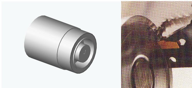
Figure 6.4. Stage 4: Face turning, turning of the cavity.
