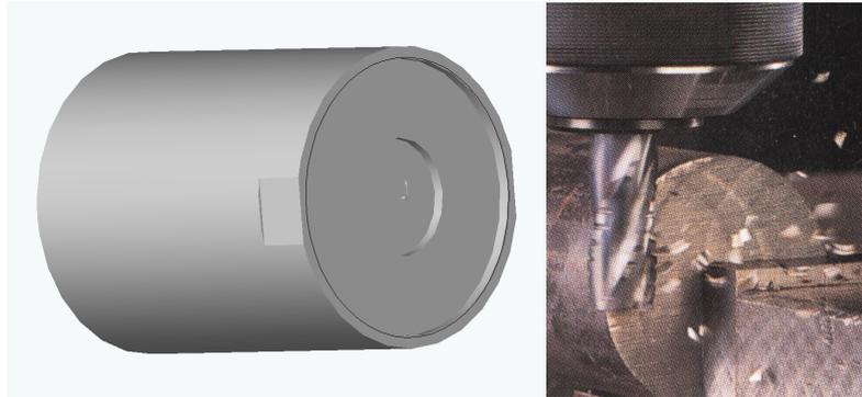
Figure 6.11. Stage 5: Milling outer geometry of the cover.
