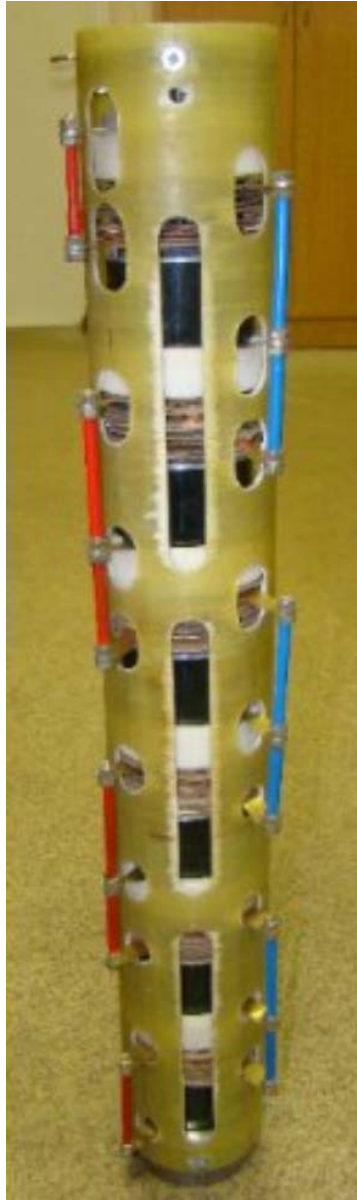
Fig.5.5 One section of the modernized NSA with resistor shunted with rod gaps. (SZP)
