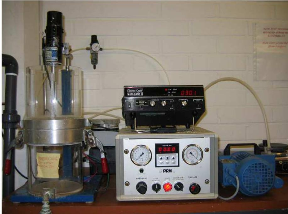
Figure 13 Turbulent Pulse Sheet Former/25/
