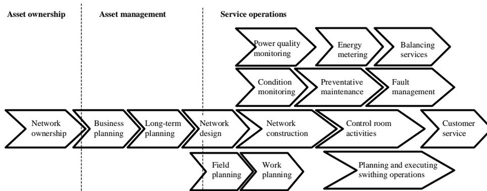
**Figure 7** Simplified illustration of operations related to managing electricity distribution networks.
