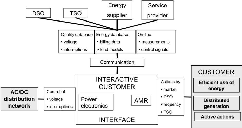
**Figure 5 Illustration of an interactive customer interface in the future electricity market.**
