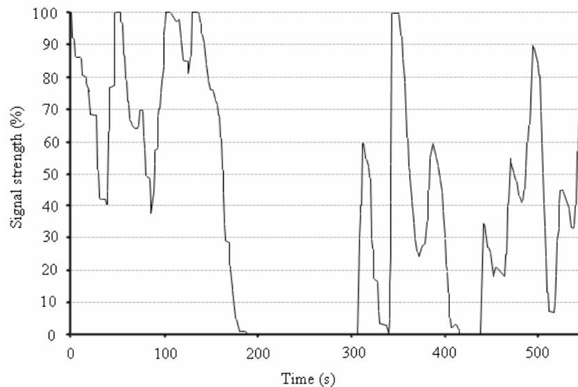
**Figure 9 Signal strength of the device in moving train [29]**
