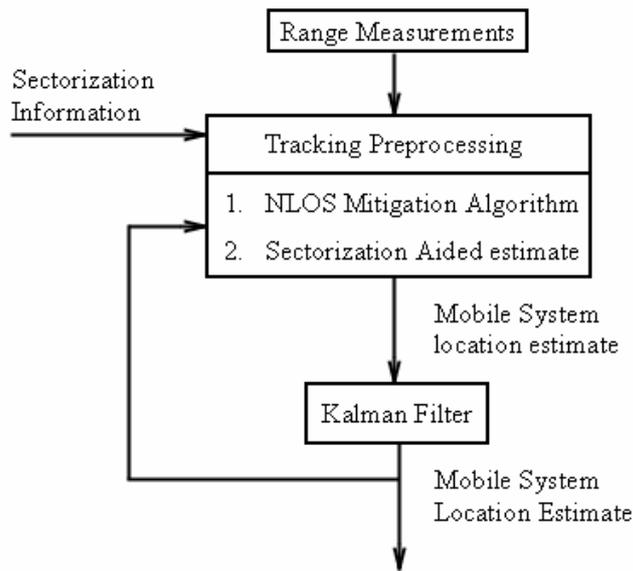
**Figure 11 Cellular Based MS Location Tracking System [34]**
