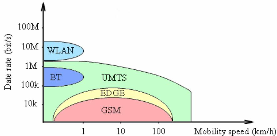
**Figure 10 Adaptable abilities of different technologies to movement**
