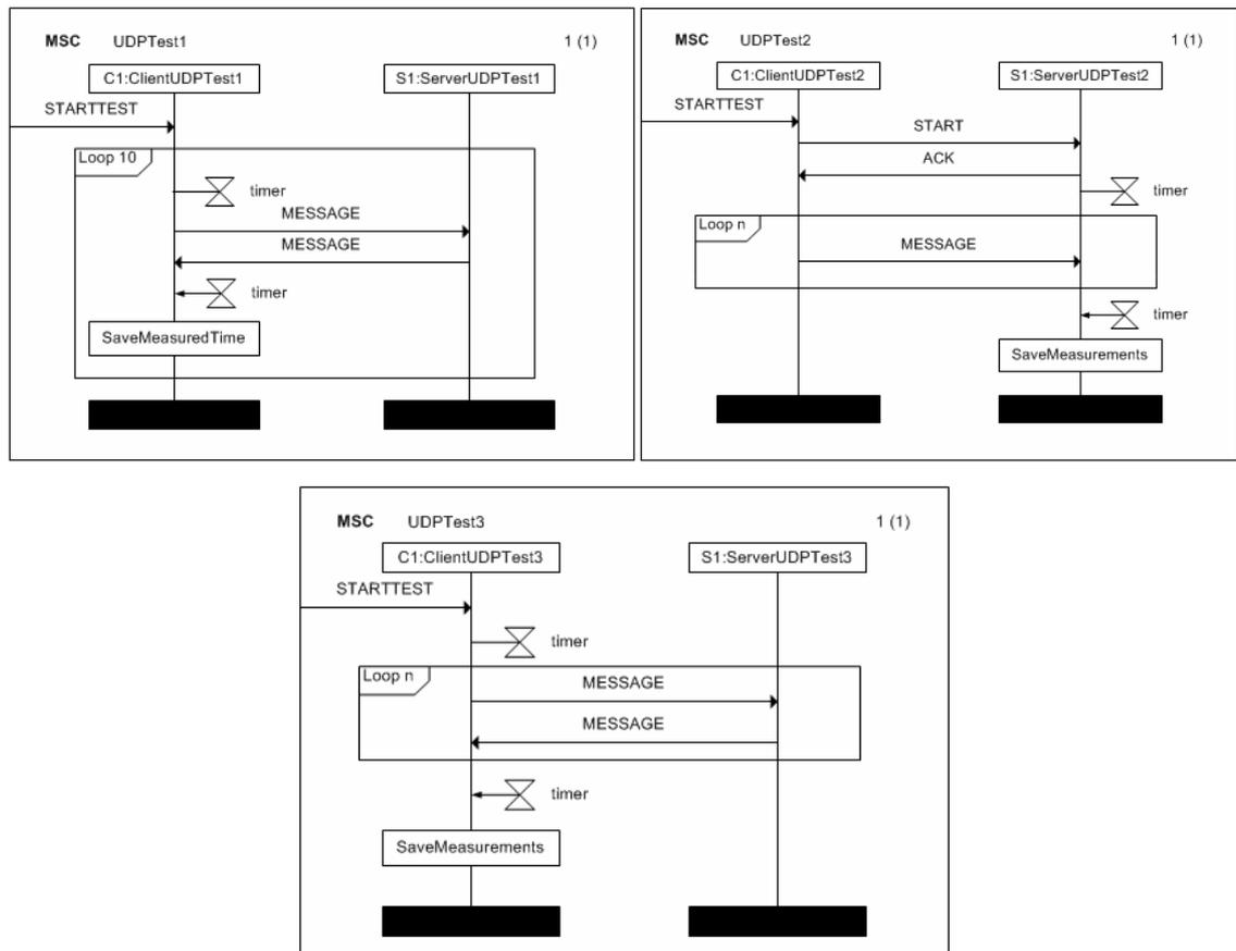
**Figure 13 MSC diagrams of UDP test (top-left: UDPTest1 – latency test, top-right: UDPTest2 – bandwidth test, down: UDPTest3 – time for package transmission)**
