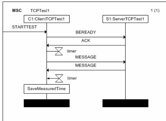
**Figure 12 MSC diagram of TCP test**
