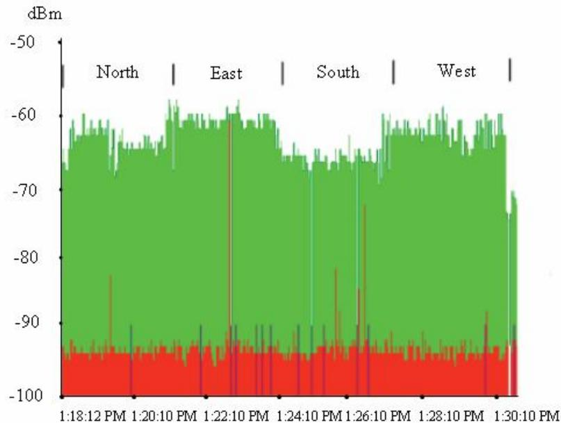
**Figure 5 Correlation between the received signal strength and the mobile device orientation (data collected on a weekday) [23]**
