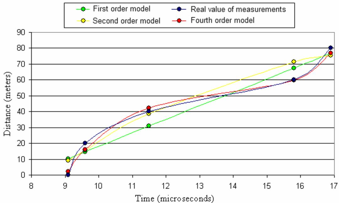
**Figure 18 Propagation models for transformation latency to distance**
