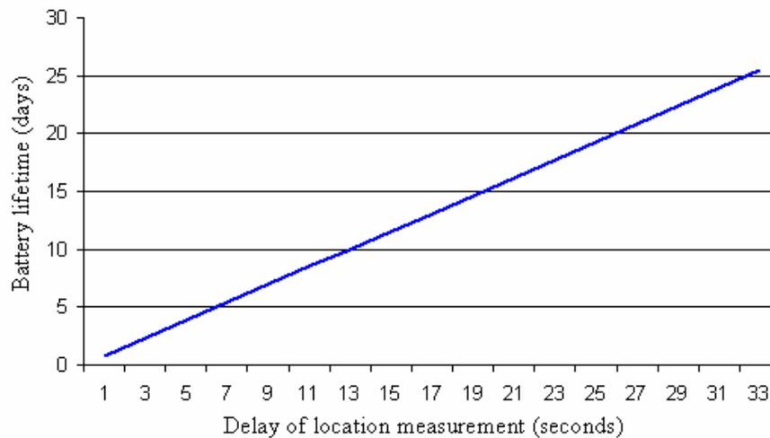
**Figure 8 Influence measurements delay to battery lifetime**
