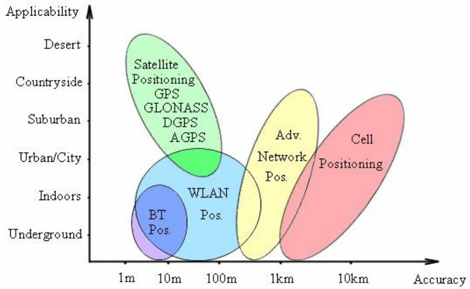
**Figure 7 Accuracy and field of application for different types of positioning [4] [26]**
