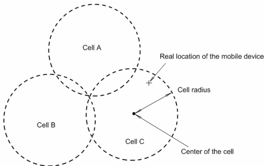
**Figure 1 Cell-coverage-based method [4]**
