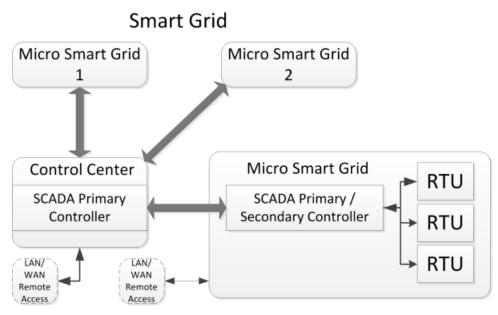
Figure 14 Proposed Smart Grid SCADA Network Layout
