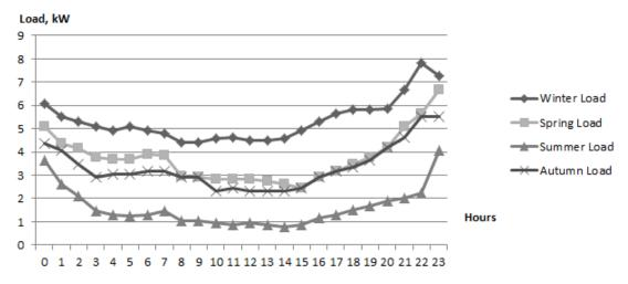
Figure 34 Load Curves for Detached Houses with Applied Growth Coefficient
