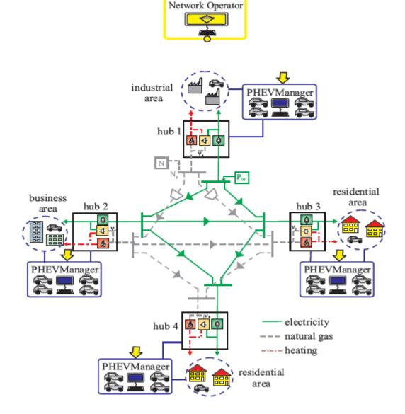
Figure 17 Energy Hub System Example
