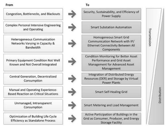
Figure 3 Transforming to Smart Grid [7]
