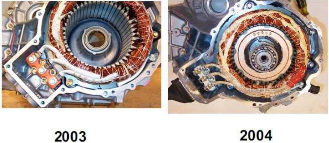
Figure 4.1 Prius 2003 and 2004 permanent magnet motors /19/
