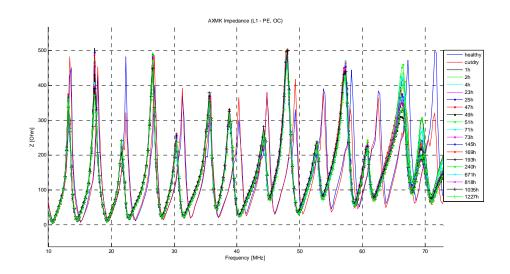
Figure 5.5. Long term impedance measurements of 25 m long AXMK cable sample. Number of hours on different curves point out the duration of which cable has been submerged under tap water with section of sheath removed. 'Healthy' and 'cutdry' are measured in dry conditions. Open circuit, measured between L1 and PEN.
