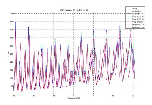
Figure 5.15. Impedance measurements of 50 m long AXMK cable sample with insulation around phases one and three gradually damaged in two steps. Open circuit, measured between L1 and L3.
