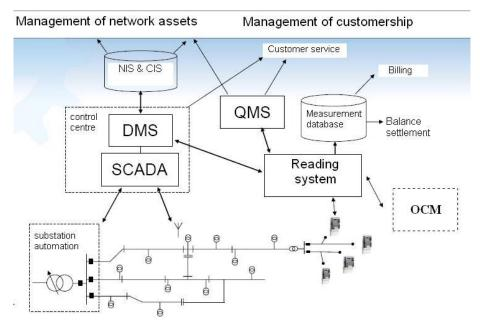
Figure 5.22. Possible integration of OCM to AMR-DMS system. (Modified from: Keränen, 2009)
