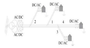
Figure 2.6. Different customer connection options in bipolar LVDC system. (Partanen et al 2010)
