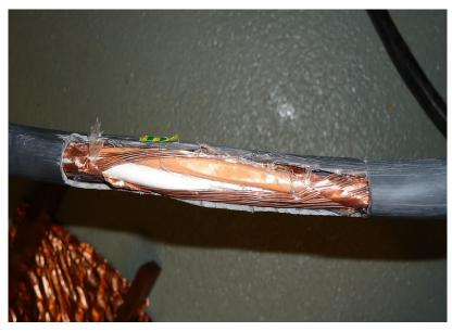
Figure 5.9. First degree damage on brown phase insulation in AMCMK cable.
