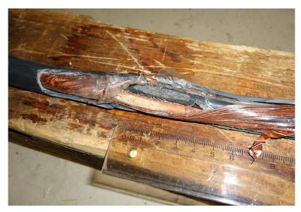
Figure 5.13. AMCMK cable with first degree damage done on brown and black phases.
