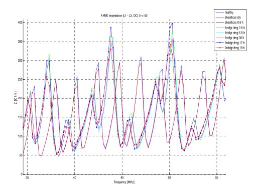
Figure 5.16. Impedance measurement results of progressive damaging of 50 m long AXMK cable sample. Close up view of Figure 5.15 of frequency band from 35 MHz to 55 MHz. Open circuit, measured between L1 and L3.
