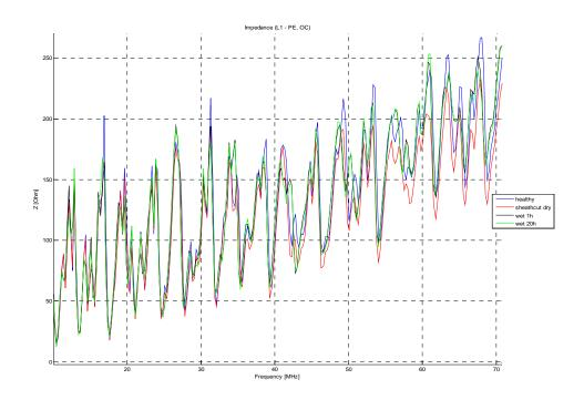
Figure 5.19. Impedance measurement results of grid setup between from the point A. Open circuit, measured between L1 to PEN.
