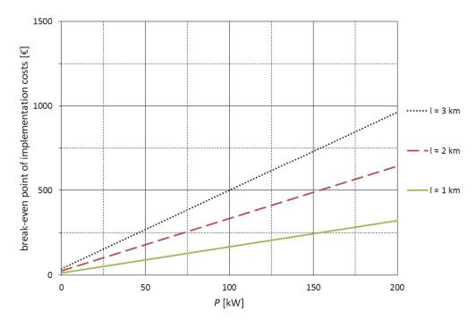
Figure 6.4. Break-even point of implementation costs of OCM to a single LV network as a function of average interruption power with different network lengths. Interconnected network, no interruption when OCM is utilized and 2 h interruption without OCM. Average power is divided between 70 % residential type and 30 % service type customers.
