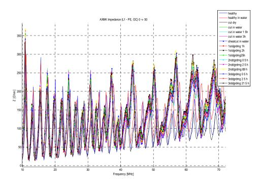
Figure 5.11. Impedance measurements of 50 m long AXMK cable sample with phase one insulation gradually damaged in three steps. Open circuit, measured between L1 and PEN.
