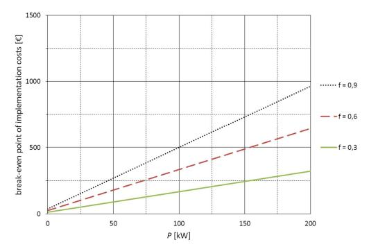
Figure 6.3. Break-even point of implementation costs of OCM to a single LV network as a function of average interruption power with different incipient fault frequencies [1 / 100 km, a]. Interconnected network, no interruption when OCM is utilized and 2 h interruption without OCM. Average power is divided between 70 % residential type and 30 % service type customers.
