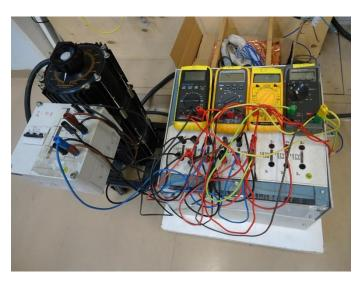
Figure 5.2. Voltage test setup. Variable autotransformer is connected to 1:1 isolation transformer in order to achieve galvanic isolation of damaged cables from common ground potential. Transformer neutral is connected to a copper plate located in water tank to provide a return path to possible phase – to – ground leakage current from damaged non-concentric AXMK cable. Phase currents and returning current from copper plate were measured using regular multimeters.
