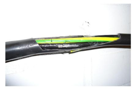
Figure 5.10. Final degree damage on brown phase insulation in AXMK cable.
