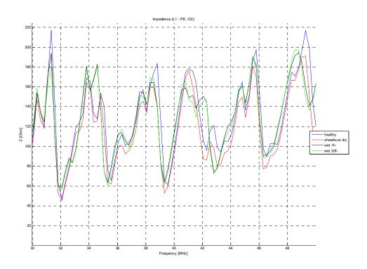
Figure 5.20. Impedance measurement results of grid setup from the point A. Open circuit, measured between L1 to PEN. Close up view of Figure 5.19 of frequency band from 30 MHz to 50 MHz.
