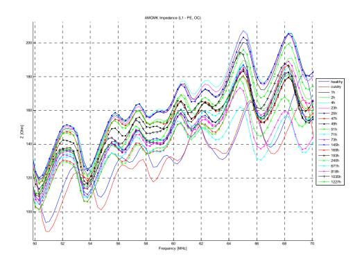
Figure 5.7. Long term impedance measurements of 25 m long AMCMK cable sample. Close up view of Figure 5.6 of frequency band from 50 MHz to 70 MHz. Open circuit, measured between L1 and PEN.
