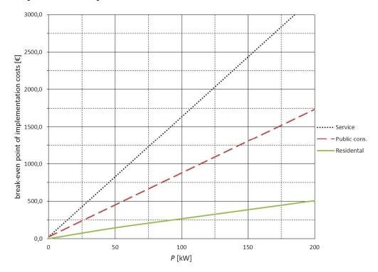
Figure 6.1. Break-even point of implementation costs of OCM to a single LV network as a function of average interruption power. No interconnections available to by-pass the fault. OCM is assumed to drop the duration of interruption from 5 h to 1 h.
