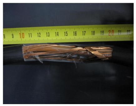
Figure 5.3. AMCMK cable with 10 cm long section of sheath and polypropylene tapes removed.
