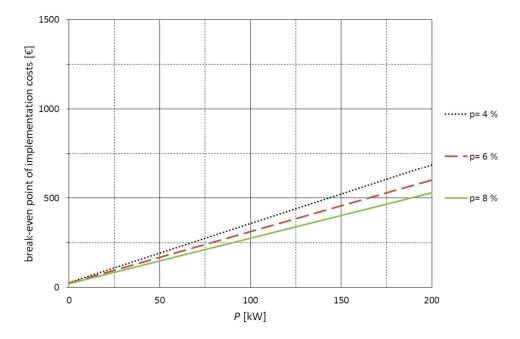
Figure 6.6. Break-even point of implementation costs of OCM to a single LV network as a function of average interruption power with different interest rates. Interconnected network, no interruption when OCM is utilized and 2 h interruption without OCM. Average power is divided between 70 % residential type and 30 % service type customers.
