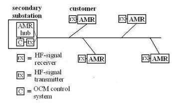
Figure 5.24. OCM system implemented to LV network with centralized read AMR meters.
