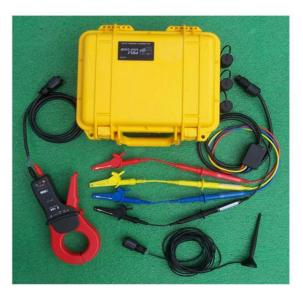
Figure 3.8. Kehui T-P22 Low Voltage Cable Fault Locator with test leads, current clamp and GSM –antenna (Kehui, 2007).
