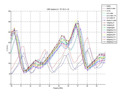
Figure 5.12. Impedance measurement results of progressive damaging of 50 m long AXMK cable sample. Close up view of Figure 5.11 of frequency band from 50 MHz to 60 MHz. Open circuit, measured between L1 and PEN.
