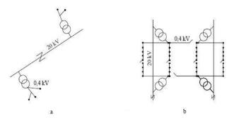
Figure 2.1. Typical a) rural and b) urban LV network. The black dots represent customers connected to the network. (Lakervi & Partanen, 2009).
