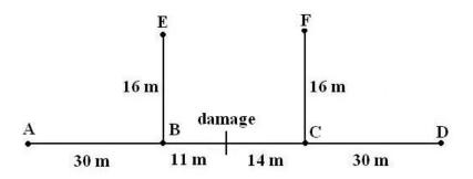
Figure 5.17. Topology of the grid setup. Grid consists of three segments of main line and two branches. Middle main line segment is damaged by cutting of a piece of sheath and submerging the cable under tap water.
