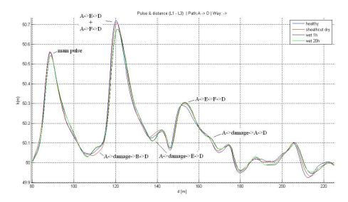
Figure 5.21. Results from gain & phase measurements from the grid point A to the point D presented in distance domain. Measured between L1 and L3 with the end of the branches being open. A value of 0,72 · c was used for signal propagation speed (Hernandez, 2012).
