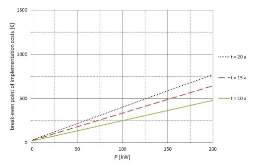
Figure 6.5. Break-even point of implementation costs of OCM to a single LV network as a function of average interruption power with different OCM system lifetimes. Interconnected network, no interruption when OCM is utilized and 2 h interruption without OCM. Average power is divided between 70 % residential type and 30 % service type customers.
