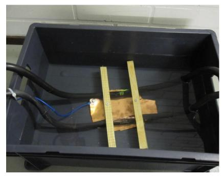
Figure 5.4. Test setup for long-term measurements. A 10 cm long section of sheath is removed from both cables and cables are submerged under tap water. Wooden clamps keep the cables securely in place and copper plate, which is connected to isolation transformers neutral, simulates the conductivity of the mass of earth.
