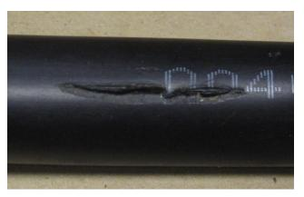
Figure 3.3. Cut in a sheath of an underwater AXMK cable. Probably caused by a propeller of an outboard engine.
