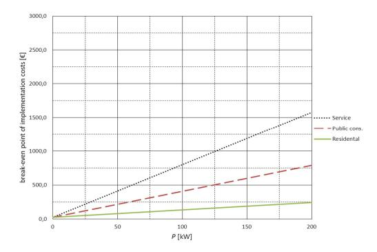
Figure 6.2. Break-even point of implementation costs of OCM to a single LV network as a function of average interruption power for different customer types. Interconnected network, no interruption when OCM is utilized and 2 h interruption without OCM.
