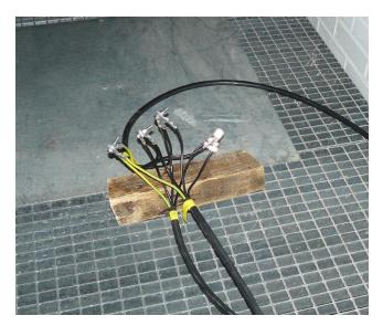
Figure 5.18. Connection point of a branch in the laboratory grid model.
