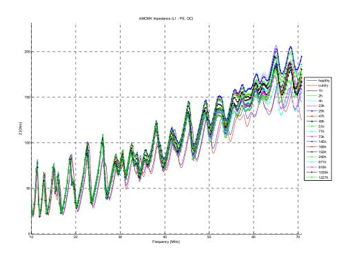
Figure 5.6. Long term impedance measurements of 25 m AMCMK cable sample. Number of hours on different curves point out the duration of which cable has been submerged under tap water with section of sheath removed. 'Healthy' and 'cutdry' are measured in dry conditions. Open circuit, measured between L1 and PEN.
