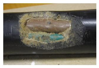
Figure 3.5. Section of sheath material and insulation of an underground AXMK cable eaten away by a mole.
