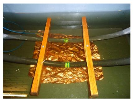
Figure 5.8. Submerged parts of first 50 m samples of both cable types with 5 cm long cut on the sheaths.
