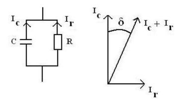
Figure 4.2. Equivalent circuit of insulation and definition of loss angle  $\delta$ .
