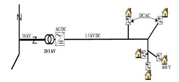
Figure 2.5. A basic concept of LVDC distribution. (Kaipia et al. 2006)
