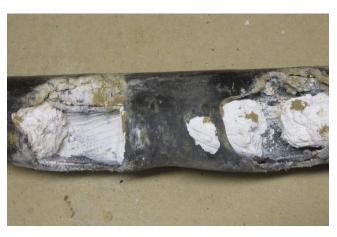
Figure 3.4. Permanently faulted part of an underground AXMK cable. Root cause of failure is probably a mole damaging the sheath.
