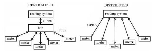
Figure 5.23. Examples of centralized and distributed communications between AMR reading system and meters. (Modified from: Valtonen, 2009)
