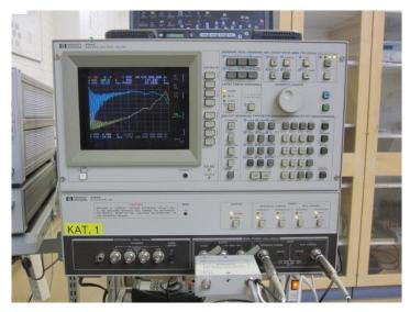
Figure 5.1. Hewlett-Packard 4194A impedance / gain-phase analyzer.
