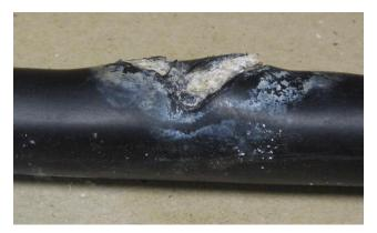
Figure 3.2. Permanently faulted part of an underwater AXMK cable. Root cause of failure is probably a propeller of an outboard engine.
