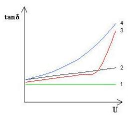
Figure 4.4. Fundamental shapes of tan  $\delta$  –curve in different condition states of insulation material (Aro et al. 2003).
