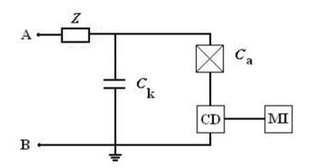
Figure 4.5. Basic concept of partial discharge measurement (Aro et al. 2003).
