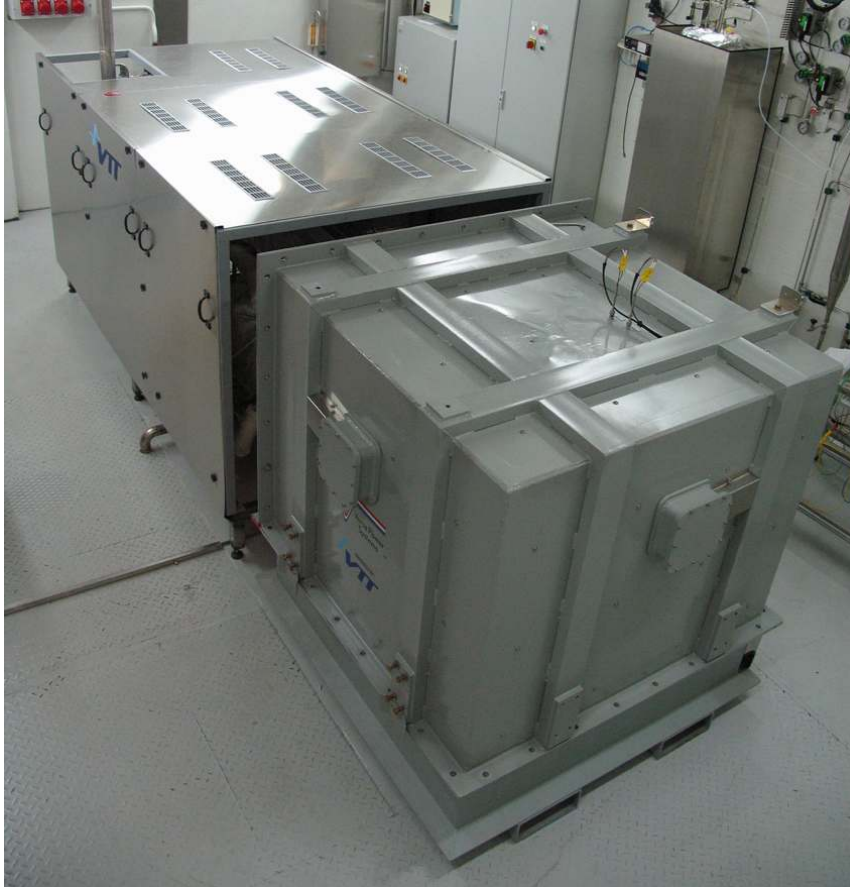
Figure 1.6. 10 kW SOFC prototype operated by VTT.
