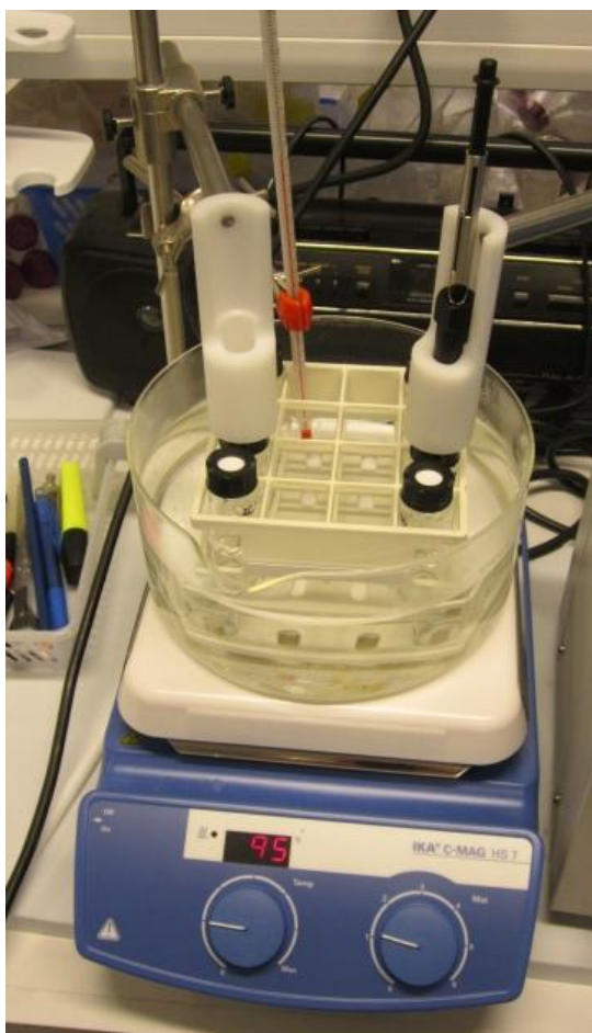
Figure 13. The water bath with vials, SPME instrument and thermometer.
