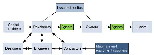
Fig. 2.1: Commercial relationships in the building supply chain. Complexity of interactions among these participants is one of the barriers to energy efficient buildings. [WBCSD, 2009].
