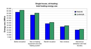
Fig. 5.2: The effect of different energy renovations on the total heating energy use of an oil-heated house in two Finnish towns; Helsinki in Southern Finland and Jyväskylä in Central Finland [Holopainen, 2008].
