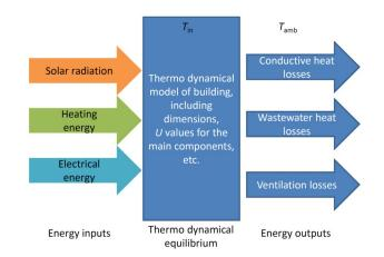
Fig. 6.1: Operational principle of the energy efficiency classification tool. It calculates the annual building heat energy consumption based on the given technical details of the building.
