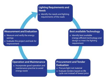
Fig. 4.1: Generic steps to increase energy efficiency in street lighting [USAID, 2010].
