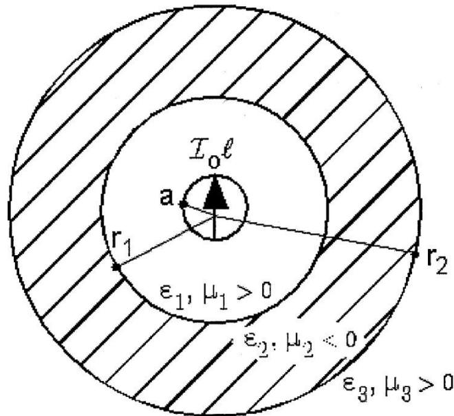
**Figure 5.1** [17]. An infinitesimal electric dipole with a length of  $l$  placed in RHM 1 and separated from RHM 3 by LHM 2
