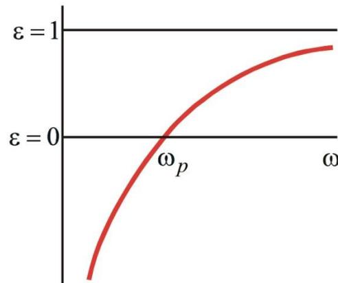
**Figure 2.1** [3]. A qualitative representation of the typical dependence of the real part of the permittivity of a plasma on frequency. Below the plasma frequency, this value is negative
