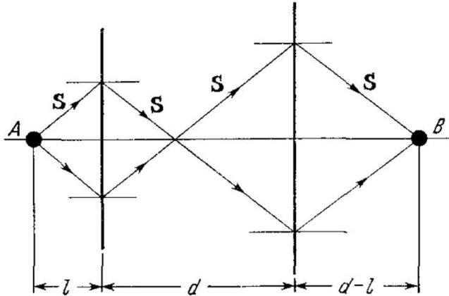
**Figure 4.2** [1]. Light propagating through a LHM-slab gets focused twice: once within the slab and then out of the boundaries of the slab (point B).
