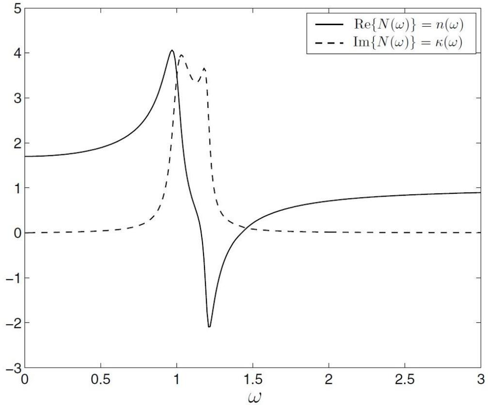
**Figure 1.2** [12]. The real part of the refractive index may change its sign within the framework of the single resonance Lorentzian model for complex  $\epsilon$  and  $\mu$ . Here  $\omega_{0e} = 1$ ,  $\omega_{pe} = 1$ ,  $\gamma_e = 0.1$ ,  $\omega_{0m} = 1.2$ ,  $\omega_{pm} = 0.8$ ,  $\gamma_m = 0.05$
