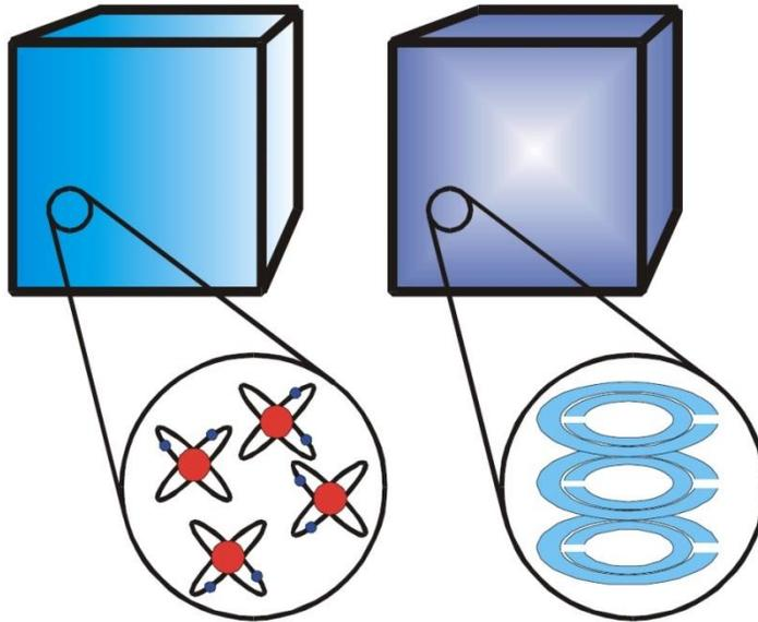
**Figure 2.14** [3]. Permittivity and permeability of conventional materials are governed by the properties of their atoms/molecules, whereas those of metamaterials – by the properties of the elementary unit cells which may contain many atoms
