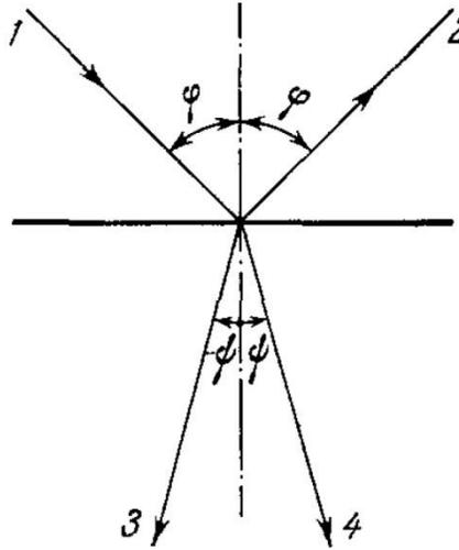
**Figure 1.1** [1]. Refraction and reflection when the two media have the same and different rightness. 1 – incident ray, 2 – reflected ray, 3 - refracted ray if the lower medium is left-handed (the refraction angle is negative in this case), 4 - refracted ray if the lower medium is right-handed. The upper medium is presumed to be right-handed
