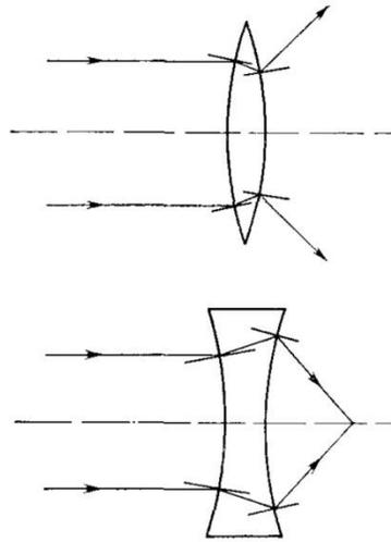
**Figure 4.1** [1]. Lenses made of a LHM focus light rays in a “reversed” manner as compared to conventional materials
