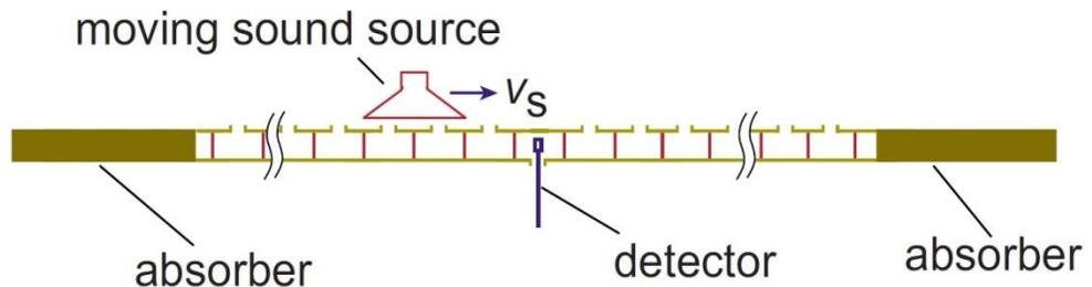
**Figure 3.6** [10]. The experimental setup for the verification of the reversed Doppler effect
