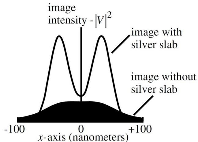
**Figure 4.5** [11]. The calculated intensity distribution along the transverse coordinate
