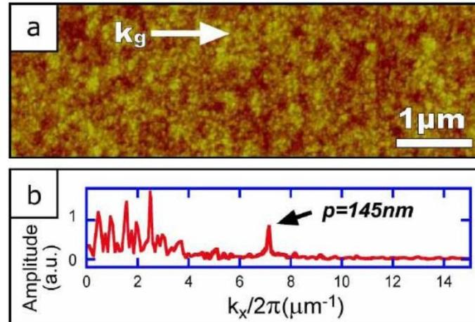
**Figure 4.11** [14]. The image of a 145 nm period grating and the Fourier transform of it
