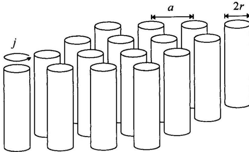
**Figure 2.4** [6]. A periodic structure constituted by metallic cylinders
