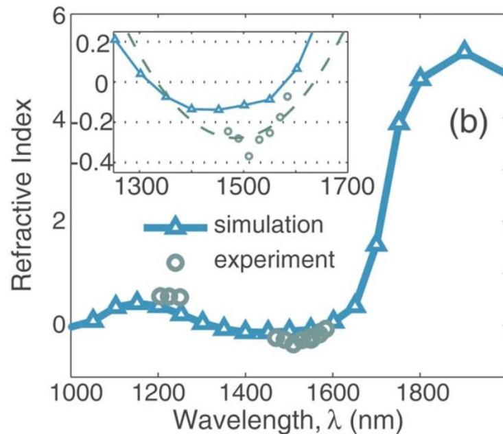
**Figure 2.13** [8]. The experiment and simulation results representing the real part of the refractive index of the double-periodic structure described above as a function of wavelength. The real part of the refractive index is negative in the vicinity of a wavelength of 1500 nm
