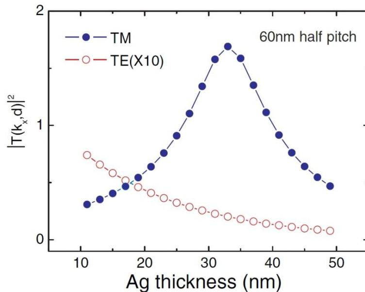
**Figure 4.15** [15]. The results of calculations for the image transfer function defined as  $|E_{\text{image}}|/|E_{\text{object}}|$ . The object is presumed to have a 60 nm half-pitch
