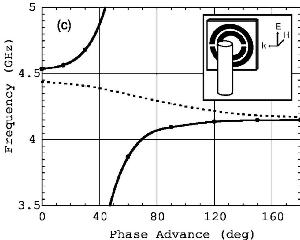
**Figure 2.11** [7]. Frequency versus  $kd$ . Ring parameters:  $c = 0.8$  mm,  $d = 0.2$  mm,  $r = 1.5$  mm; lattice constant  $a = 8.0$  mm
