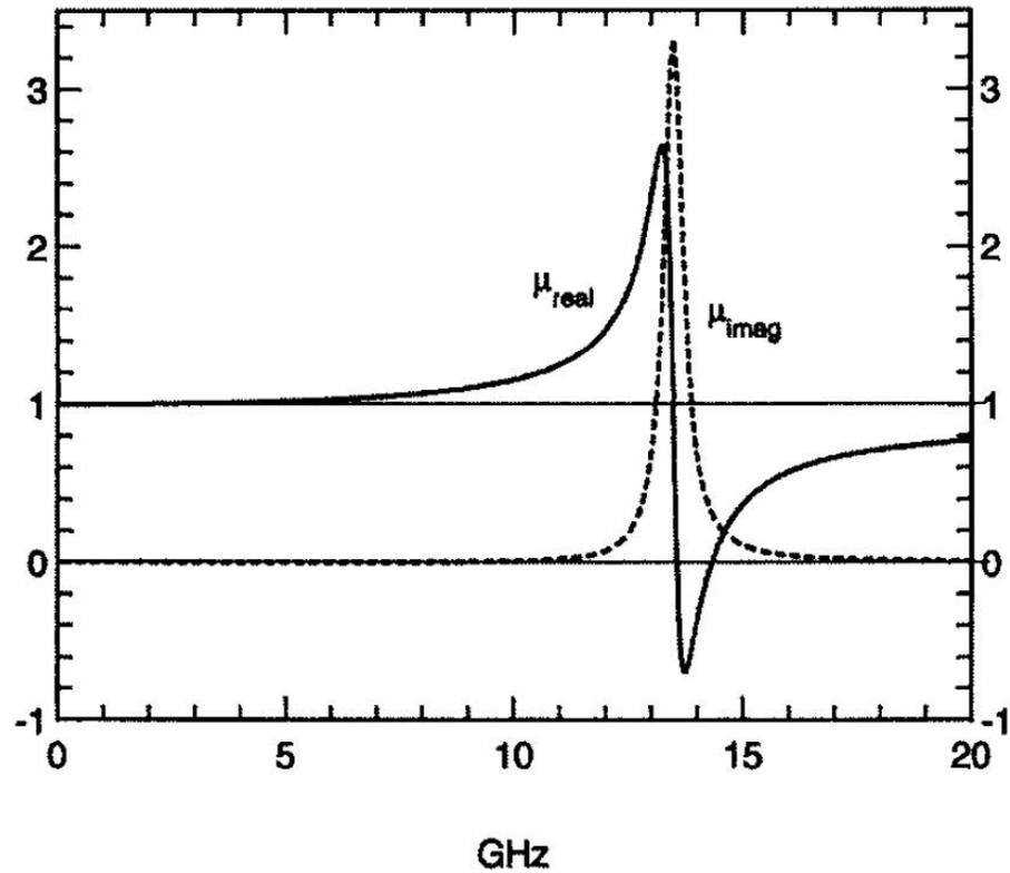
**Figure 2.9** [6]. The real and imaginary part of the permeability of the system of stacked rings as functions of frequency.  $a = 10^{-2}$  m,  $c = 10^{-3}$  m,  $d = 10^{-4}$  m,  $l = 2 \cdot 10^{-3}$  m,  $r = 2 \cdot 10^{-3}$  m,  $\sigma = 2 \cdot 10^3$  ohm/m
