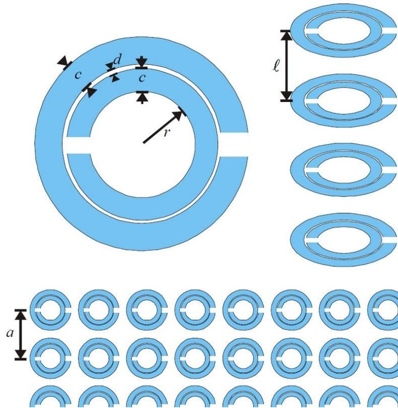
**Figure 2.8** [3]. The geometry of the split rings and their arrangement
