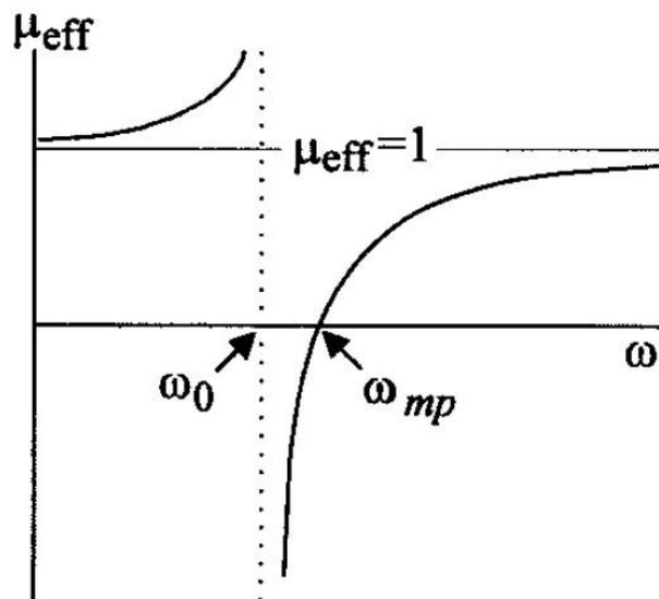
**Figure 2.7** [6]. The effective permeability of an array of the two-sheet cylinders. The material is presumed to be highly conductive
