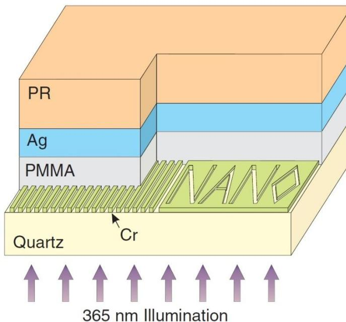
**Figure 4.12** [15]. The experimental setup investigated by Fang et al. The thickness of the silver slab is 35 nm, the thickness of the PMMA layer is 40 nm. PR means photoresist
