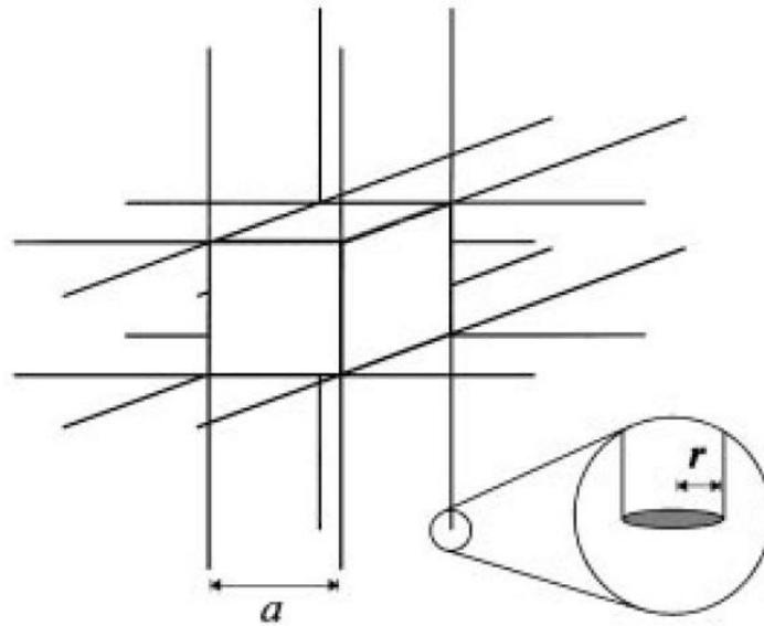
**Figure 2.2** [5]. The periodic structure composed of thin wires mimicking the dielectric response of a plasma
