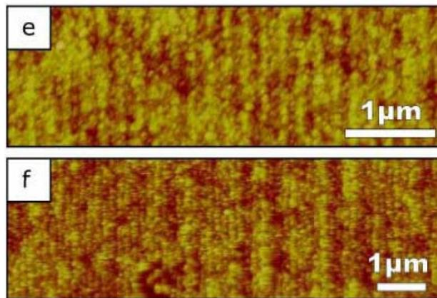
**Figure 4.10** [14]. Gratings with periods below the diffraction limit were resolved during the experiment. The images correspond to the 200 nm (the upper image) and 170 nm (the lower image) period gratings
