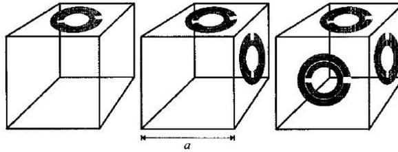
**Figure 2.10** [6]. Making a cubic unit cell of an isotropic material with split rings
