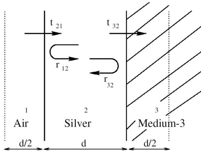
**Figure 4.6** [13]. Geometry of an asymmetric lens system
