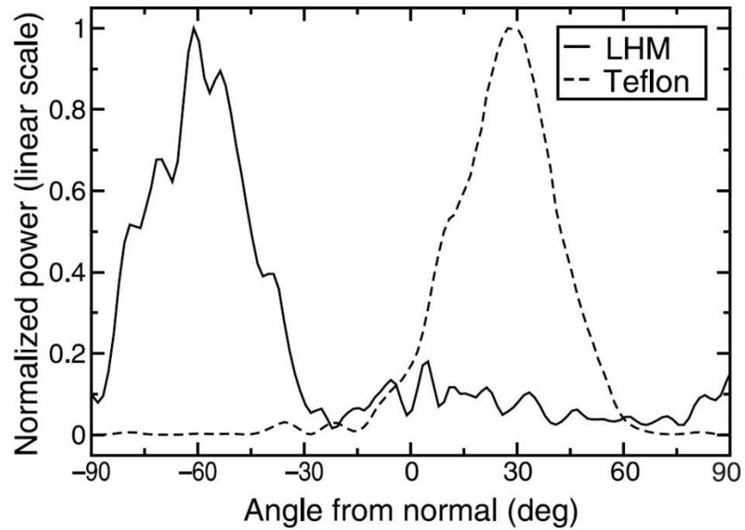
**Figure 3.3** [9]. The transmitted power measured versus the presumed refractive angle. The beam width is due to diffraction at the exit of the incident channel and the angular sensitivity of the detector being independent of the properties of the samples investigated
