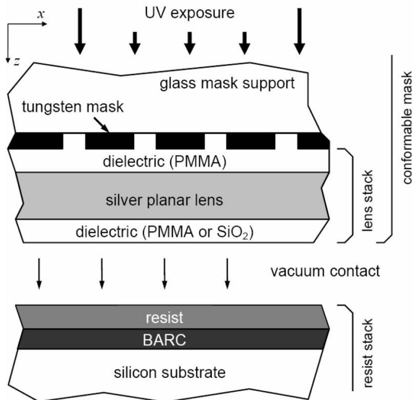
**Figure 4.9** [14]. The experimental near field imaging arrangement investigated in [14]. BARC means bottom antireflection coating, PMMA means polymethylmetacrylate
