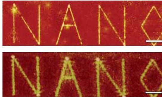
**Figure 4.14** [15]. The upper image was obtained with the silver slab, the lower – with a PMMA layer instead of it. The scale bar is 2  $\mu\text{m}$ , the width of the lines is 40 nm
