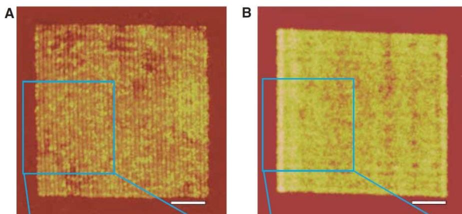
**Figure 4.13** [15]. Image of the grating described above in the presence of the silver slab (A) and in the absence of it (B). The scale bar is 1  $\mu\text{m}$
