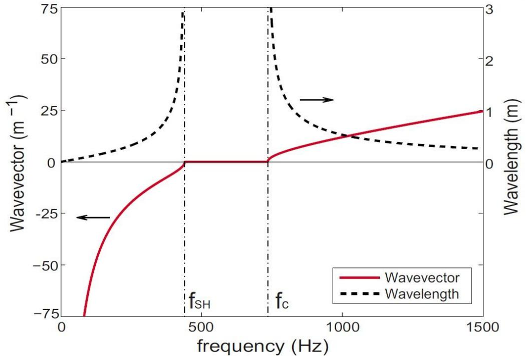
**Figure 3.5** [10]. The wavenumber and wavelength of the medium described above versus frequency. The medium is double-negative below  $f_{SH}$  and double-positive above  $f_C$ . The gap between these cut-off frequencies corresponds to evanescent waves
