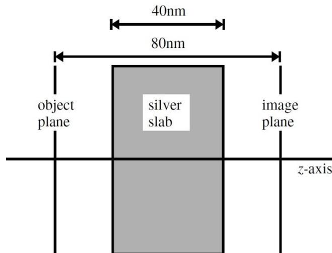
**Figure 4.3** [11]. A slab is presumed to be made of silver in order to model the amplification of evanescent waves in the electrostatic limit
