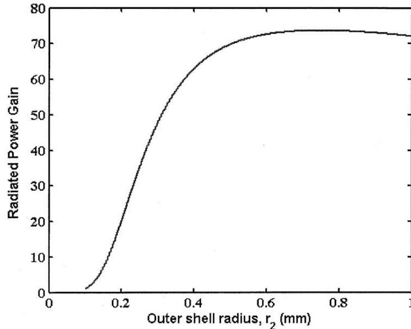
**Figure 5.2** [17]. The radiated power gain of a dipole surrounded by a shell made of an LHM with  $n = -1$  versus the outer radius of the shell. The maximum value of the gain for the values of the parameters of the problem described above takes place at  $r_2 = 748.8 \mu\text{m}$
