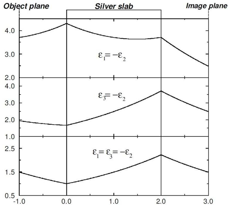
**Figure 4.7** [13]. Calculation results for field strength dependence on the z-coordinate within and in the vicinity of a silver slab for the symmetric and the both asymmetric configurations described above
