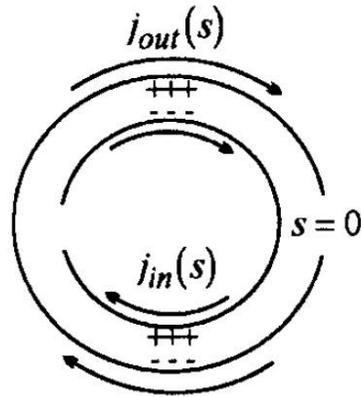
**Figure 2.6** [6]. The capacitance of the structure enables the external magnetic field parallel to its axis to induce current in it
