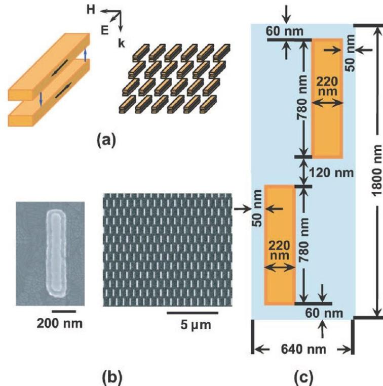
**Figure 2.12** [8]. (a) The double periodic array of pairs of parallel gold nanorods and the incident field; (b) FESEM-images of the array of rods and a single rod; (c) geometrical parameters of the elementary cell of the array
