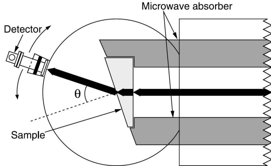
**Figure 3.2** [9]. A prism-shaped sample is placed between the circularly shaped metallic plates (shown transparent). A detector rotates around the plates and records the transmitted power spectrum. The thick solid black line depicts the path of the microwave beam if the sample is made of a RHM. The dashed line is the normal to the material-air interface where the beam gets refracted
