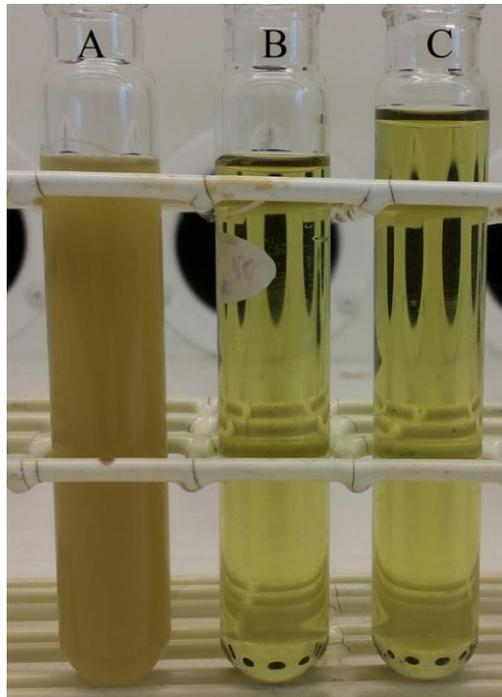
Figure 13. Real oil-water emulsion filtration with 3.5 vol% MAA\_2 membrane. A is feed solution, B is permeate for first two hour filtration and C is permeate for the last two hour filtration. Filtration conditions:  $T = 24 \pm 2$  °C,  $p = 3$  bar,  $FR = 1.4$  m/s,  $Re = 2900$ .
