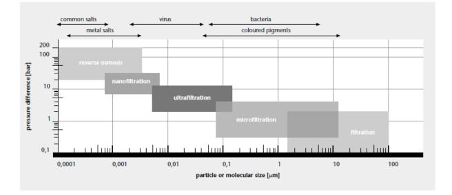
Figure 8: Classification of membrane processes based on particle size (Plnnekamp & Friedrich, 2003)
