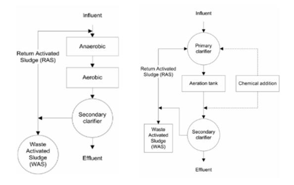
Figure 6: Biological and chemical process for phosphorus removal (MCPA, 2006)
