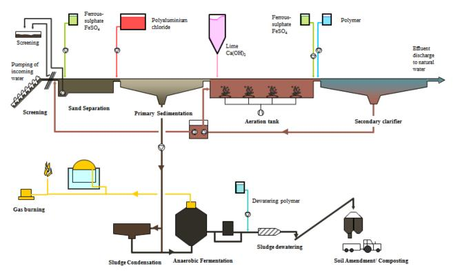
Figure 4: Conventional Activated Sludge Process at Kenkäveronniemi WWTP, Mikkeli, Finland
