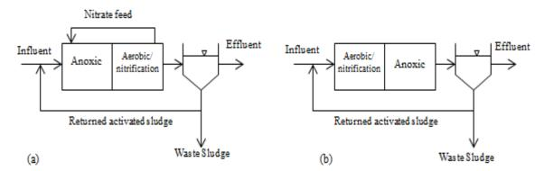
Figure 5: (a) Pre-anoxic and (b) Post-anoxic denitrifications (Metcalf & Eddy, 2003)
