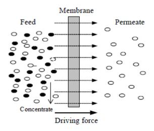
Figure 7: Membrane filtration principle (Abeyanyaka, 2009)
