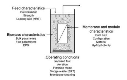
Figure 15: Interrelationships of parameters affecting membrane fouling (Le-Chech et al., 2006)
