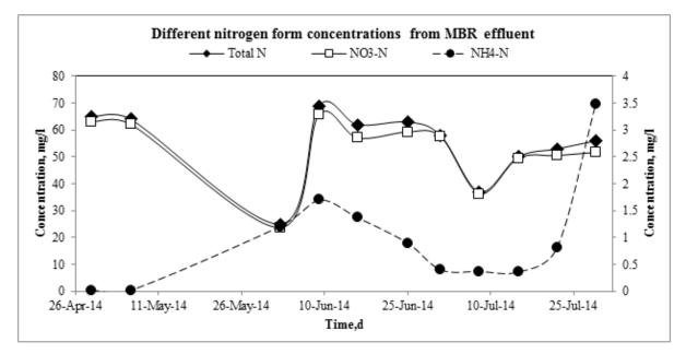
Figure 31: Concentration of different nitrogen from MBR effluent
