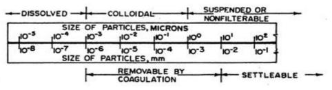
Fig. 2 below shows the classification and size ranging of solids constituents in wastewater.
