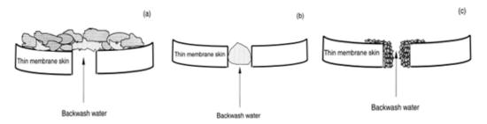
**Figure 13:** Membrane fouling mechanisms: (a) Gel/ cake formation (b) Pore plugging (c) Pore narrowing (Bourgeous et al., 2001)
