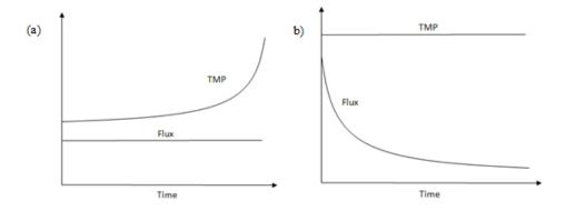
Figure 12: (a) Constant flux mode (b) Constant TMP mode
