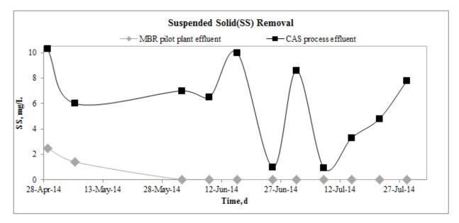
Figure 28: Total suspended solids removal
