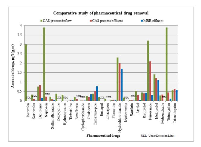
Figure 33: Concentrations of selected PPCPs in CASP influent & effluent and MBR permeate
