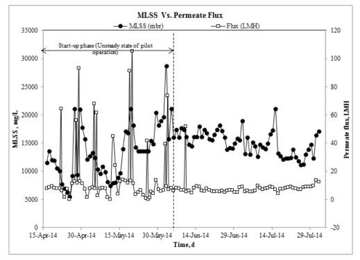
Figure 19: MLSS concentration vs. permeate flux
