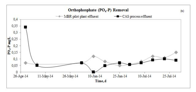
Figure 29: (a) Total phosphorus, (b) PO4-P removal
