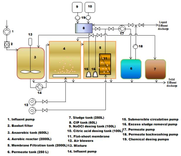
Figure 18: Schematic diagram of MBR pilot plant set up
