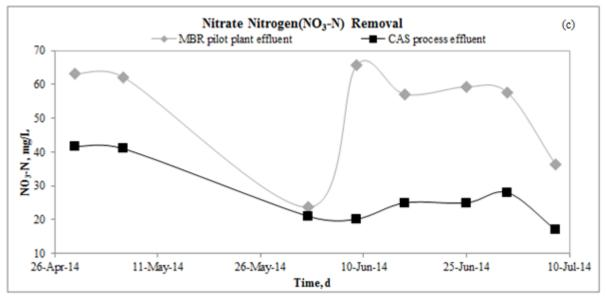
Figure 30: Nitrogen (a) TN (b) NH<sub>4</sub>-N (c) NO<sub>3</sub>-N removal
