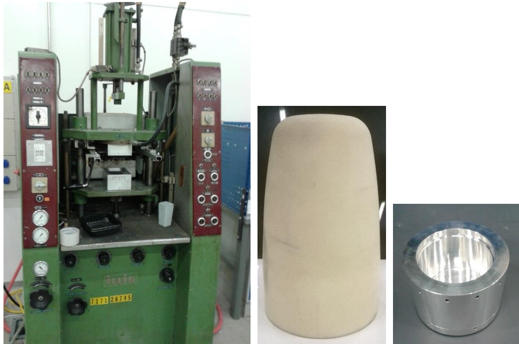
Figure 30 ILLIG forming machine (left), plug (center) and lower mold (right). (Coveris)
