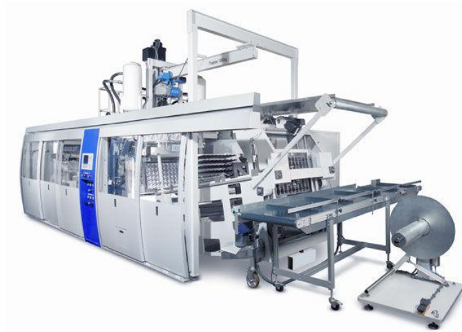
Figure 11 A thermoforming machine. The heated sheet is formed and cut in the mold section and products are stacked and transferred to the belt. The film strip is wound to the grinder and blown back to use. (Gabler)
