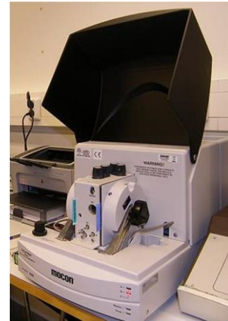
Figure 34 GTR testing method in theory and in the Mocon Ox-tran device in practice. (Labthink 2013, Tampere University of Technology 2014)
