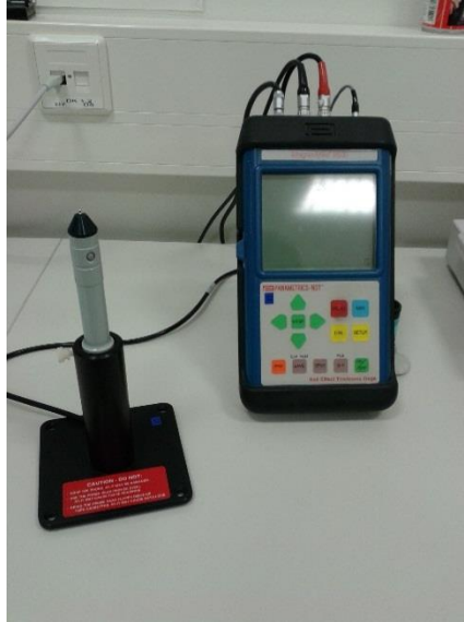
Figure 32 Magna-Mike 8500 ball measuring machine (Coveris)
