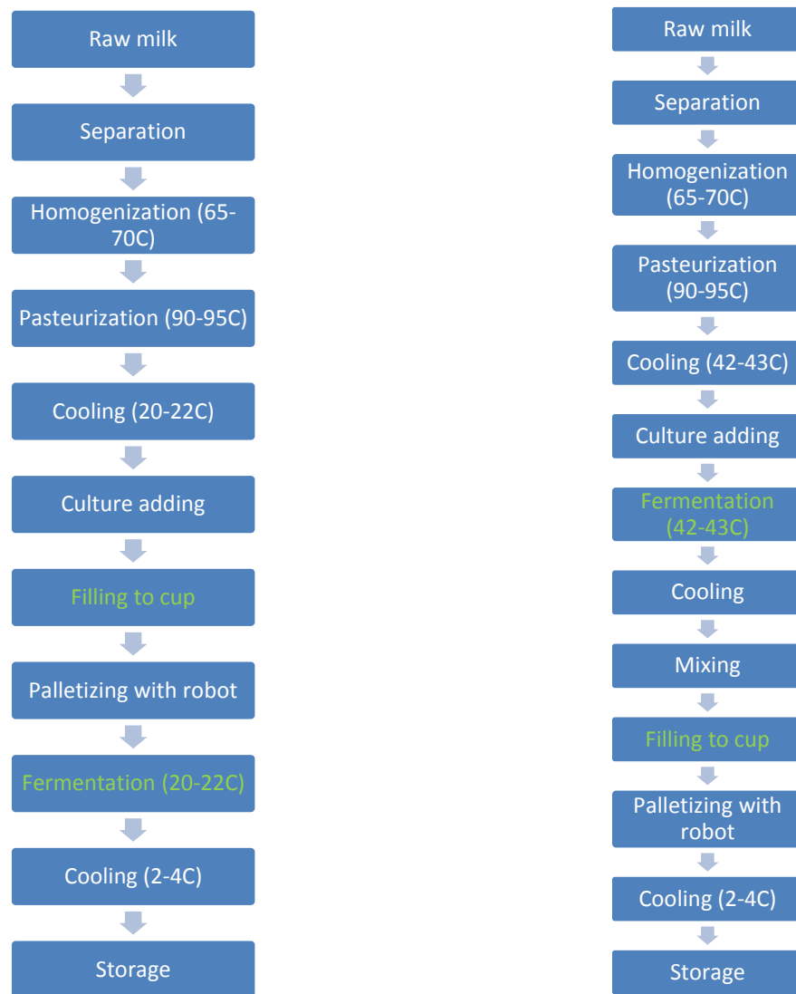
Figure 24. The processes of viili (left) and yogurt (right) (Kukkonen 2012; Väistö 2010)
