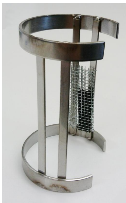
Figure 5. The metal stand for catalyst installation in the autoclave.
