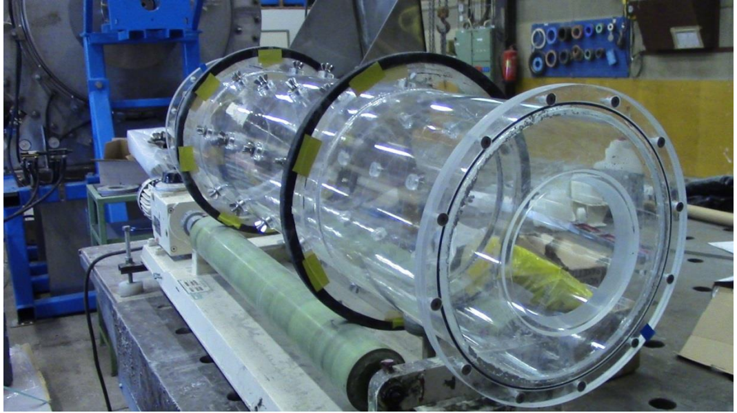
Figure 20 The rotating drum used in the experiments. Feed end on the left of the drum and discharge end on the right.
