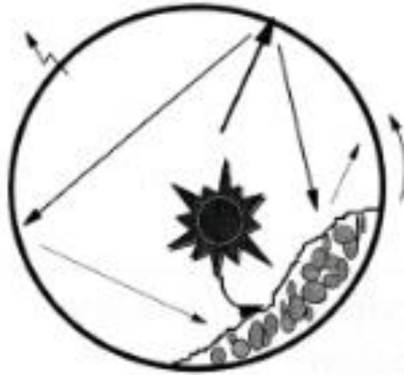
Figure 14 Heat flow paths in a rotary kiln. Radiation heat exchange in the cross section (Boateng, 2008).
