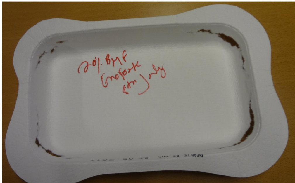
Picture 40. Ruptures in sample Conditioned Enoforte with 15% blank holding force.
