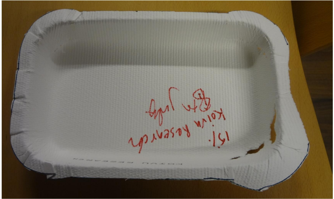
Picture 29. Ruptures in sample Conditioned Koivu Research pulp with 15% blank holding force.
