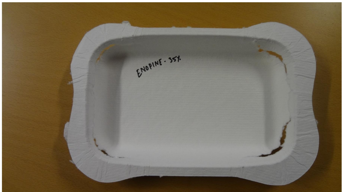
Picture 22 .Ruptures in sample Enopine with 35 % blank holding force.
