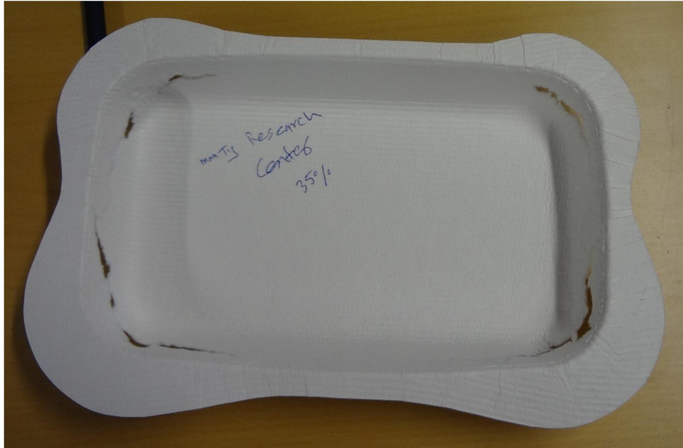
Picture 3. Rupture in sample Manty with 35 % blank holding force.
