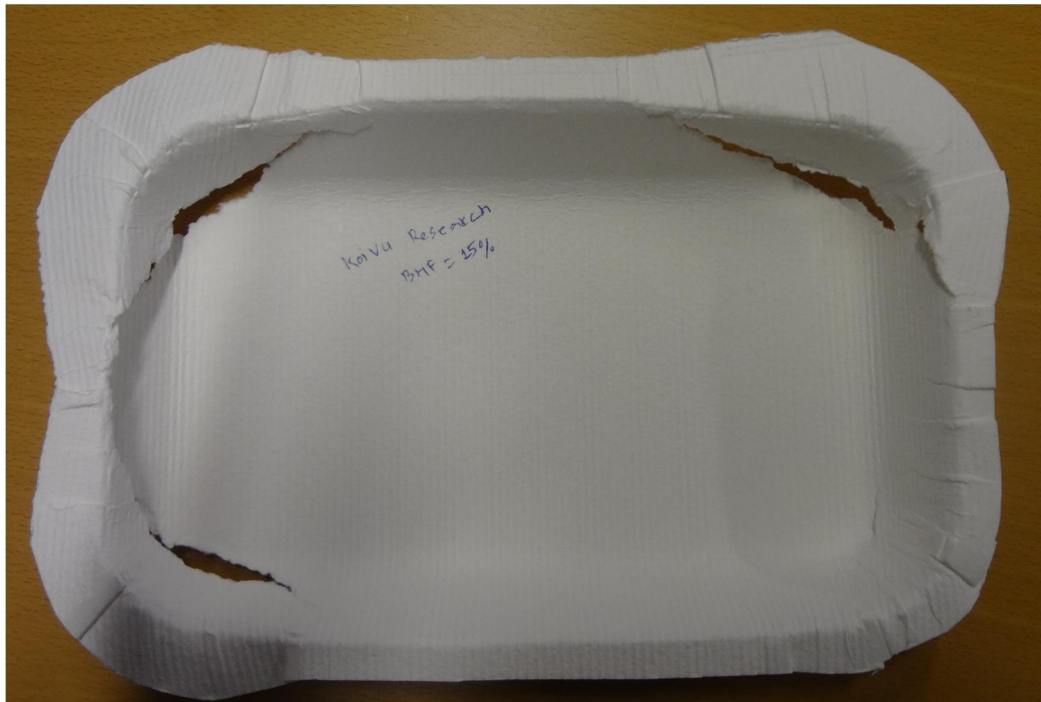
Picture 5. Ruptures in sample Koivu research with 15 % blank holding force.
