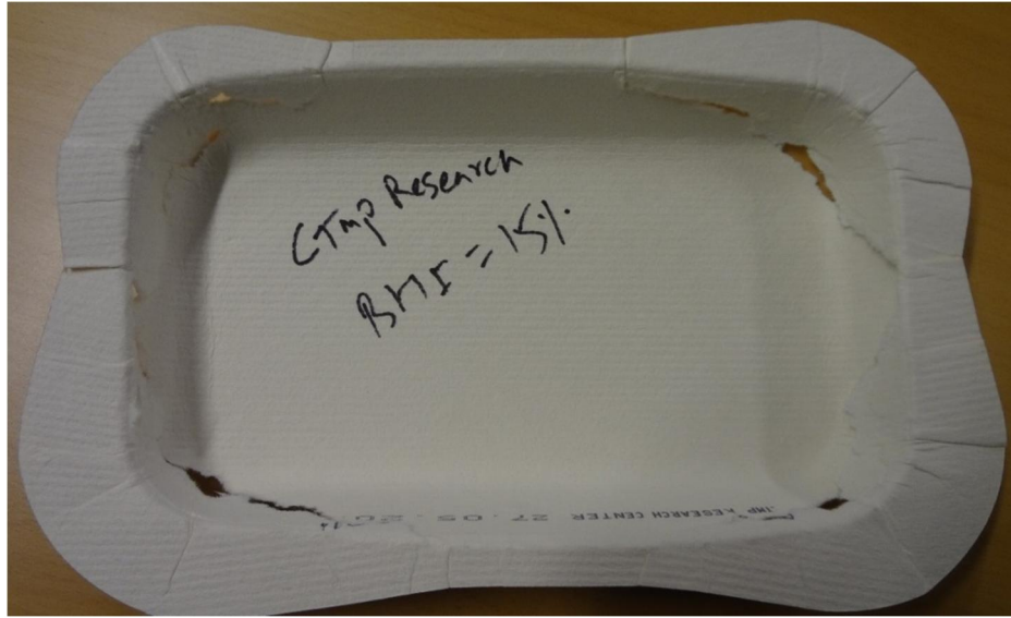
Picture 8. Ruptures in sample CTMP Research center with 15 % blank holding force.
