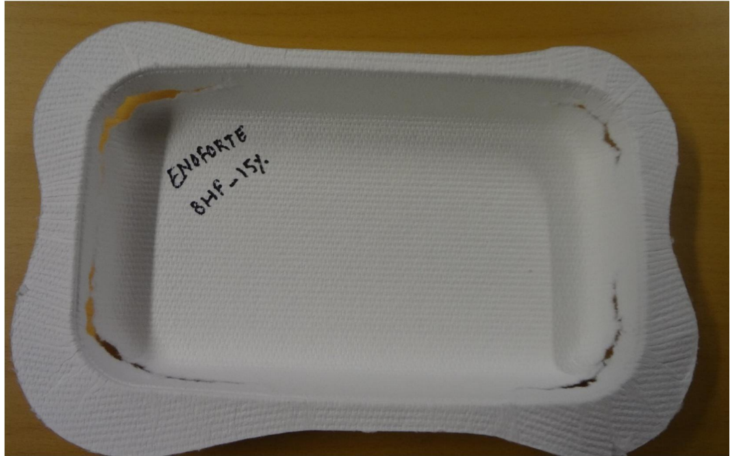
Picture 15 .Ruptures in sample Enoforte with 15 % blank holding force
