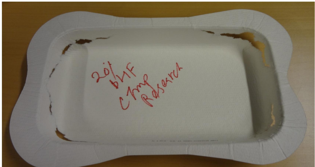
Picture 32. Ruptures in sample Conditioned CTMP Research with 20% blank holding force.
