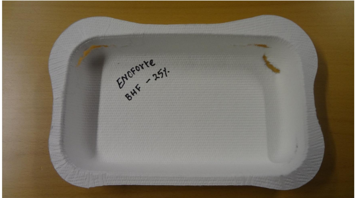
Picture 17. Ruptures in sample Enoforte pulp with 25 % blank holding force
