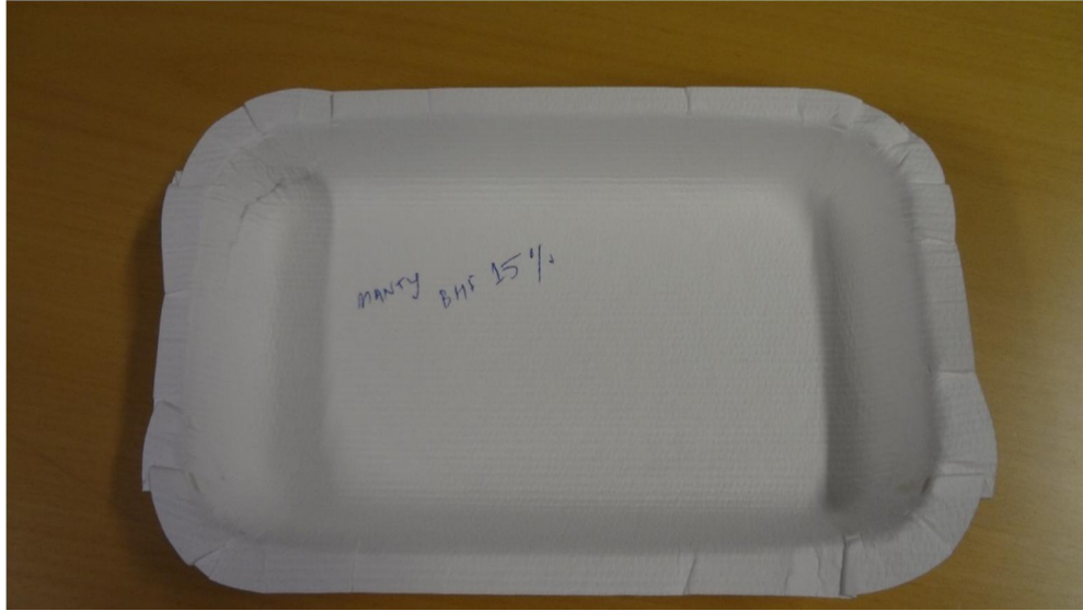
Picture 1. Ruptures in sample Manty with 15 % blank holding force.
