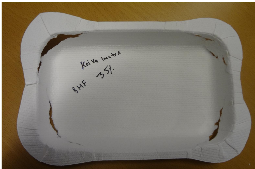
Picture 24. Ruptures in sample Koivu Imatra with 35 % blank holding force.
