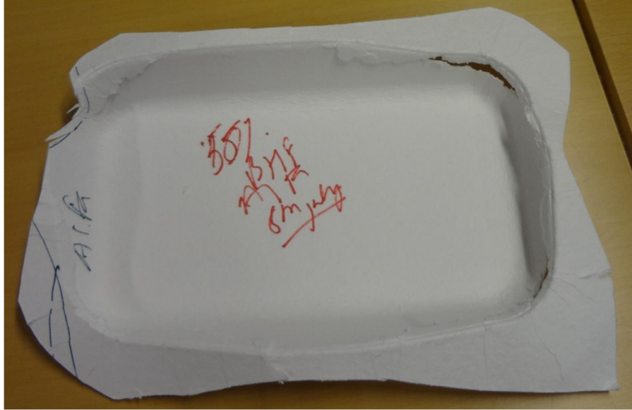
Picture 37. Ruptures in sample Conditioned Eno Alfa with 35% blank holding force.
