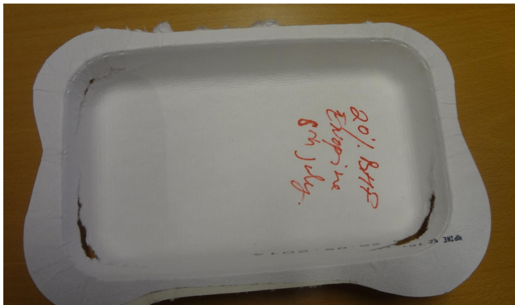
Picture 42. Ruptures in sample Conditioned Enopine with 20% blank holding force.
