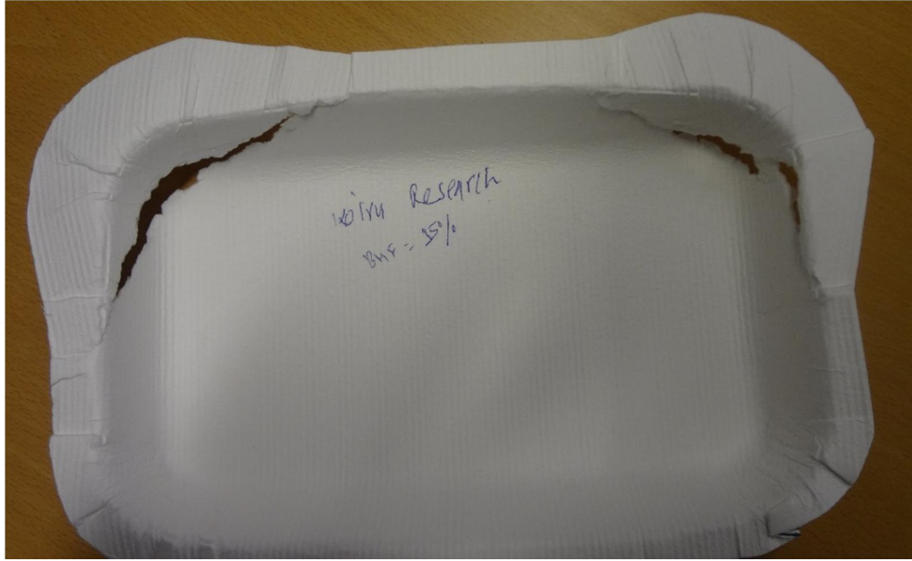
Picture 4. Ruptures in sample Koivu research with 15 % blank holding force.
