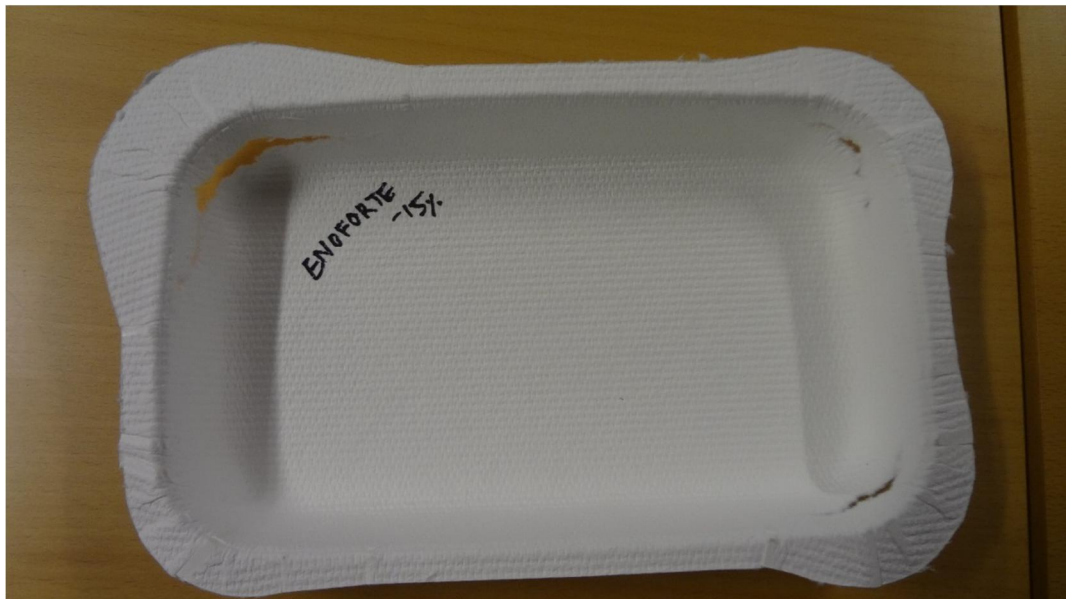
Picture 16. Ruptures in sample Enoforte with 15 % blank holding force
