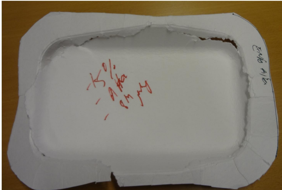
Picture 38. Ruptures in sample Conditioned Eno Alfa with 15% blank holding force.
