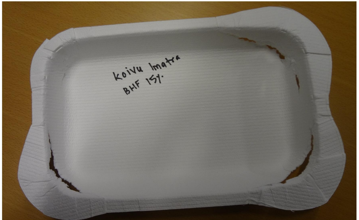
Picture 23. Ruptures in sample Koivu Imatra with 15 % blank holding force.
