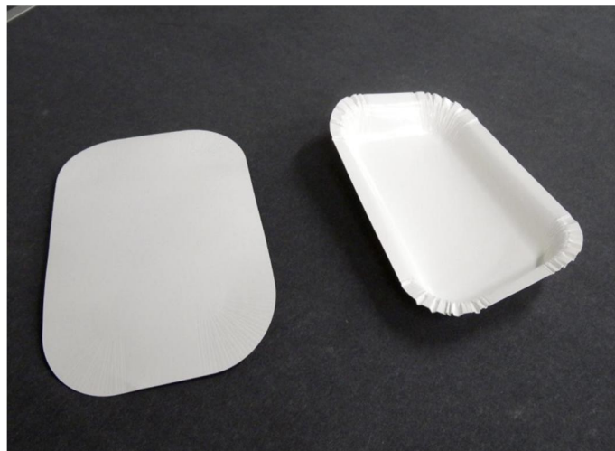
Figure 8. A blank sheet and a pressed tray in the forming module of LUT Adjustable Packaging Line.
