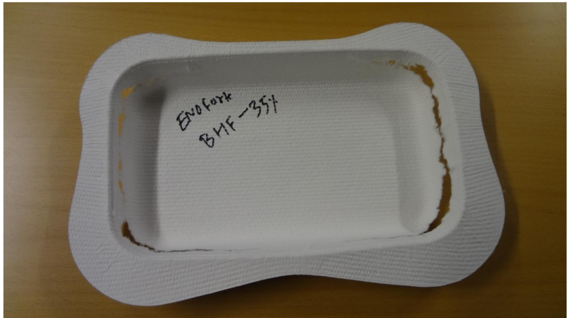
Picture 18. Ruptures in sample Enoforte with 35 % blank holding force
