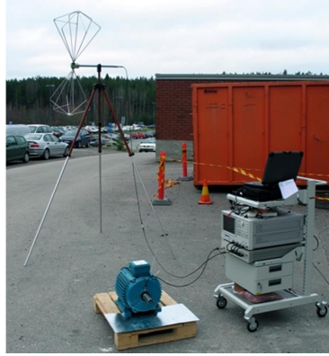
Fig. 4.3. Experimental measurement setup for link budget verification in the outdoor environment, where the transmitted signal is fed by an external signal source. In this measurement series, the motor was standing still and EDM was imitated by a 10 \Omega shunt resistor assembled over the insulation of the DE bearing.
