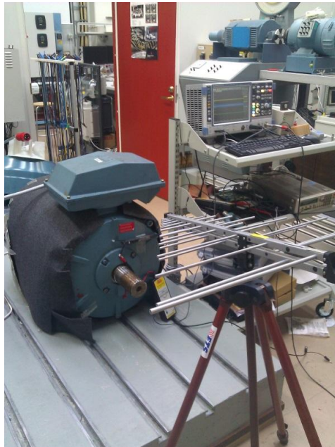
Fig. B2. P_n = 75 kW motor laboratory setup, where the motor is assembled on a motor test platform. It is pointed out that unlike the setup for the P_n = 15 kW motor, the P_n = 75 kW motor is also grounded through the platform.
