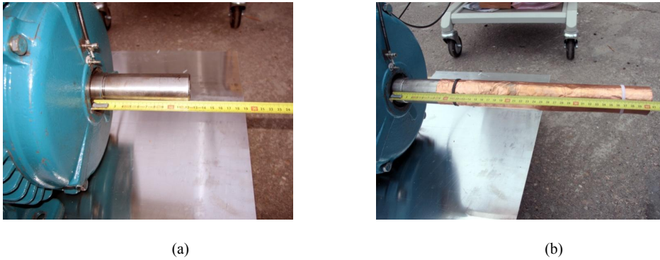
Fig. C2. Feed point of the motor with a 10\ \Omega surge resistor placed parallel to the feed point connection screws. In Fig. C2a, the shaft length is 12 cm; in Fig. C2b, the extended shaft length is 41 cm.
