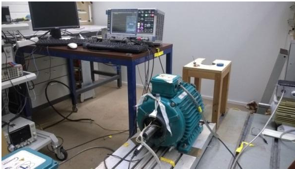
Fig. D2. Ni-HFMNFP assembled on the DE plate in the laboratory measurement setup.
