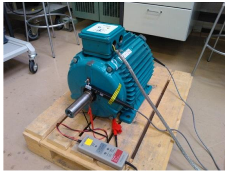
Fig. B1. P_n = 15 kW motor laboratory measurement setup placed on a wooden platform. The antenna is outside the photograph.
