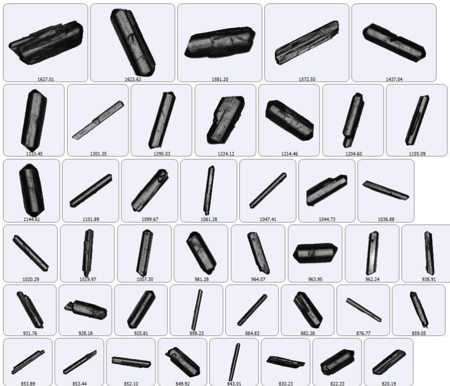
Figure 13. Particle images (x2.5) for crystallized product at 145 Hz and 20 °C/h.
