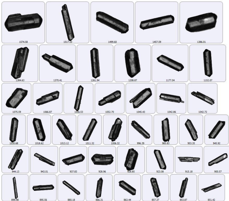
Figure 11. Particle images (x2.5) for crystallized product at 145 Hz and 5 °C/h.
