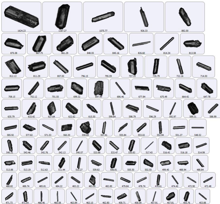
Figure 3. Particle images (x2.5) crystallized product without PEF at 10 °C/h.
