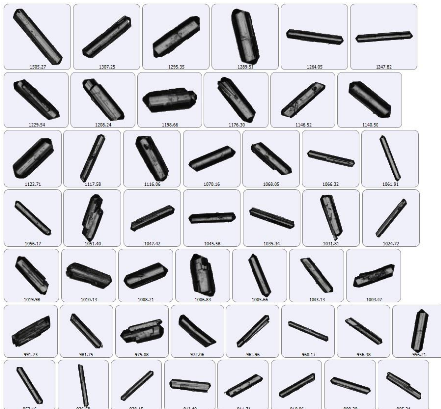
Figure 10. Particle images (x2.5) for crystallized product at 950 Hz and 20 °C/h.
