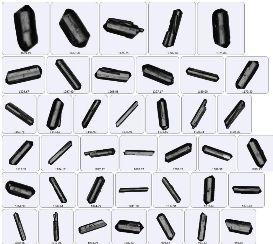
Figure 9. Particle images (x2.5) for crystallized product at 950 Hz and 10 °C/h.
