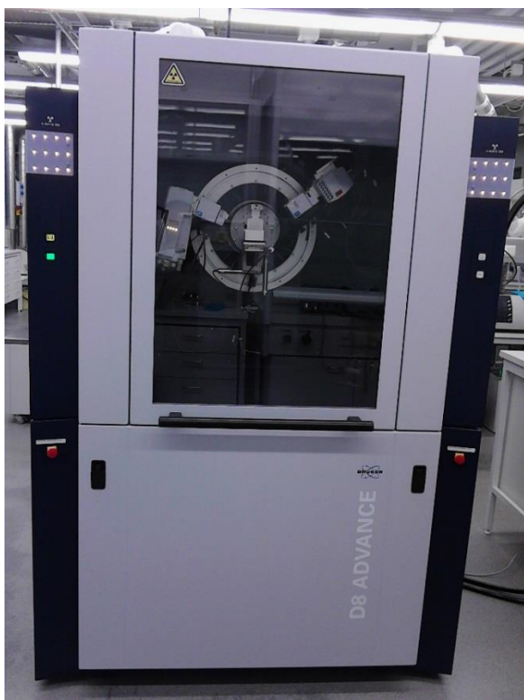
Figure 16. An image of Bruker D8 Advance X-ray diffractometer.
