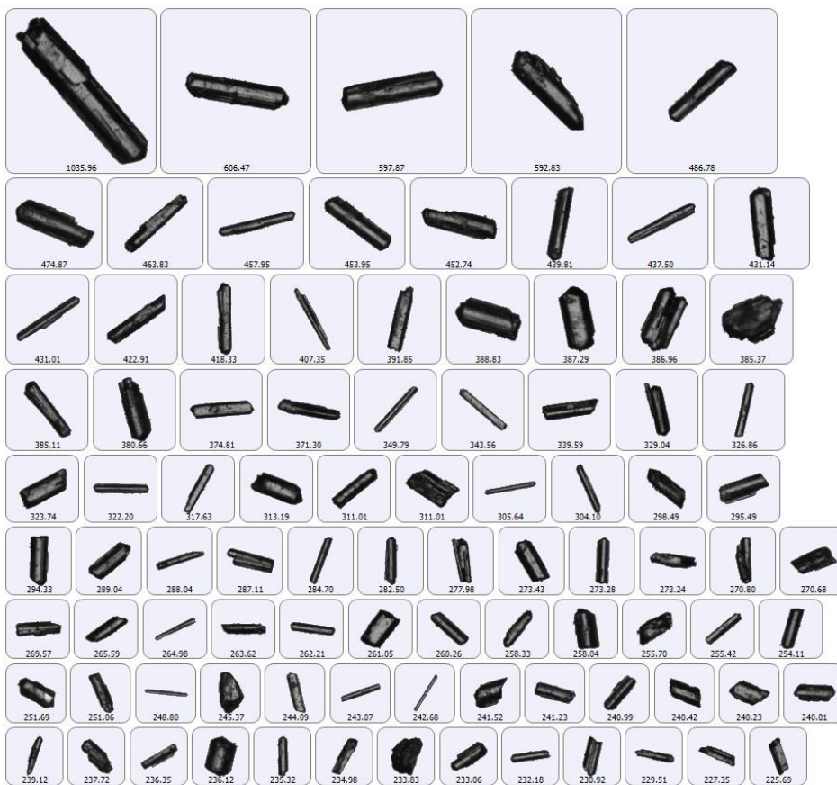
Figure 2. Particle images (x2.5) for crystallized product without PEF at 5 °C/h.
