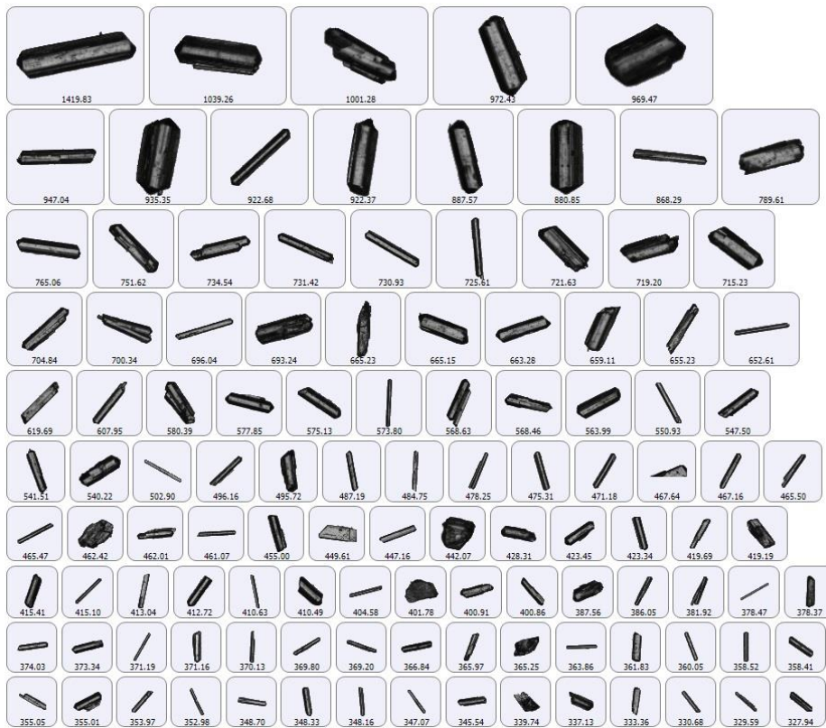
Figure 5. Particle images (x2.5) for crystallized product at 294 Hz and 5 °C/h.
