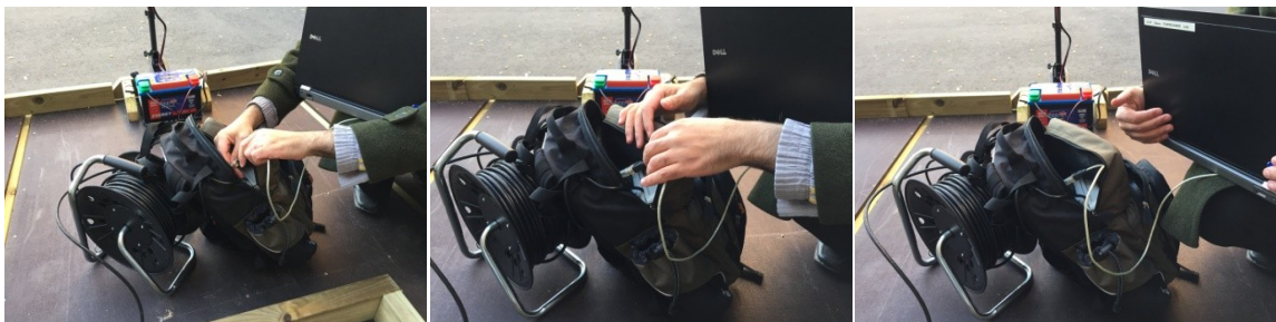
Figure 30 Connecting the PaquaBag to the laptop to set the time
