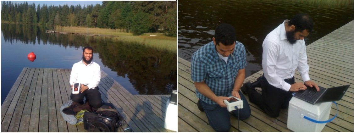
Figure 34 Manual readings using a similar probe but connected to the calibrating device
