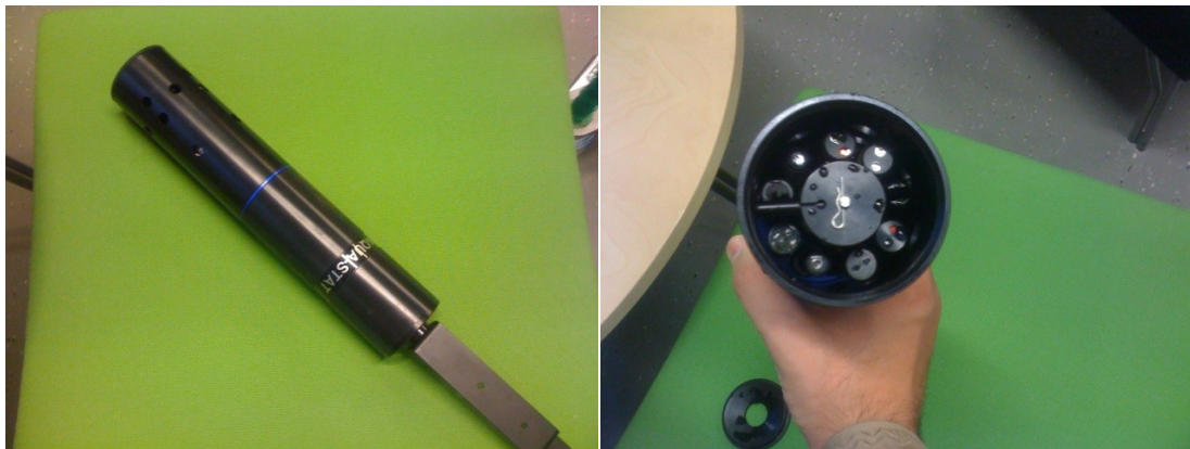
Figure 9 The probe and the multiple sensors inside
