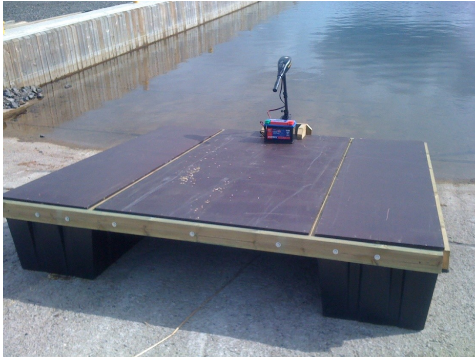
Figure 29 The ferry with the motor for the driving test
