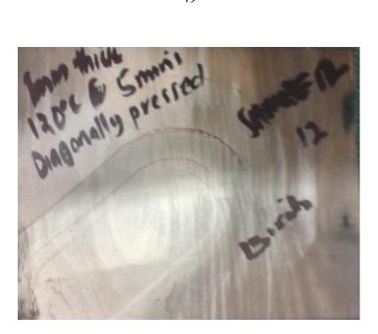
**Figure 30.** Birch forming test 3 of Sample 12 (Diagonally pressed)
