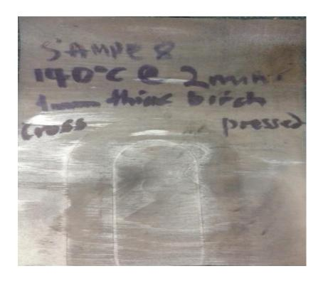
Sample of birch wood pressed under the temperature  $140^{\circ}\text{C}$
