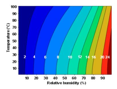
**Figure 13**. Equilibrium moisture content of wood (labeled contours) as a function of relative humidity and temperature (Glass & Zelinka, 2007, pp. 2-3).
