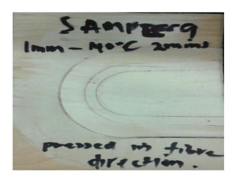
$\label{eq:APPENDIX II, 3/6}$  Sample of birch wood pressed and hold for 5 minutes under the packaging line machine
