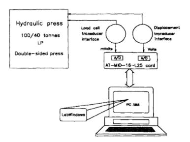
**Figure 17.** The interface between the hydraulic press and the PC (Browne and Battikha, 1995, pp. 218-223.).
