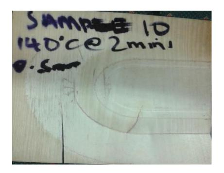
$\label{eq:APPENDIX II, 6/6}$  Sample of birch wood pressed under the temperature 140°C in diagonal orientation
