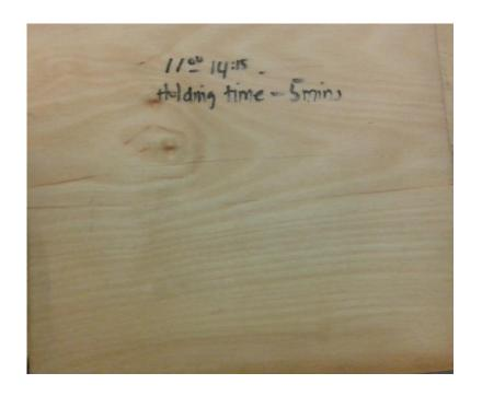
Sample of birch wood pressed in opposite direction of fiber grain.
