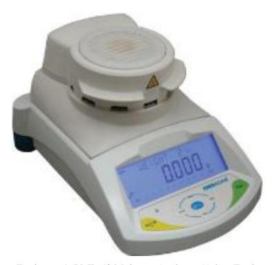
Figure 18. Adam Equipment's PMB 53 Moisture Analyzer (Adam Equipment, 2015).
