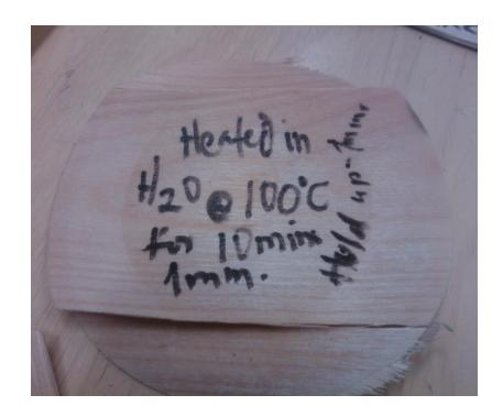
Samples of Birch veneer turned submerged in water.
