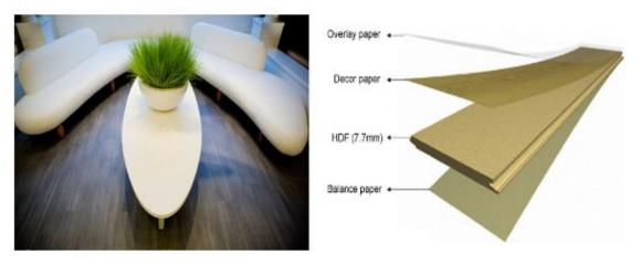
Figure 7. Structure of Commercial Flooring laminates (An, Kim & Kim, 2011, pp. 44-51).
