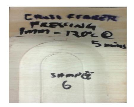
Sample of birch wood showing wetted surfaces after pressing under intense heat of 130 and  $10^{\circ}\text{C}$  respectively.
