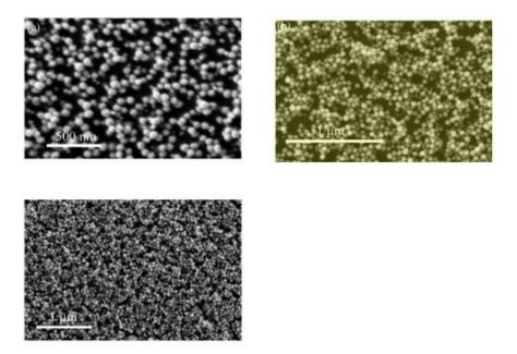
**Figure 11.** Images of thin solid film of various cycles. a) 2-cycle b) 4-cycle c) 20-cycle (Jia et al., 2014).
