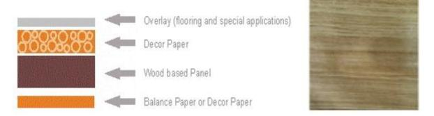
**Figure 10.** Thermally fuse impregnated papers (Kandelbauer et al., 2009, pp. 556-565).
