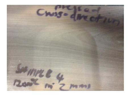
Picture 8. Sample of birch wood pressed in the same direction of fiber grain
