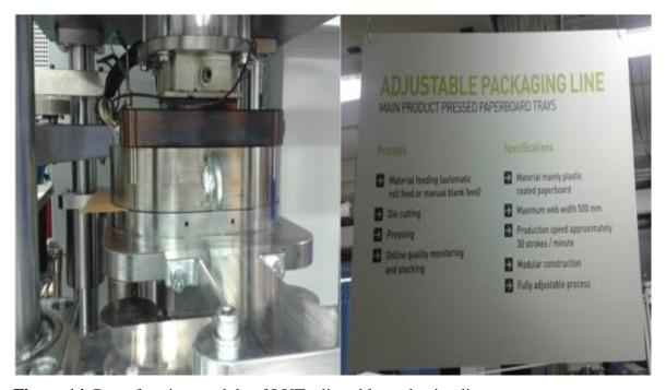
Figure 14. Press forming module of LUT adjustable packaging line
