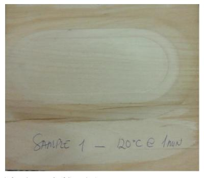
Figure 29. Birch forming test 3 of Sample 1.
