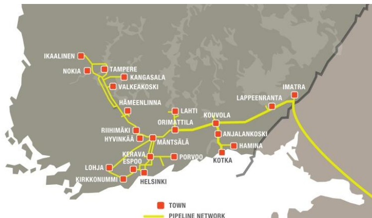
Figure 5.13: Current natural gas pipeline network (Source: Gasum)
