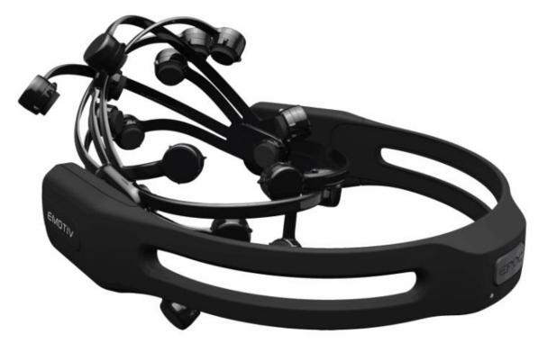
Figure 14.Tthe EPOC headset
