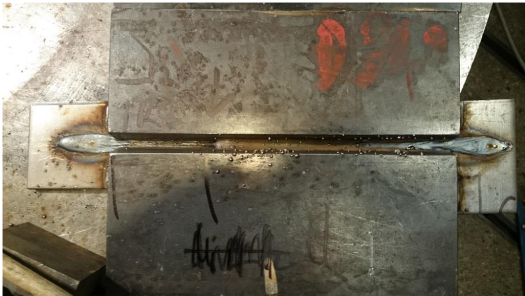
Figure 38. Increased spatter due to magnetic arc blow and arc disturbances. Spatter started to affect the welding in the middle section of the weld so that the welding pass had to be stopped.
