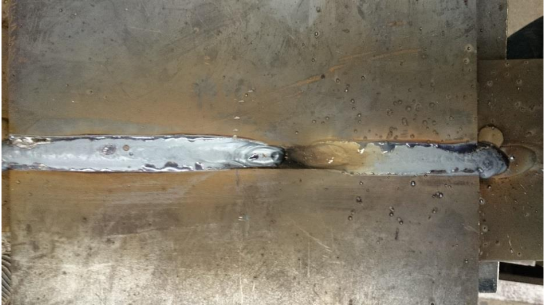
Figure 40. Test with metal cored filler wire OK Tubrod 14.02 and OK Aristorod 13.26 – welding direction from right to left leading with metal cored filler wire resulted in more spatters.
