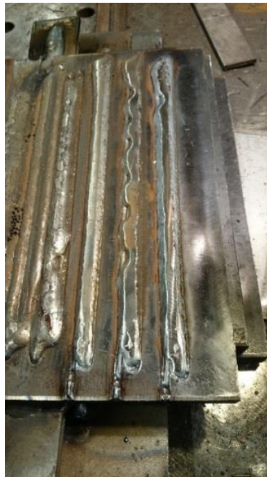
Figure 54. Test of usable angles of tandem MAG in surface welding.
