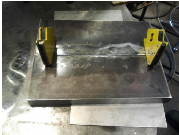
Figure 27. Preparation for welding and root gap measurement.
