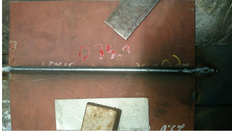
Figure 43 Test weld D35.1 – Root pass after welding.
