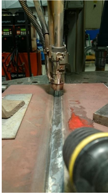
Figure 48. Angle of the welding head before welding the fifth bead - D35.5 with 20° angle between the wires and the welding direction.
