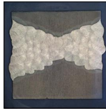
Figure 8. Tandem MAG horizontal position (PC). (Harris, 2014, p.7.)
