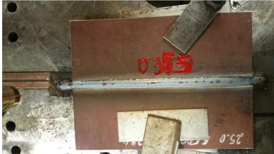
Figure 49. Test weld D35.5 – fifth bead after welding.
