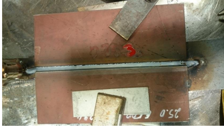
Figure 46. Test weld D35.3 – Third bead after welding.
