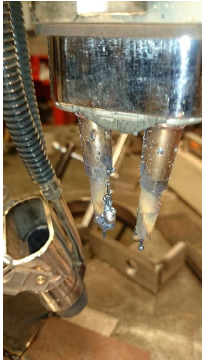
Figure 35. Spatter due to wrong torch placement in the welding gap
