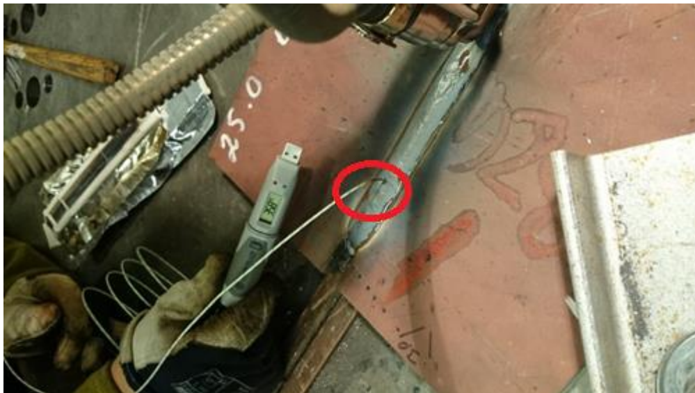
Figure 42. Weld cooling time measurements from 800 Celsius to 500 Celsius.
