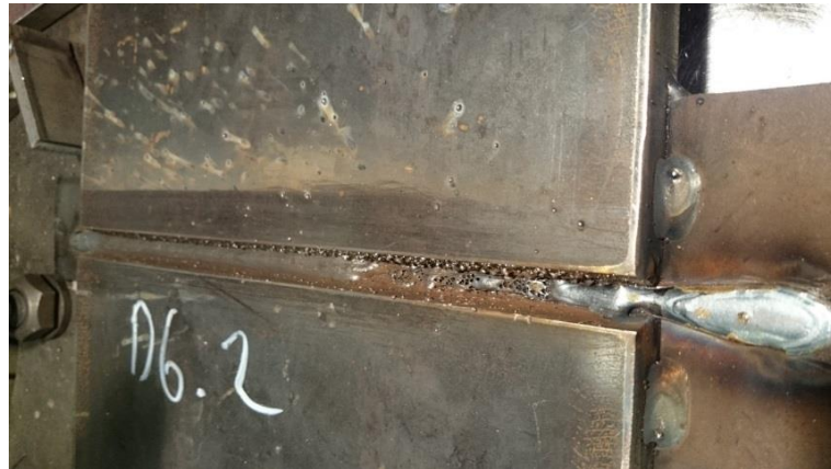
Figure 32. Spatter and welding gas problems with 15 L/min + 15 L/min gas flow rates.
