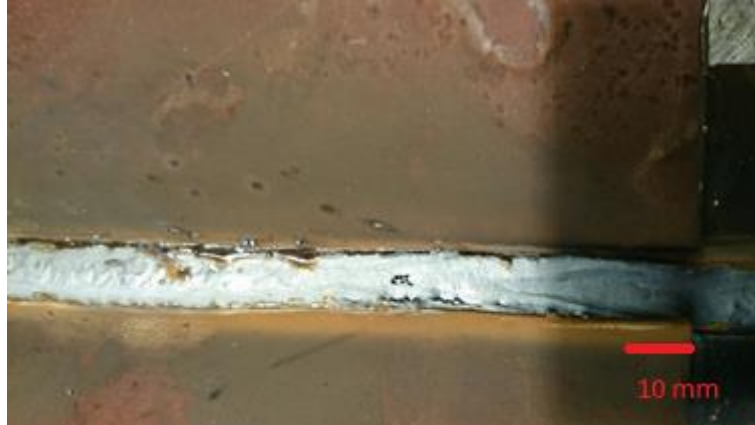
Figure 33. Gas pores near the end part of work piece due to gas problems and problems caused by magnetic arc blow while welding with 0.8 kJ/mm and gas flow rates of 20 L/min + 15 L/min.
