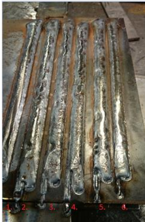
Figure 53. Gas flow rate test with parameters of 2.5 kJ/mm heat input.
