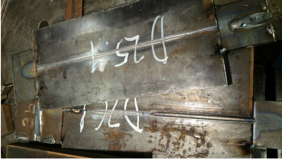
Figure 37. Example of root bead problems where the first part of the weld showed excessive penetration on the right, middle section had stabilized and visually good root while the end part had too little penetration on the left.
