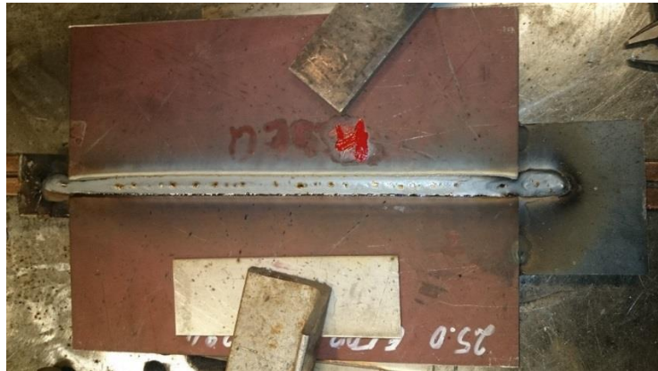
Figure 47. Test weld D35.4 – fourth bead after welding.
