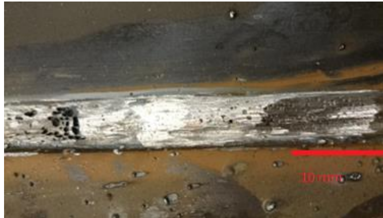
Figure 34. Close-up of gas pores beneath the weld surface after grinding while welding with 0.8 kJ/mm and gas flow rates of 20 L/min + 15 L/min.
