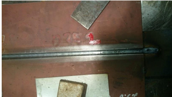
Figure 44. Test weld D35.2 – Second pass after welding.
