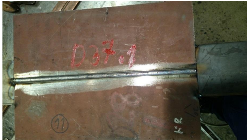
Figure 50. Example of succesful root pass quality
