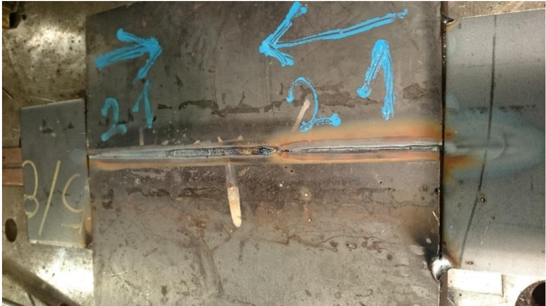
Figure 39. Test with metal cored filler wire OK Tubrod 14.02 and OK Aristorod 13.26 – root leading with OK Aristorod 13.26 showed deeper and wider penetration. Both of the wires had diameter of 1.2 mm.
