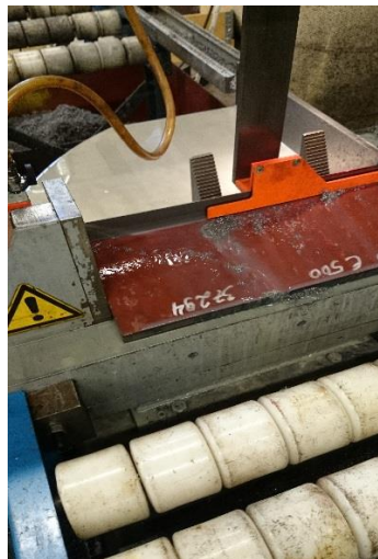
Figure 26. Sawing the joint to correct angle
