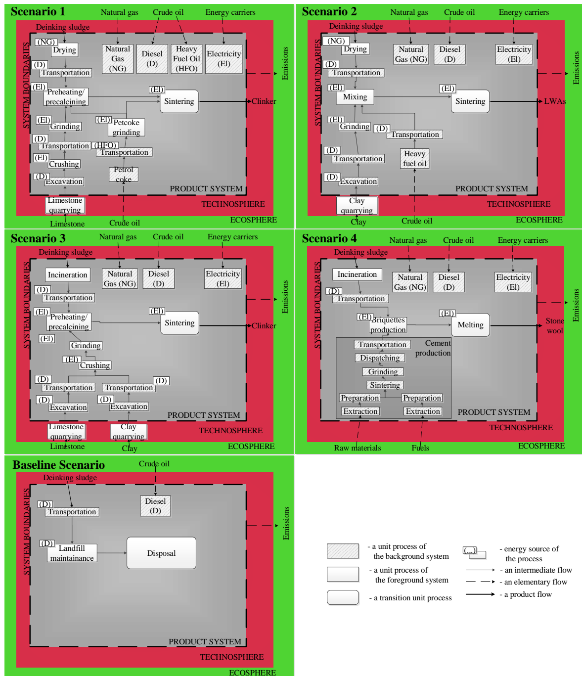
Figure 10. Detailed flow-chart of the unit processes included in each product system assessed in the study.
