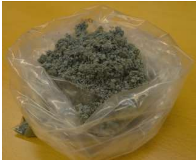
Figure 5: Appearance of deinking sludge generated at the case study paper mill.
