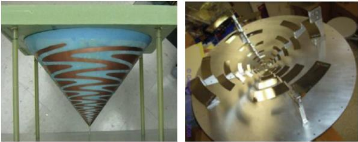
Fig. 1.3. Sinuous antenna (left) and self-complementary antenna (right).
