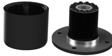
Fig. 2. Rotor and stator of the PMSM studied. The stator with semiclosed slots is skewed to avoid cogging. The stator winding is a double-layer tooth coil winding containing two coil sides in each slot.
