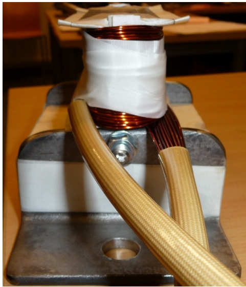
Figure 2.21: Photo of a tooth (stator segment) that contains the stator coil with parallel strands.
