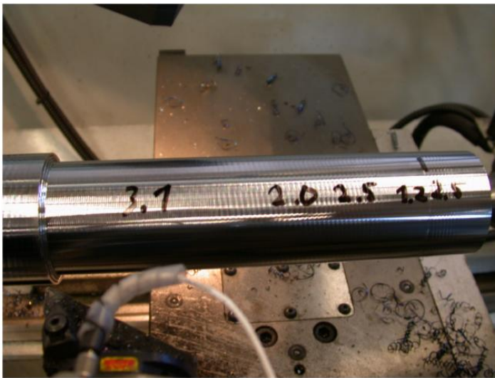
Figure 6.1: Visible chatter marks. Surface roughness values measured in micrometers ( R_a or arithmetic average).
