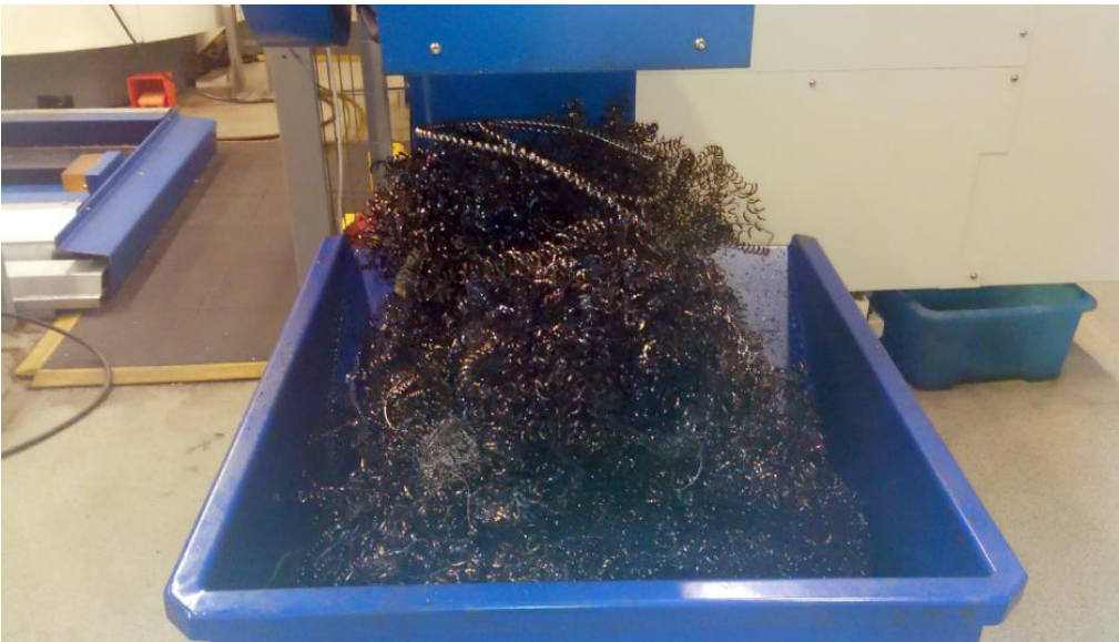
Fig. 7.1: Handling long chips is difficult, as the swarf may clog conveyor systems (such as the one seen on top of this figure).
