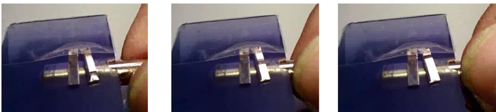
Figure 4.1. When 1) an MSM element is placed near 2) a diametrically magnetized cylindrical magnet, 3) a local twin configuration, named a shrinkage, is formed near the poles of the magnet (top). As the magnet is rotated, this shrinkage travels along the MSM element to follow the poles of the magnet (bottom, left to right). Pictures provided courtesy of the Magnetic Materials Laboratory, BSU.
