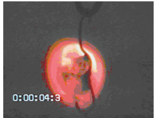
Figure 4-4, Example of black liquor droplet at the end of devolatilization, laboratory conditions (Åbo Akademi).
