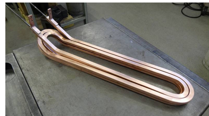
Fig. 2. Liquid-cooled tooth-coil shown without insulation.
