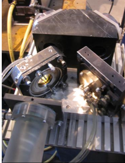
Figure 33. Beam splitter device that cuts of 50% of laser power.
