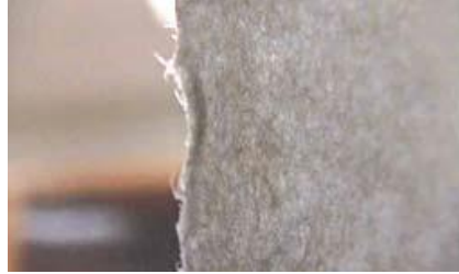
Figure 28. Water jet cut edge quality with turbulent flow (Kershaw, 2015).
