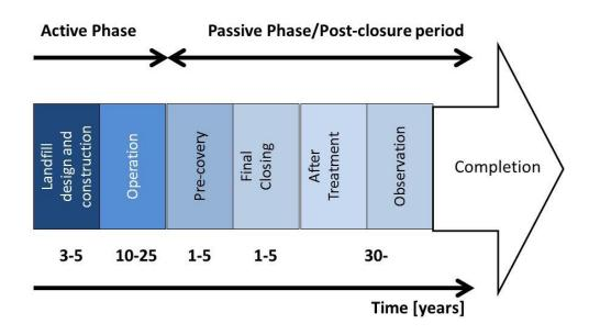
Fig. 3. Landfill management phases throughout the life-cycle; the time-frames are typical for Finland and could vary case by case (Modified after Laner *et al.*, 2012).
