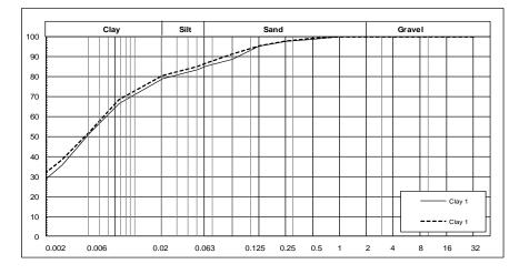
Fig. 13. Grain size distribution curves of Clay 1.
