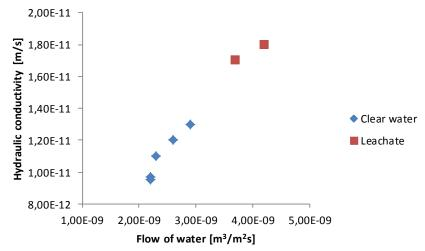
Fig. 19. Geosynthetic clay liner hydraulic conductivity results tested with clean water and leachate.
