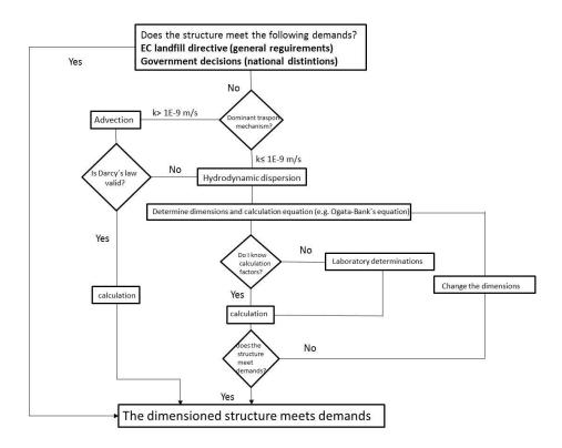
Fig. 24. Flowchart showing the landfill bottom structure risk analysis with the SRA method.
