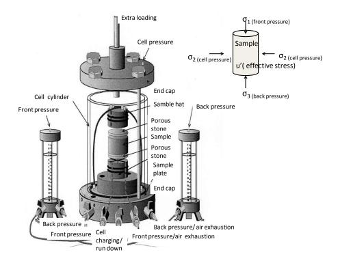
Fig. 15. The sample has been in a flexible wall permeameter under water pressure to squeeze rubber ring tightly against the sample, preventing potential edge flow (Modified after Virtanen, 2001).
