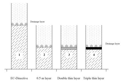
Fig. 11. Four different conceptual bottom layer structures and dimensions used in this study. 1) EC directive and 2) 0.5-meter layer has single homogenous material as a mineral layer, 3) double layer has very thin and low hydraulic conductivity layer and below higher hydraulic conductivity layer, 4) triple layer has two very thin and quite low hydraulic conductivity layers and below higher hydraulic conductivity layers (Environmental permit registry, 2010)
