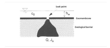
Fig. 8. Katsumi leakage model (Modified after Katsumi et al., 2001).
