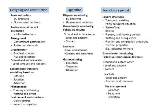
Fig. 4. MSW landfill environmental management divided into three management periods during the life-cycle (Modified after Laner *et al.,* 2012; Morris & Barlaz, 2011; Pivato, 2004; Christensen *et al.,* 2000).
