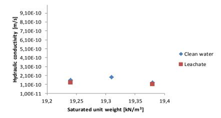
Fig. 21. Hydraulic conductivity of natural clay materials tested with clean water and leachate.
