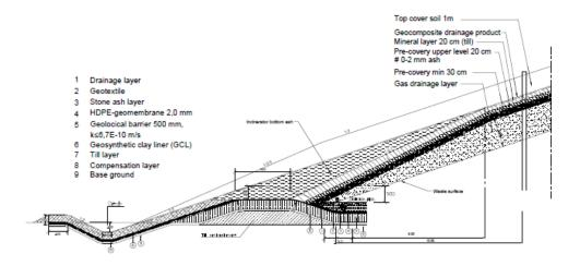
Fig. 25. The structural dimensioning of the surface structure.
