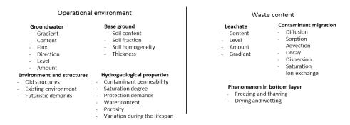
Fig. 5. Identifiable effects related to the landfill operational environment and waste content based on theory (Modified after Laner *et al.*, 2012; Morris & Barlaz, 2011; Pivato, 2004; Christensen *et al.*, 2000).
