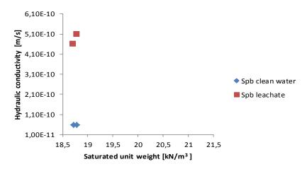
Fig. 20. Sand mixed with polymer bentonite hydraulic conductivity (m/s) results testing with clean water and leachate.
