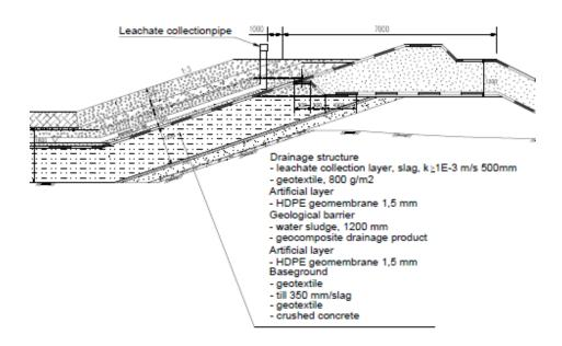
Fig. 27. The structural dimensioning of the innovative bottom structure.
