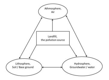
Fig. 16. Main areas where landfills could cause problems and pollute the environment. (Modified after Butt *et al.*, 2014 and Moriarty *et al.*, 1993).
