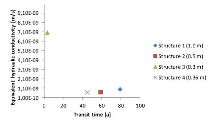
Fig. 18. Transit times of four different structures have been calculated based on the equivalent calculation caused by advection. Hydraulic conductivity values were the examined hydraulic conductivity values in this study.
