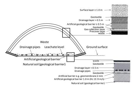
Fig. 1. Conceptual presentation of the landfill structure (VNp 861, 1997).
