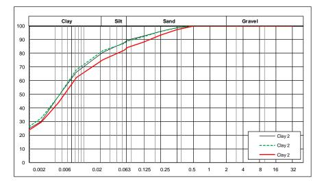
Fig. 14. Grain size distribution curves of Clay 2.
