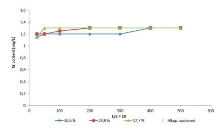
Fig. 28. The chromium solubility test results with the leachate (alkup. suotovesi means leachate in English).
