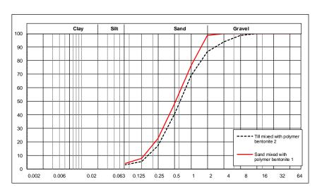
Fig. 12. Grain size distribution curves of sand and till mixed with polymer bentonite material.
